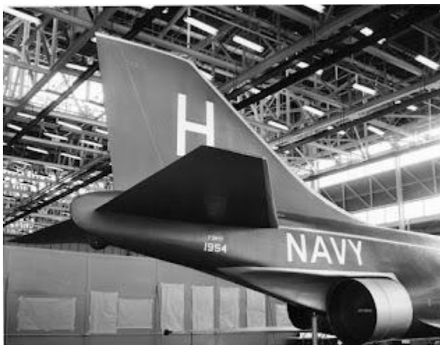
Tail section of the F3H-G mockup showing the two different engine sizes- The J79 was on the right side, the J65 was on the left side.
