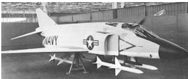
F4H full scale mock up showing the originally planned trapeze launchers for the Sparrow missiles.
