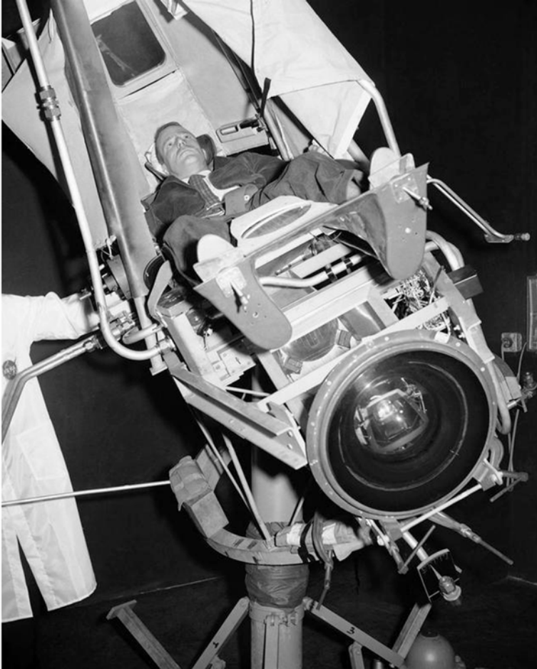
Carpenter demonstrates the use of the ALFA trainer. It furnished practice in using the manual controls that keep the Mercury capsule in proper alignment during flight. The mirror in the lower foreground is part of the optical system which gave the astronaut a visual check on the relationship of the capsule and the Earth during simulated flight. (Photo: NASA)
