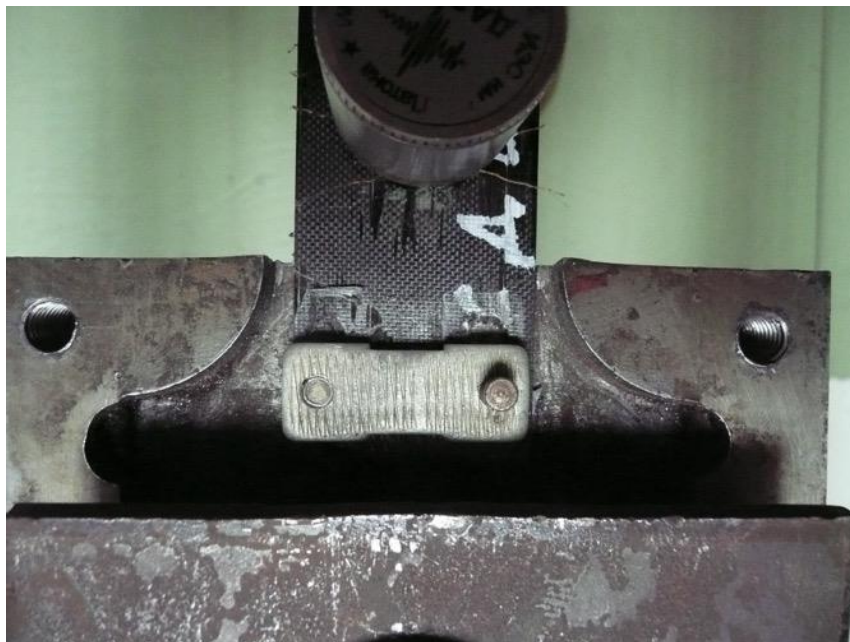
Figure 72. The area of carbon fibre specimen destruction. Coordinate of destruction is near 284 mm (sensor No 2)
