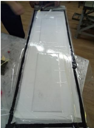
Figure 76. Panel with sensors, under a vacuum film, prepared for molding
