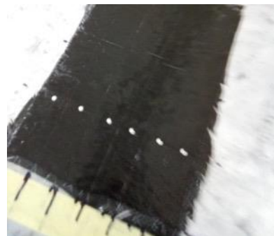
Figure 77. Installation of sensors with the help of grid on samples for shear and bending tests
