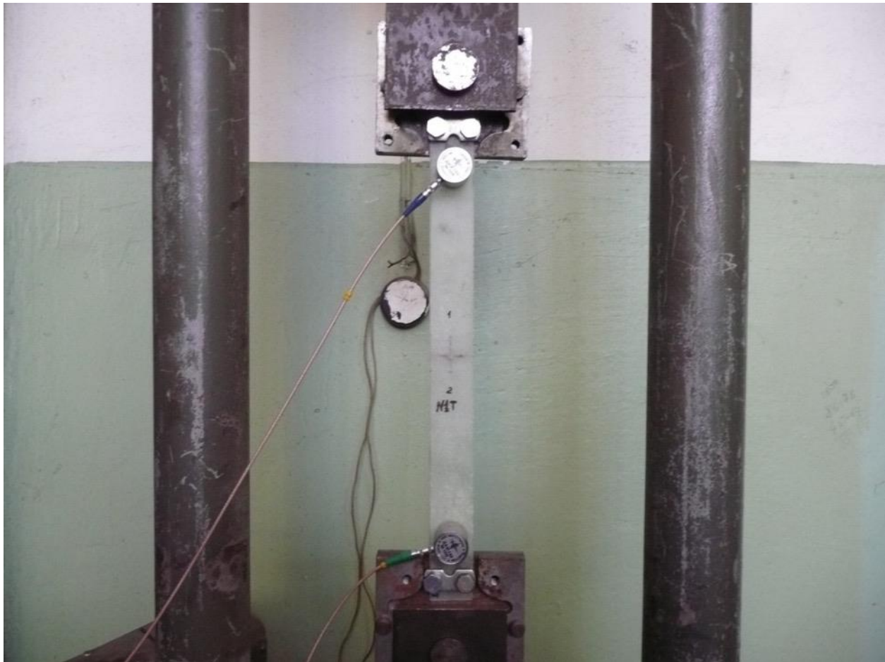
Figure 66. The test machine hold part with fiberglass specimen having embedded simulator of piezo sensor
