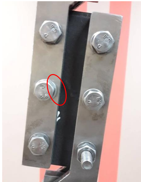
Figure 94. Delamination at the sensor zone
