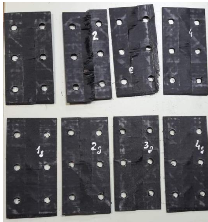
Figure 84. Samples after shear tests: top – without sensors, bottom – with sensors
