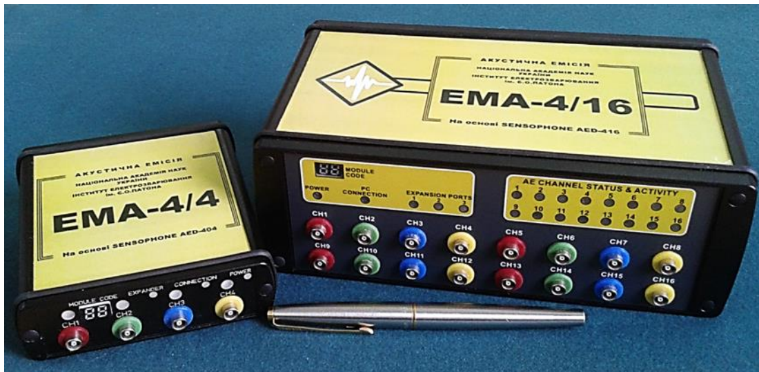
Figure 9. New generation instruments EMA-4 based on 4-channel and 16-channel modules AED-404, AED-416
