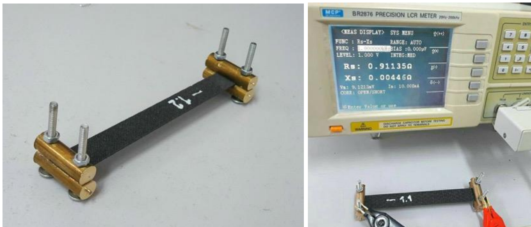
Figure 6. Electrical resistivity measurement
