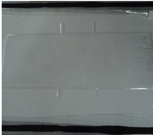
Figure 76. Panel with sensors, under a vacuum film, prepared for molding
