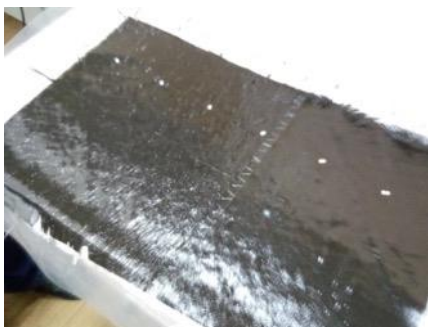
Figure 77. Installation of sensors with the help of grid on samples for shear and bending tests
