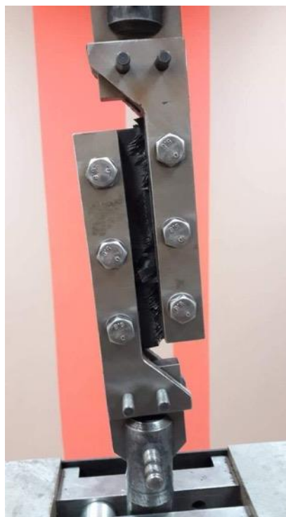
Figure 85. Tests under shear samples without a sensor
