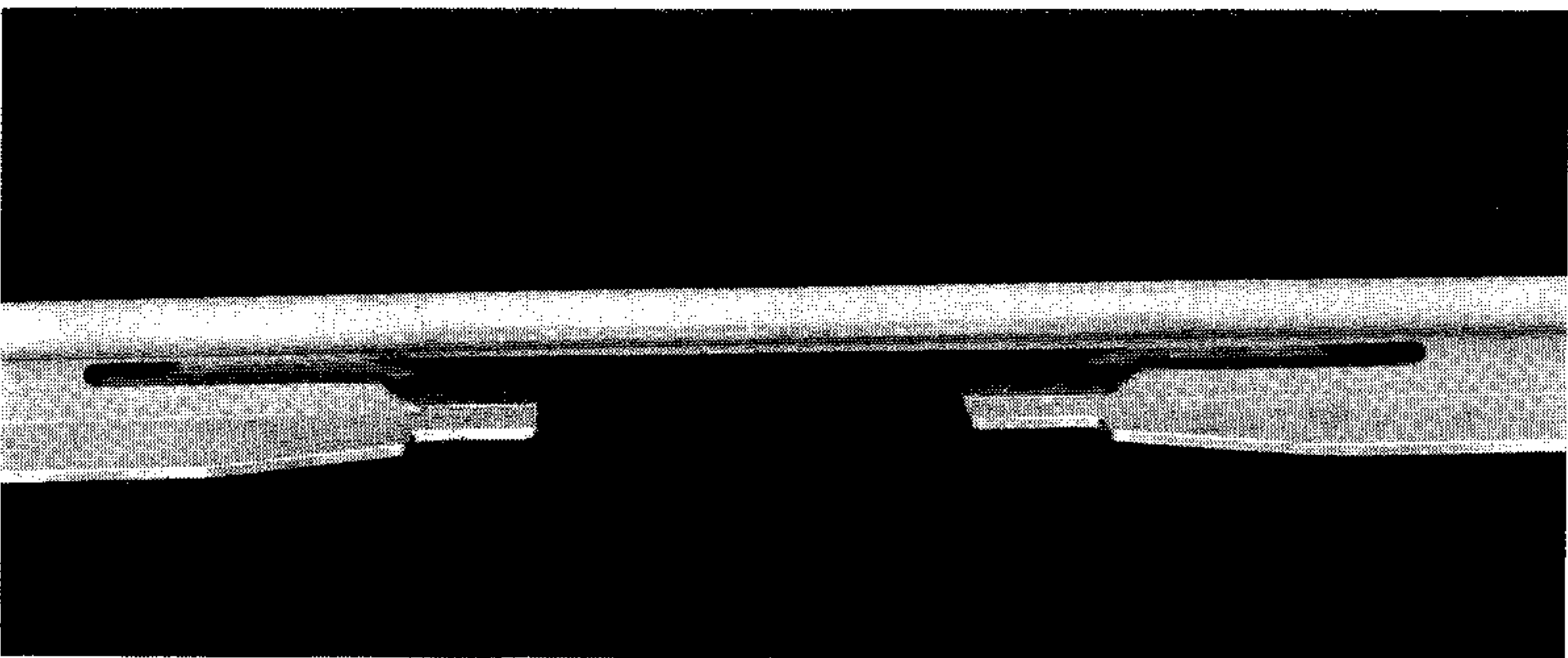
ADAPTER STRINGERS are delivered to McDonnell as 60-ft. long magnesium alloy extrusions (top left) then machined at intervals to leave only the tubing (bottom left). Gemini adapter module (right) is both equipment storage unit and radiator.
