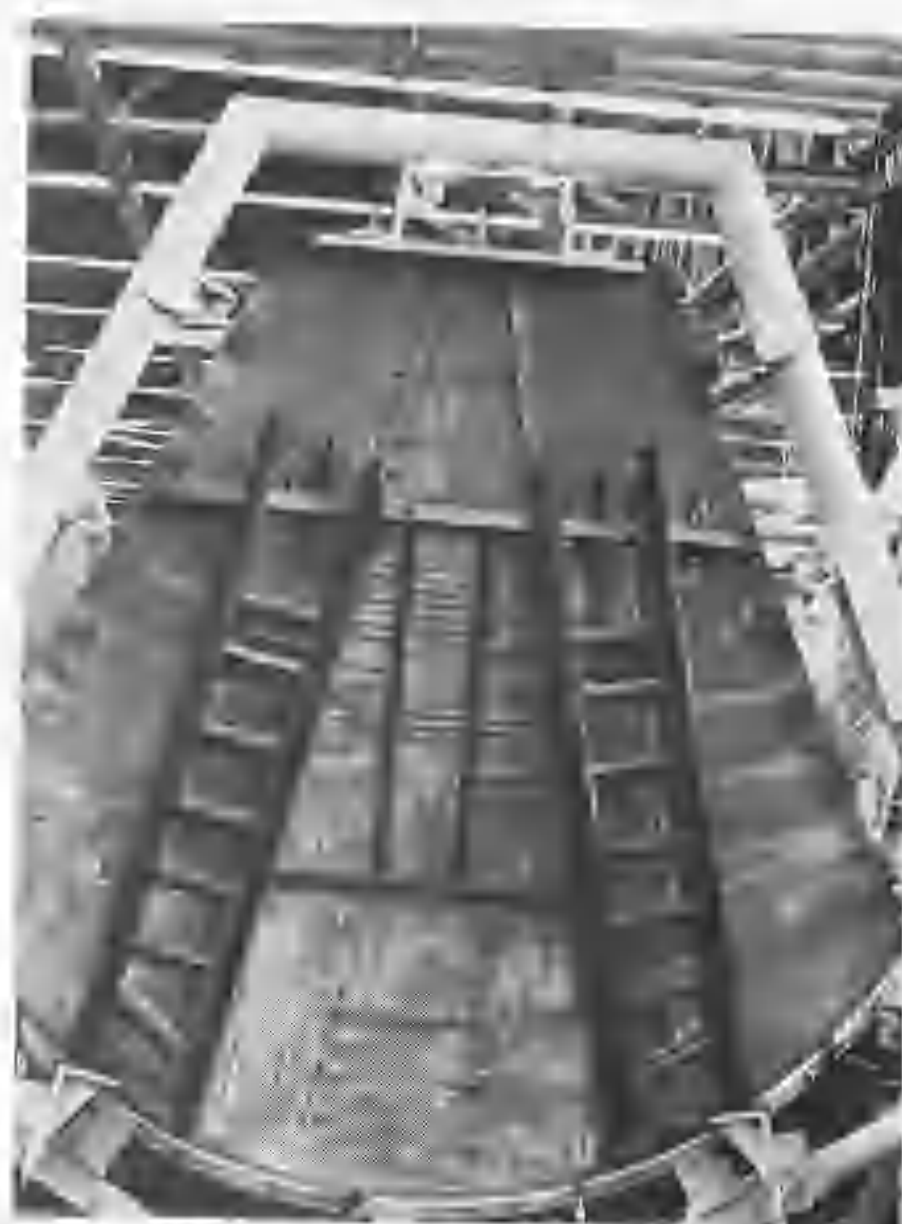
PRESSURE BULKHEAD which forms rear wall of the Gemini cockpit shows mountings for the aluminum rails on which ejection seats rest. Rubber guards are for plant use.
