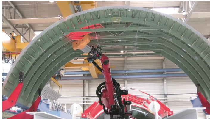
Figure 11. Fuselage section assembly inspection system
