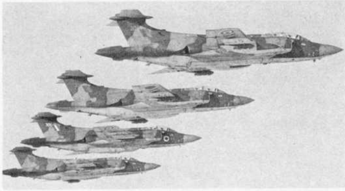
Hawker Siddeley Buccaneers, in the Martel-equipped S Mk 2B version, equip one strike bomber Wing in RAF Germany and provide the heaviest offensive support of any German-based types. Aircraft of No 15 Squadron are illustrated.
