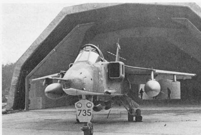
The BAC Lightning F Mk 2A (left, No 19 Squadron) will leave service with RAF Germany at the end of 1976, but the F Mk 6 will continue for several more years with No 11 Group for home defence in the UK. Hardened shelters, or "hangarettes", are being provided at all RAF bases in Germany, for aircraft on quick-reaction alert, as illustrated here at RAF Brüggen with a visiting Jaguar from No 6 Squadron.
