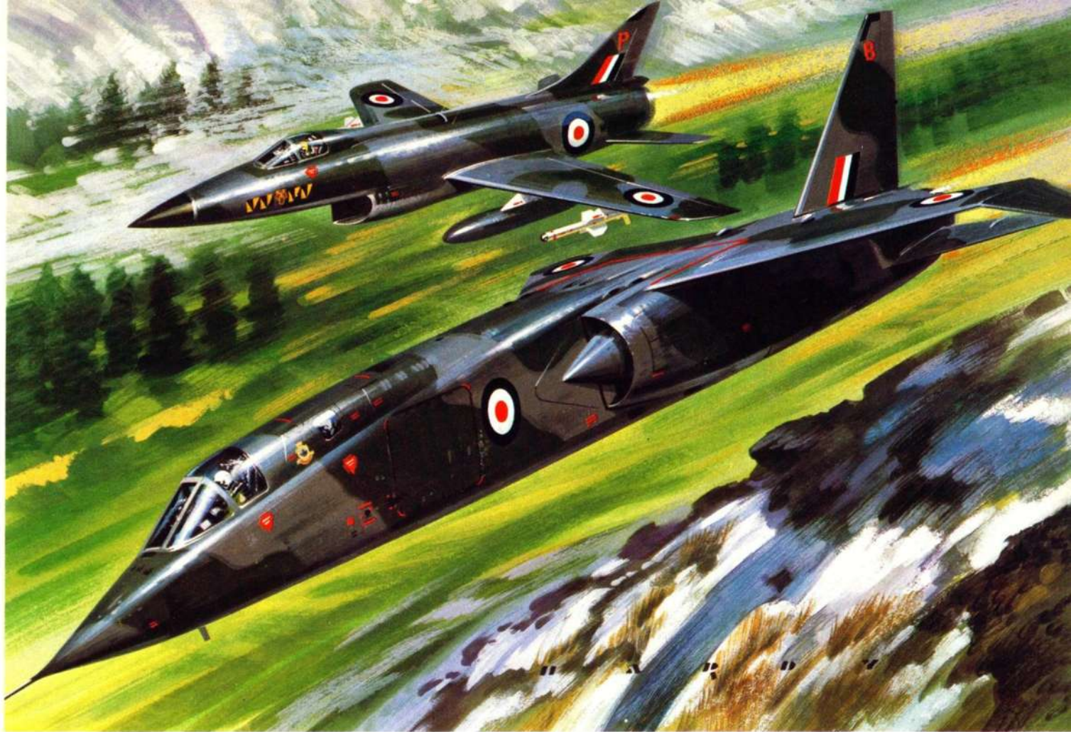
Two of the new RAF types which progressed some way towards service introduction before being cancelled are shown here in formation—in the foreground the BAC TSR 2 strike/reconnaissance bomber and behind it the Hawker P.1121 all-weather ground attack fighter.
