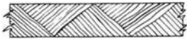
NUMBER FIVE KWILKO ½ INCH STITCHED, COVERED BOTH SIDES WITH FLAME-PROOF GAUZE.
