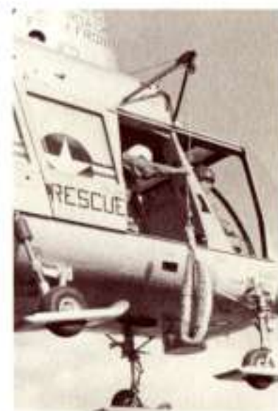
Personnel hoist mounted directly above rescue door.
