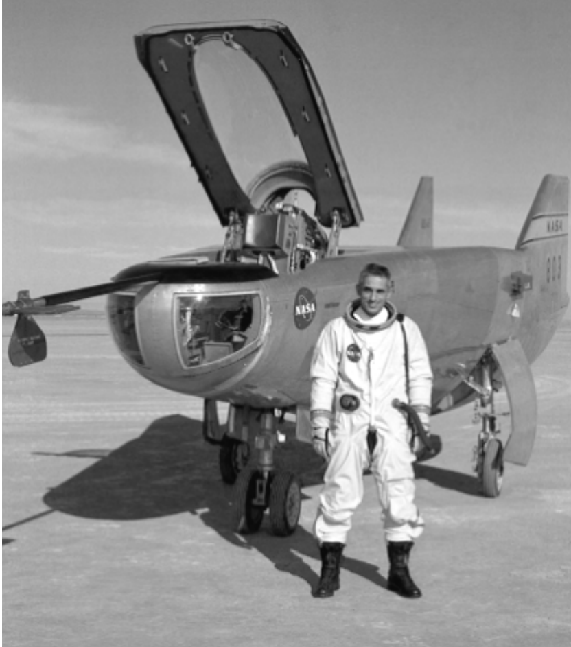
NASA research pilot John A. Manke, pictured here in front of the M2-F3 lifting body, a reincarnation of the crashed M2-F2. Paul Bickle decided to rebuild it as a backup lifting body and headquarters paid for the reconstruction, adding a stability augmentation system, a middle vertical fin, and some subtle modifications affecting the aerodynamics. It proved to be far more mannerly in flight than the M2-F1 or M2-F2. (NASA Photo Number ECN-3448.)
