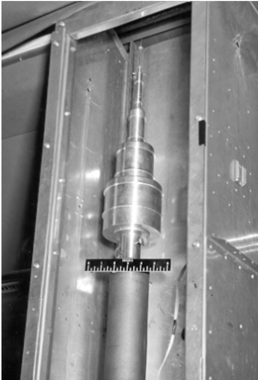
A close-up of Langmuir's ingenious, "wedding cake" shaped instrument used to measure the size and water content of ice droplets suspended in clouds. (Photo courtesy of the Dryden Flight Research Center Historical Reference Collection.)
