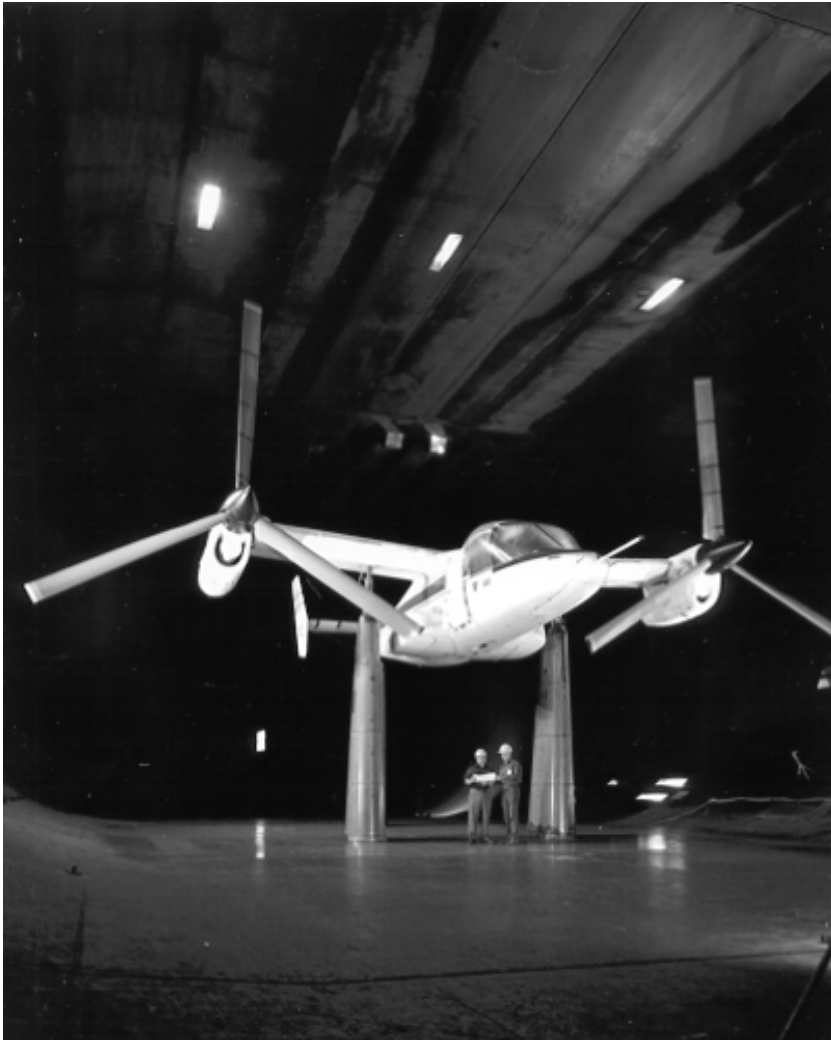
The XV-15 Tilt-Rotor aircraft number two, mounted in the Ames Research Center's forty-by-eighty-foot wind tunnel, underwent intensive aerodynamic research. Conducted in May and June 1978, these tests gauged the vehicle's airworthiness prior to the start of contractor flights the following year. (NASA Photo Number AC78-0579-1.)
