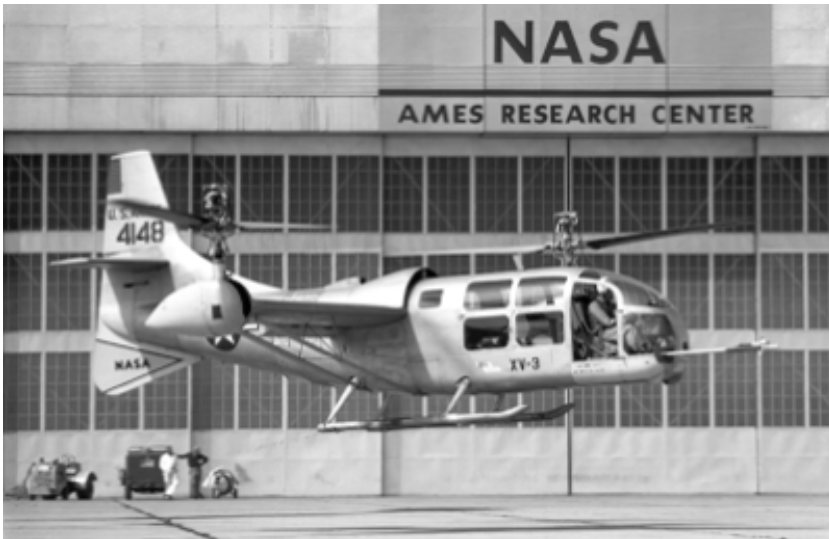
Precursor of the XV-15 Tilt-Rotor aircraft, the XV-3 is seen hovering in a 1961 photograph against the background of the Ames Research Center hangar. Designed by engineer Robert Lichten of Bell Aircraft, it lacked sufficient power and exhibited dangerous vertical cockpit vibrations. Nonetheless, the data amassed from the XV-3 demonstration flights proved invaluable to the later XV-15 project. (NASA Photo Number A-27737.)
