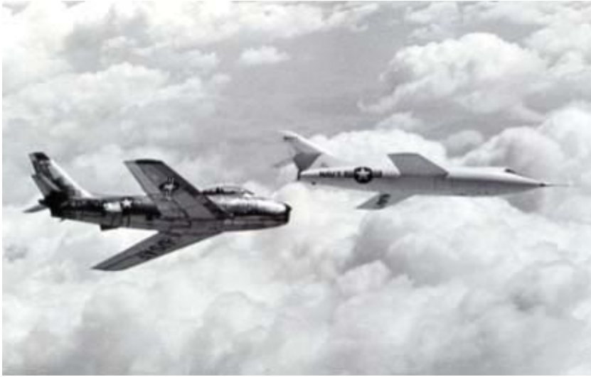
Phase II of the D-558 program centered on the D-558 Skyrocket (shown in flight with a North American F-86 Sabre flying chase). It featured a varied array of propulsion systems: turbojets, air-launched rockets, and combinations of the two. Unlike its predecessor, the Skyrocket was equipped with swept wings—an innovation arrived at independently by NACA aerodynamicist R.T. Jones—and also flew supersonically. (NASA Photo Number E-3996.)
