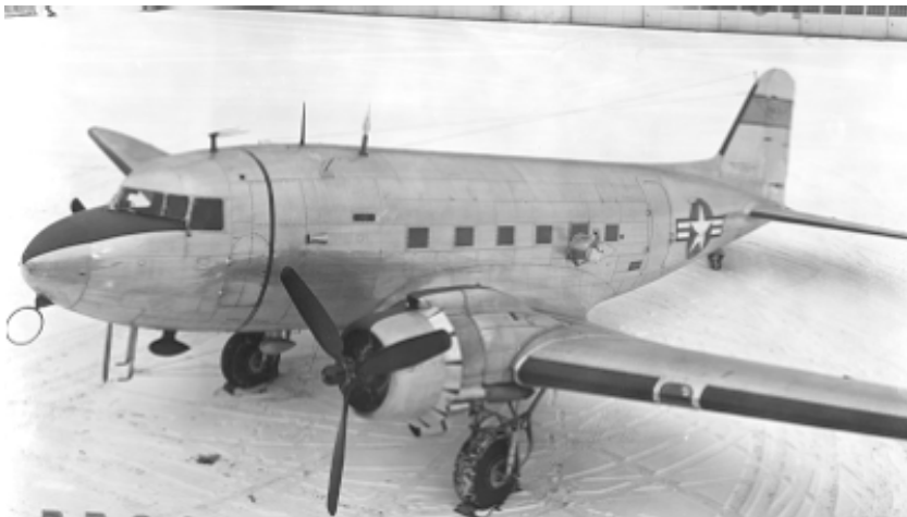
Another stalwart in the Engine Research Laboratory's icing fleet, the C-47 (pictured on a thin sheet of snow) was equipped with Irving Langmuir's multicylinder water droplet collecting device. Among the three vertical objects atop the forward part of the fuselage, the Langmuir instrument is farthest to the right. (Photo courtesy of the Dryden Flight Research Center Historical Reference Collection.)
