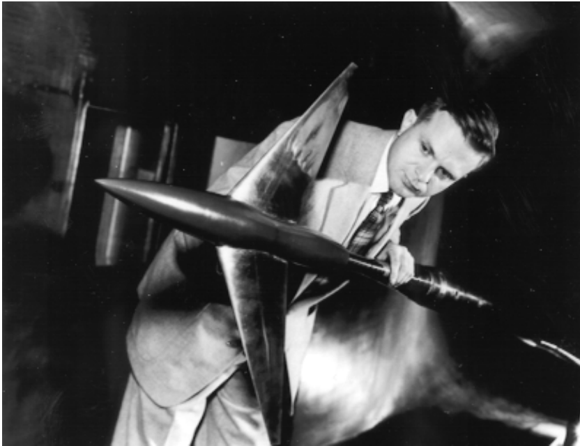
Richard Whitcomb checks a model displaying the "coke bottle" area rule design. He discovered this concept during the late 1940s to reduce transonic drag and achieved this objective again during the mid-1960s, when he conceived of the supercritical wing. Whitcomb predicted five percent more efficiency near Mach 1 using the flat-topped supercritical wing instead of standard airfoils. (Photo courtesy of NASA Headquarters Historical Reference Collection.)
