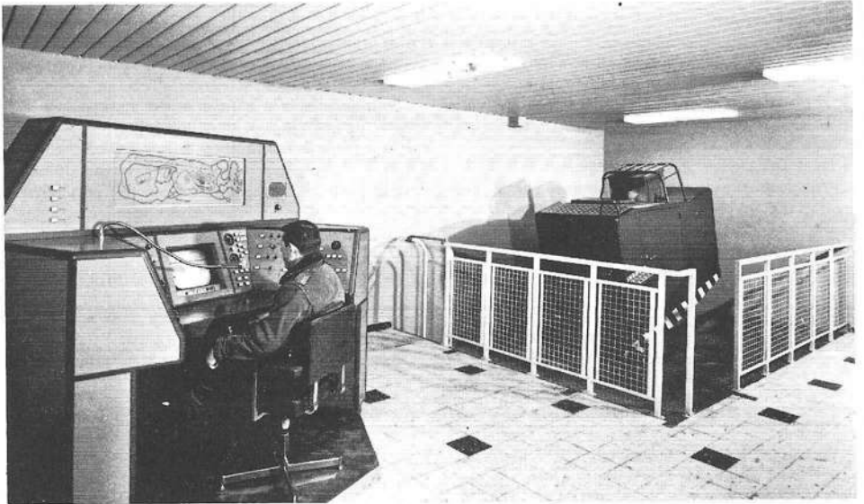
Instructor's console and pupil driver's cabin of LMT AMX 30 tank simulator
