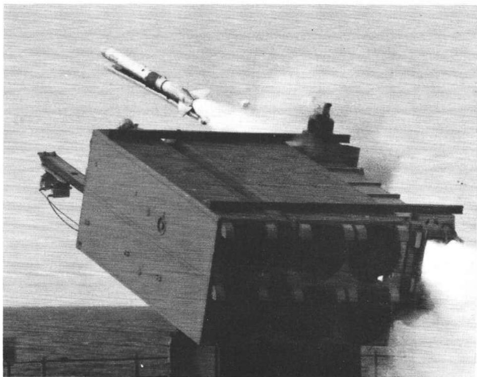
Launch of Sparrow from the new type of launcher/canister which has been developed for this missile. The Sparrow is still resting on its foam launch pad, just before aerodynamic drag separates them. The launching cell from which the missile is fired is the same container as delivered to the ship, thus permitting a simplified and smaller construction than the conventional launcher cells seen on the left
