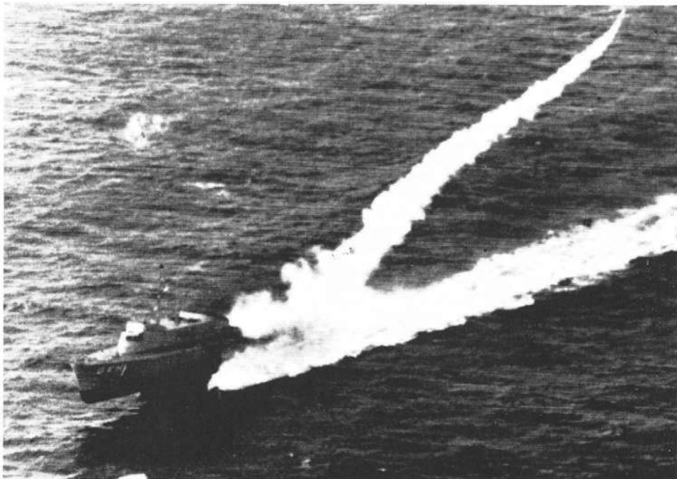
Sparrow missile launched from the development model hydrofoil Plainview (AGEH-1). The launch was effected while the hydrofoil was foilborne
