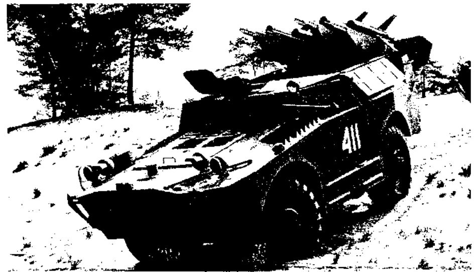
BRDM-1 showing the mounting arrangements for the four Swatter anti-tank missiles (Tass)
