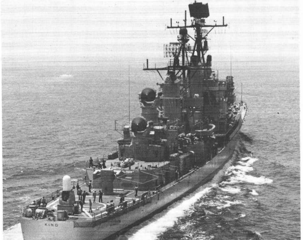
Trials installation of the Vulcan-Phalanx air defence weapon system on the helicopter deck of the USS King
