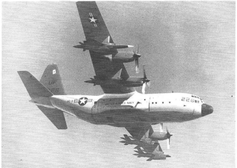
DC-130 drone launch aircraft carrying four Ryan Firebee target drones. Beneath left wing are two subsonic Firebee I (BQM-34A, Ryan Model 124), and under right wing are supersonic Firebee IIs (BQM-34E, Ryan Model 166)
