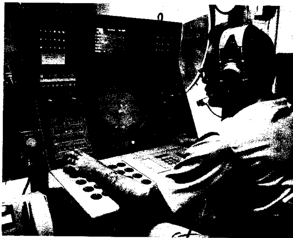
One of the eight AN/UYA-4 computer-controlled display consoles. This one provides missile fire control information to the Missile System Supervisor. The CRT shows a synthetic display with alpha-numeric labels and symbols. A smaller display above is used to present tabular information on a selective basis.
