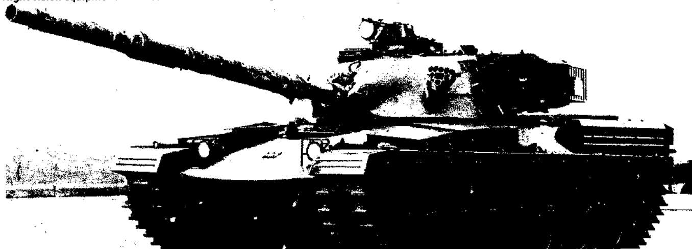
Chieftain Main Battle Tank with 120 mm gun. The thermal jacket on the gun prevents differential heating or cooling on opposite sides of the barrel, from affecting the accuracy of the gun
