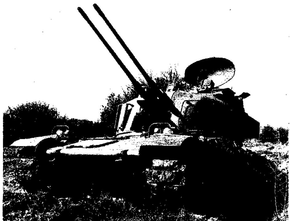
AMX-30 tank with S.A.M.M. turret equipped with Oeil Noir radar
