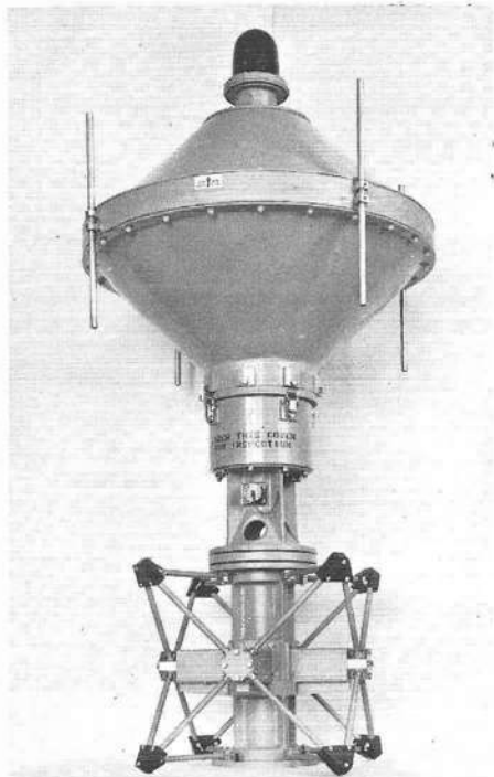
Direction finding antenna unit of the Canadian Model 100 shipborne DF system produced by General Precision Industries Ltd, Montreal. This system has a frequency coverage extending from VLF to VHF, the latter band using the lower array of 16 monopole elements. These can be arranged as crossed-Adcock and parallel dipole in both the horizontal and vertical planes of polarisation. The upper part of the array consists of a pair of multi-turn switched loops for LF and HF direction finding. The balanced dipoles are for sense
