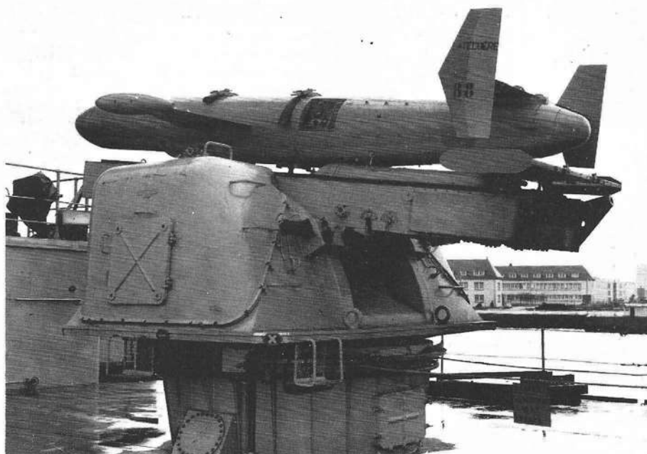
Malafon on its launcher Note how the torpedo head projects from the fuselage
