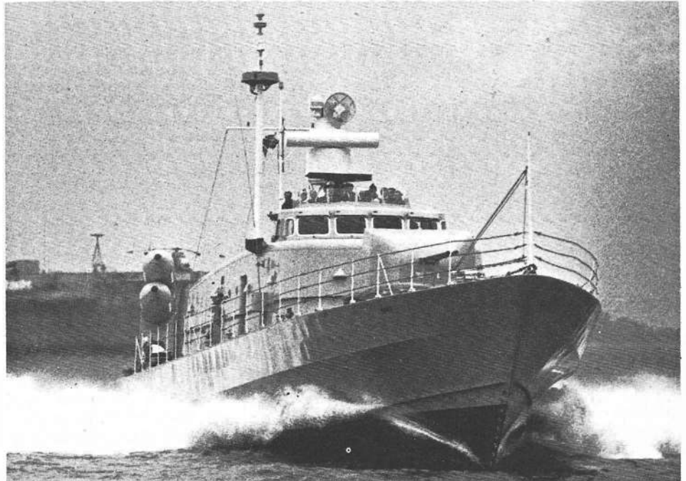
The antenna housing for the Decca RDL Series direction finding system can be seen clamped to the mast of the Vosper Thornycroft Tenacity missile boat. The fire control radar group is the Contraves Sea Hunter system
