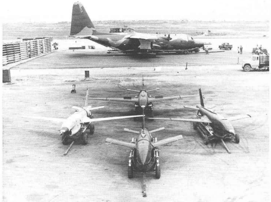
Four versions of the Teledyne Ryan Aeronautical Model 147 drone, with DC-130A launch and control aircraft being prepared for flight
