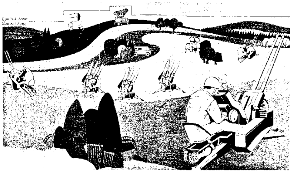
Typical gun-missile layout using the 20 mm Twin Gun. The picture indicates the way in which the "taboo" facility can be used.
