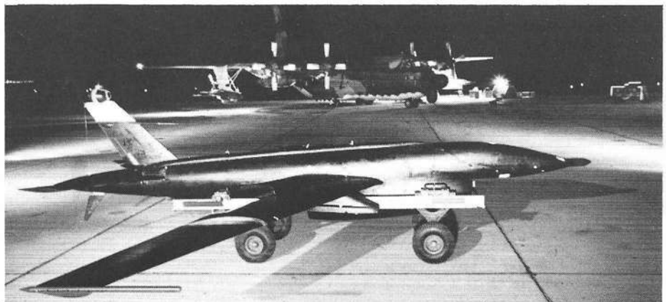
Model 147TE drone awaiting loading. The aircraft in the background, already with two more drones beneath its wings, is a specially-equipped DC-130E launch and control aircraft. Chin radome houses antenna for UPO-3 microwave guidance and control system
