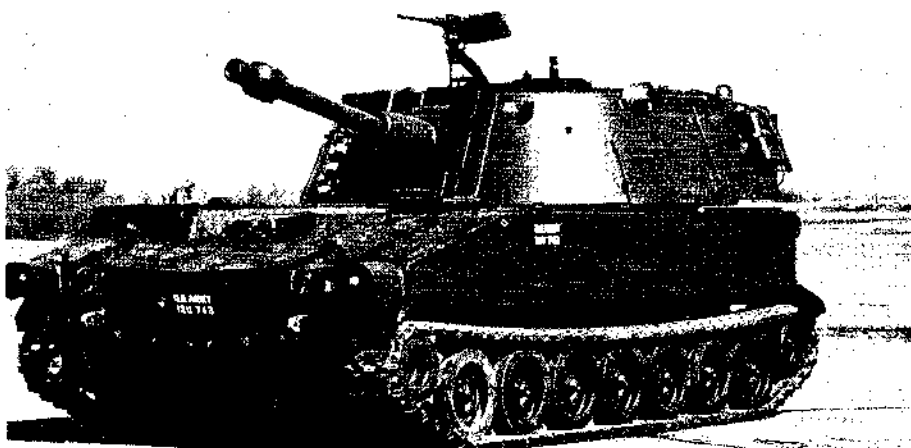
105 mm self-propelled howitzer M. 108. This photograph shows the diesel-powered version (US Army Photograph)
