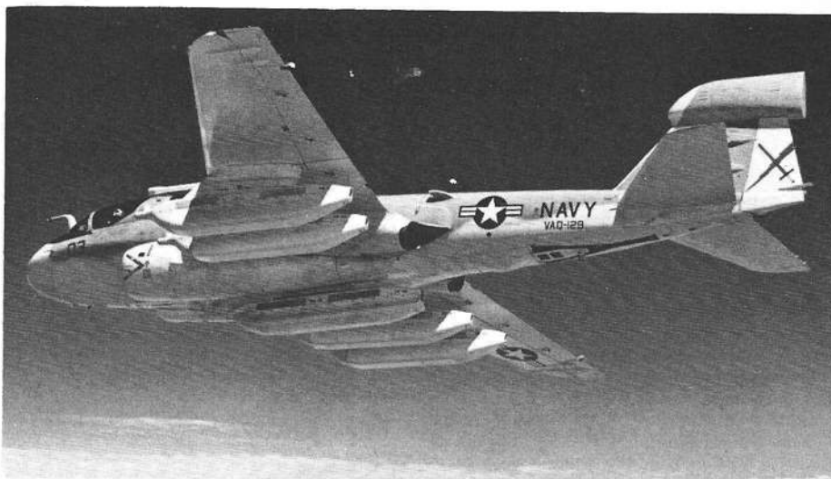
EA-6B aircraft of USN Tactical Electronics Squadron 129 (VAQ-129), showing ALQ-99 ECM pods and fin-top housing for ECM receivers. Each pod contains two jamming transmitters and a receiver; the fin housing contains six antennas and a receiver. Antenna for ALQ-100 deception jammer projects from left wing
