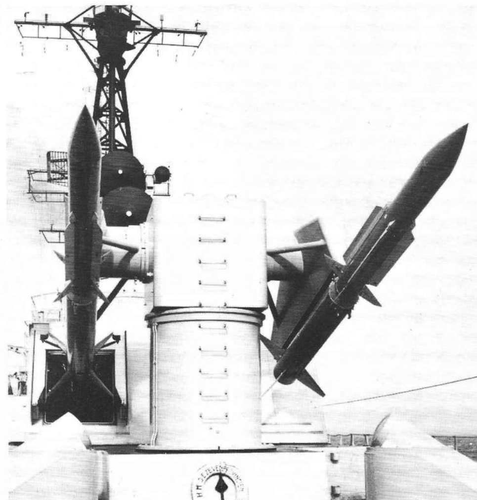
Advanced Terrier missiles on twin launcher of Royal Netherlands Navy cruiser De Zeven Provinciën. Note open reload hatch on left
