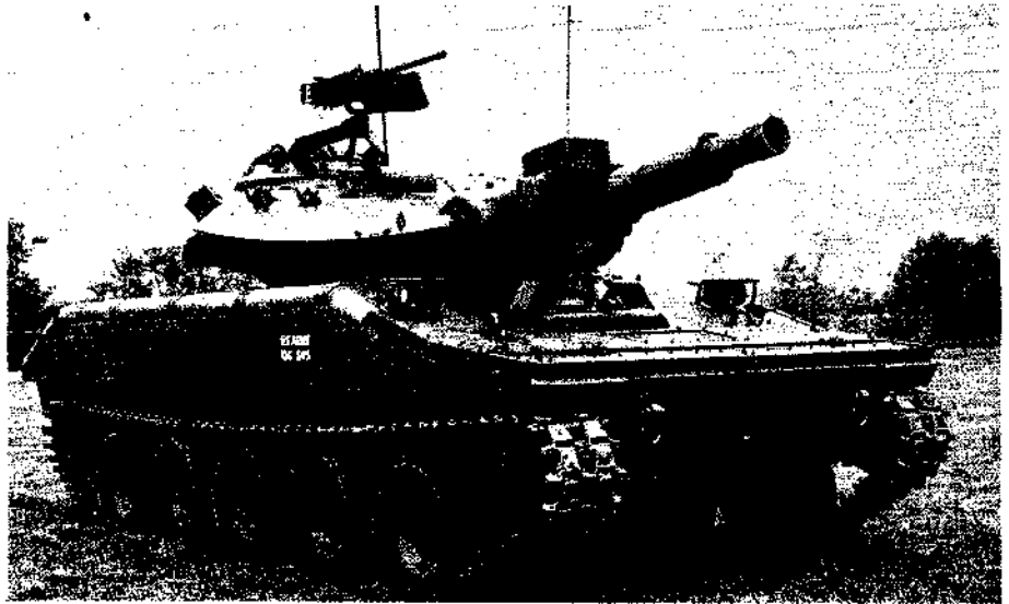
M551 Sheridan with XM 81 152 mm dual purpose gun / launcher
