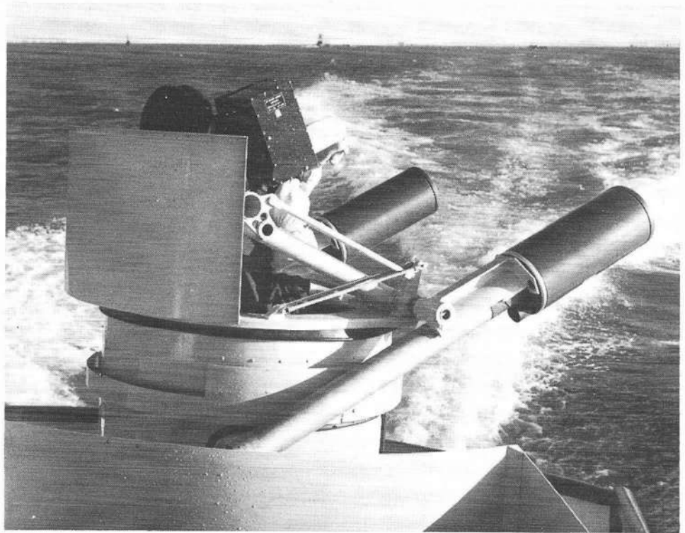
Smallest of the Blowpipe container fits, this twin-launcher/aimer installation can be bolted directly to the deck of any vessel
