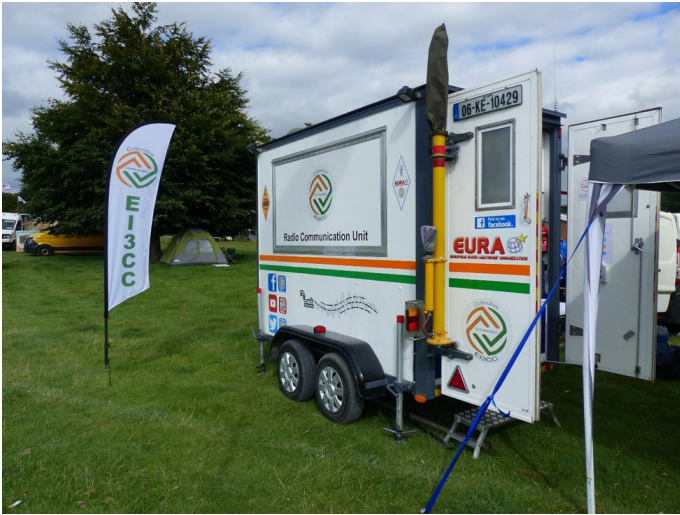
RCU with Clark Mast fitted
