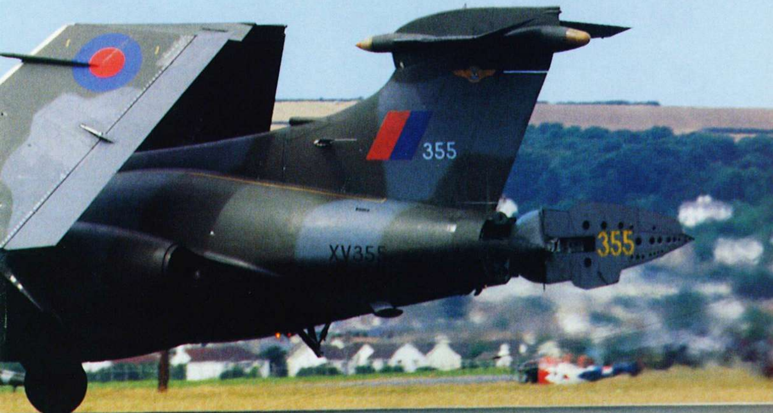
Wing-folding remains a feature of the Buccaneer in RAF service. PRM
