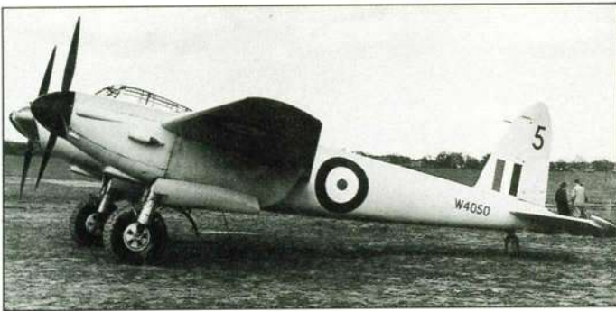
Subsequently serialled W4050, the first aircraft was powered by RR Merlin 21s. Military Aircraft Photographs
