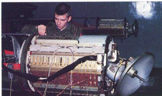
Top left: The Ready-Use Missile Store contains re-load rounds which are constantly fed with dried air. Replacement is a matter of lowering the launcher to the horizontal position and installing a new round carried on a side-lifting vehicle. Above left: With covering panels removed, a Bloodhound is hooked-up to the Missile Overall Test Equipment (MOTE) for fault analysis. Checking the electronics is 22 year-old Junior Technician Paul Carter from Cleethorpes. Above right: 'Our warriors in serried ranks assembled' Never quaver (they conceal it if they do) — W.S. Gilbert, The Mikado . Like birds, the missiles stand with their backs to the prevailing wind — which just happens to mean that they point East. Paul Jackson photographs
