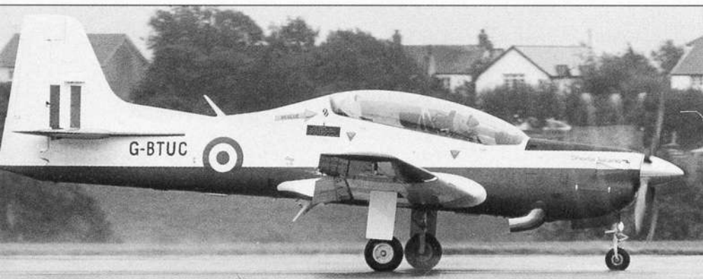
Below: Shorts modified an airframe to take the 1,151 shp TPE331 engine. PRM Bottom: The Tucano in RAF training colours. PRM
