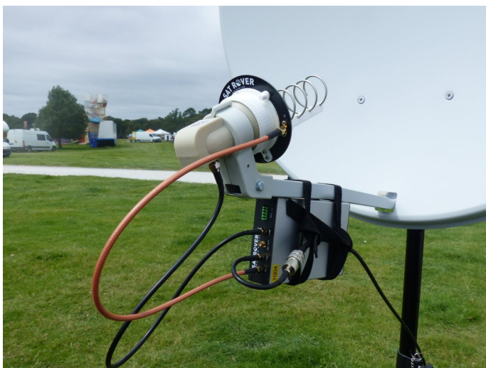
Fig.7 Twist the LNB in a clockwise direction to achieve best signal strength - this should correspond to a skew angle of 21–22 deg
