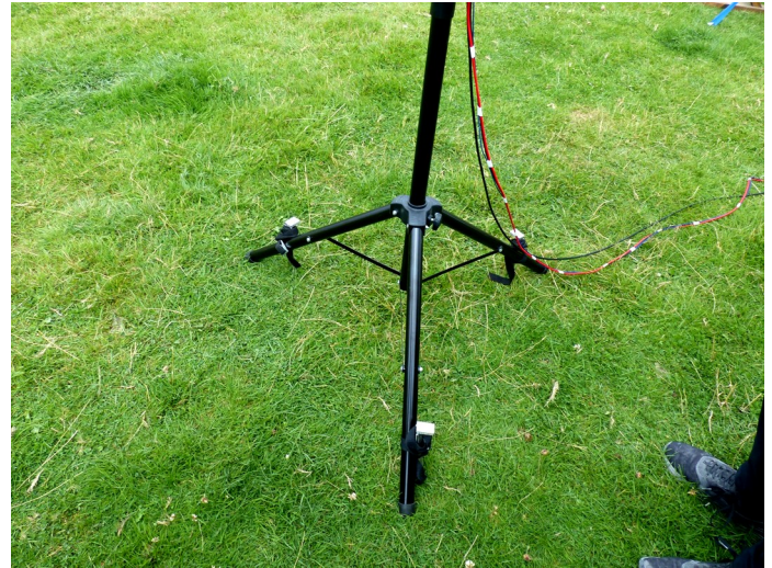
Fig.4 securing the feet of the tripod with pegs and straps
