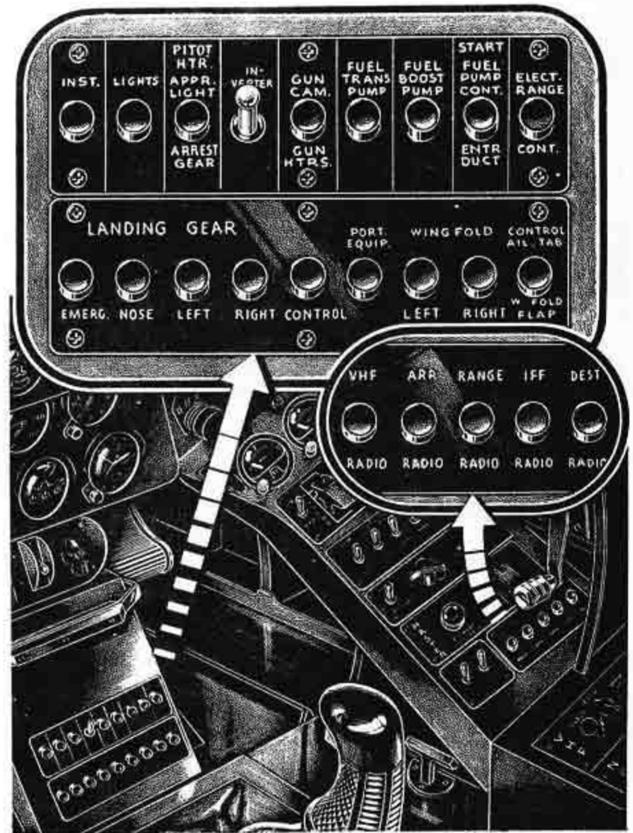
Figure 1-18. Main Distribution Panel
