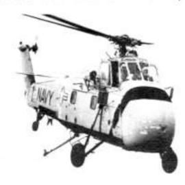
Texas, the SH-34J differed from its predecessor by incorporating devices to measure ground speed and altitude with radar, automatic engine RPM controls; an automatic hover coupler; and improved flight instruments and cockpit arrangement. Now, with automatic stabilization equipment and the approach coupler, ASW helicopter pilots could descend to and remain in a hover automatically.
