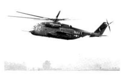
The CH-53E will be able to quickly remove disabled aircraft from a carrier deck, and load heavy cargo rapidly using the wide rear ramp, the roller floor, and tie-down fittings in the cabin. Refueling may be done on shore or on deck using pressure or gravity equipment. With a high-density seating arrangement, the CH-53E will be able to transport 55 troops.
