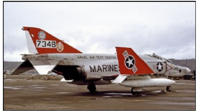
RF-4B 157348 was used by the Naval Air Test Center (NATC) at NAS Patuxent River (MD) as a pattern aircraft for the 'Project Sure' upgrade programme for the RF-4B fleet. This included an onboard systems upgrade as well as airframe strengthening. The aircraft has a red tail with the NATC badge on top and the Project 'Sure' badge on the bottom of the tail. (Stephen Miller)
