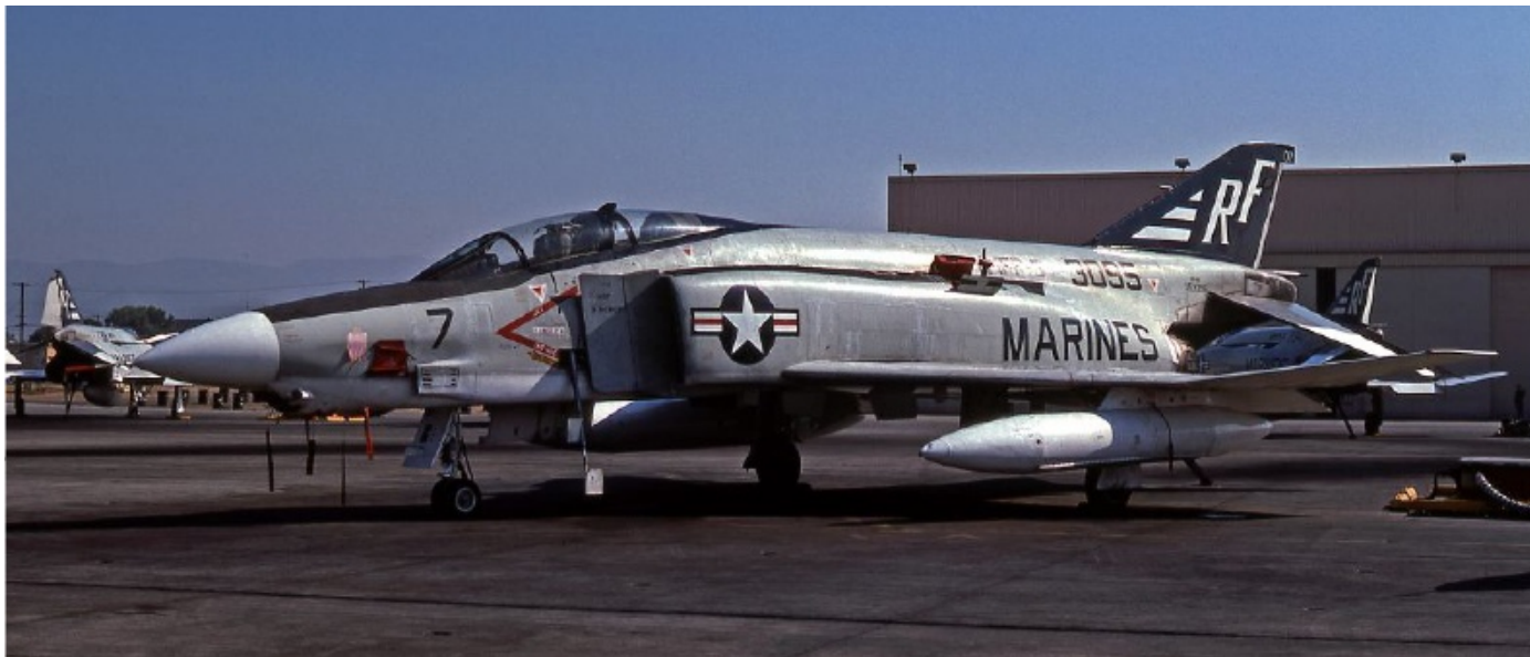
RF-4B 153095/RF-7 of VMFP-3 at MCAS El Toro in oct78. Note the extended ram-air turbine. The tail markings are dark blue with white markings. The markings on the fuselage and the anti-glare shield are black. (Bruce Trombecky via Patrick Roegies)
