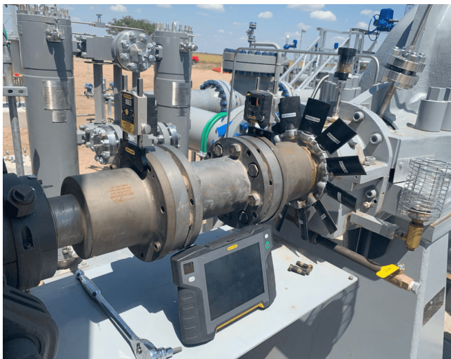
Laser shaft alignment system mounted using magnetic axial brackets.
