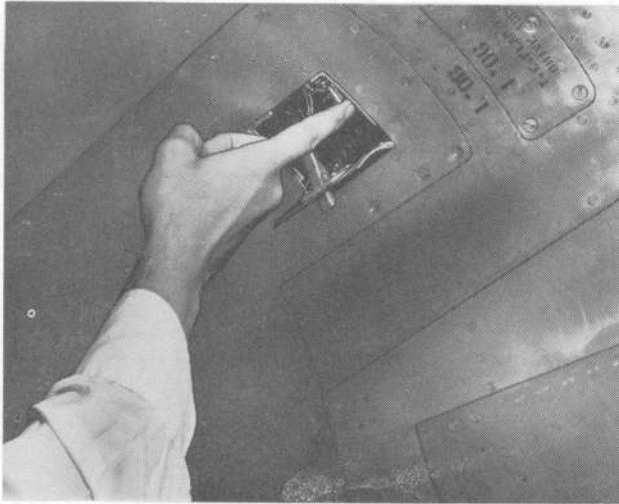
CLOSING OF DESTRUCTOR INSTALLATION HYDRAULIC RELEASE SWITCH. (LANDING GEAR DOOR RELEASE SWITCH)
