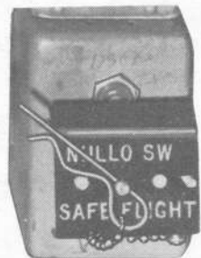
AUX NULLO SWITCH BOX (IN E COMPARTMENT)
