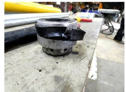
Damaged seal from wrong lubricant
