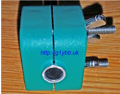
Using Clamps to mark Centreline
