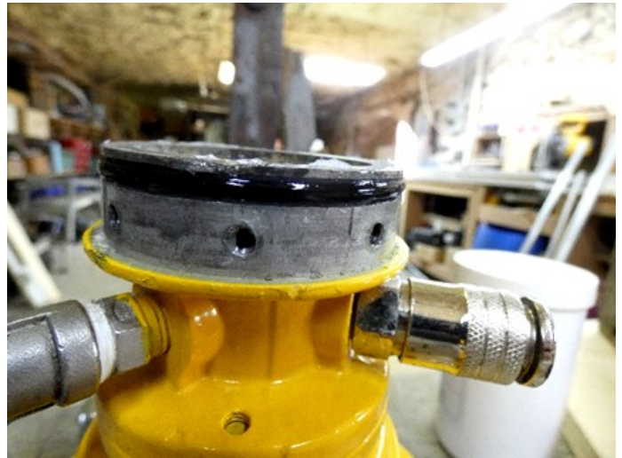
Seal fitted and wiped with the Clark silicone
