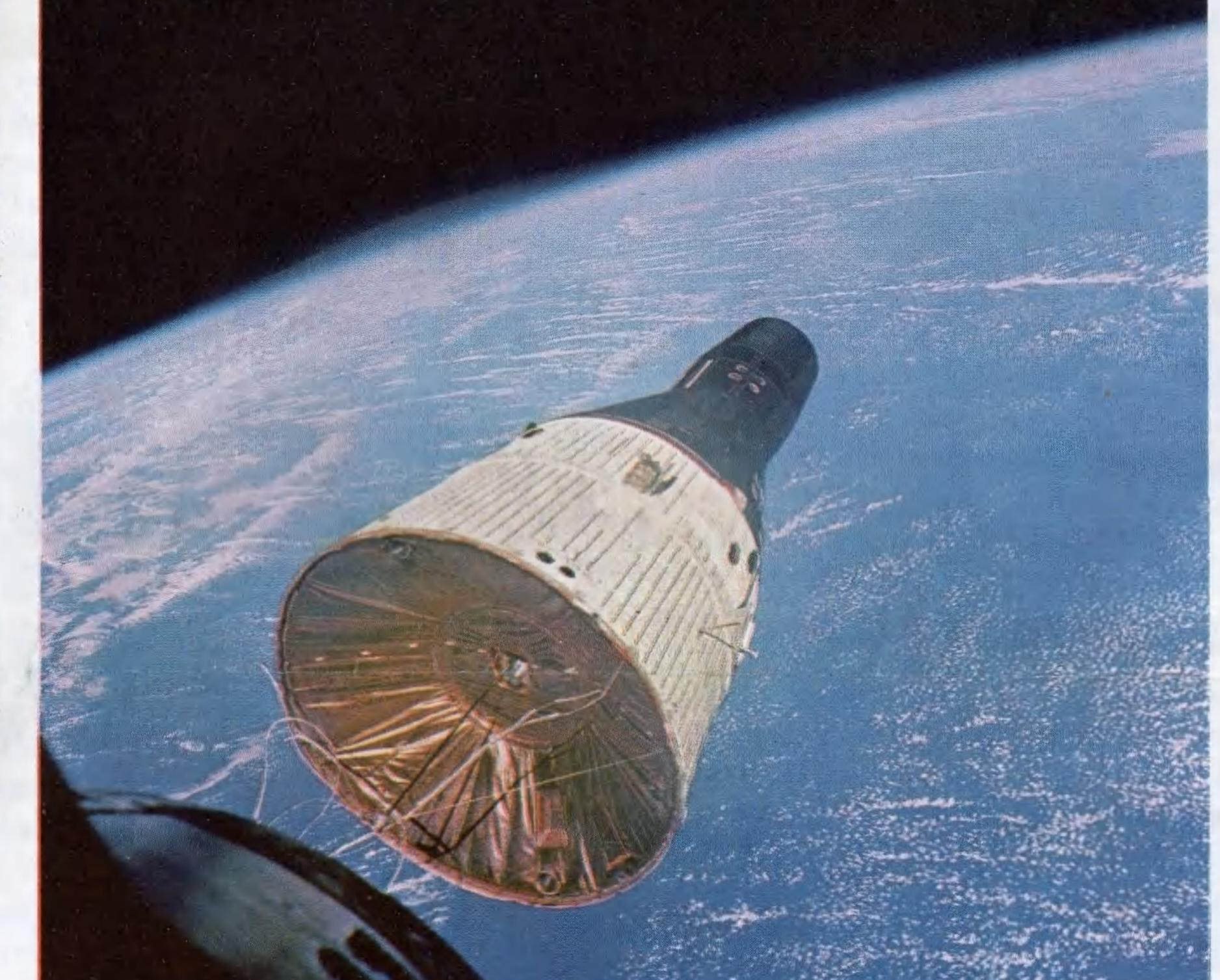
thermal blanket for protecting equipment. Adapter is 37 feet from Gemini 6 window from which photo was made.
