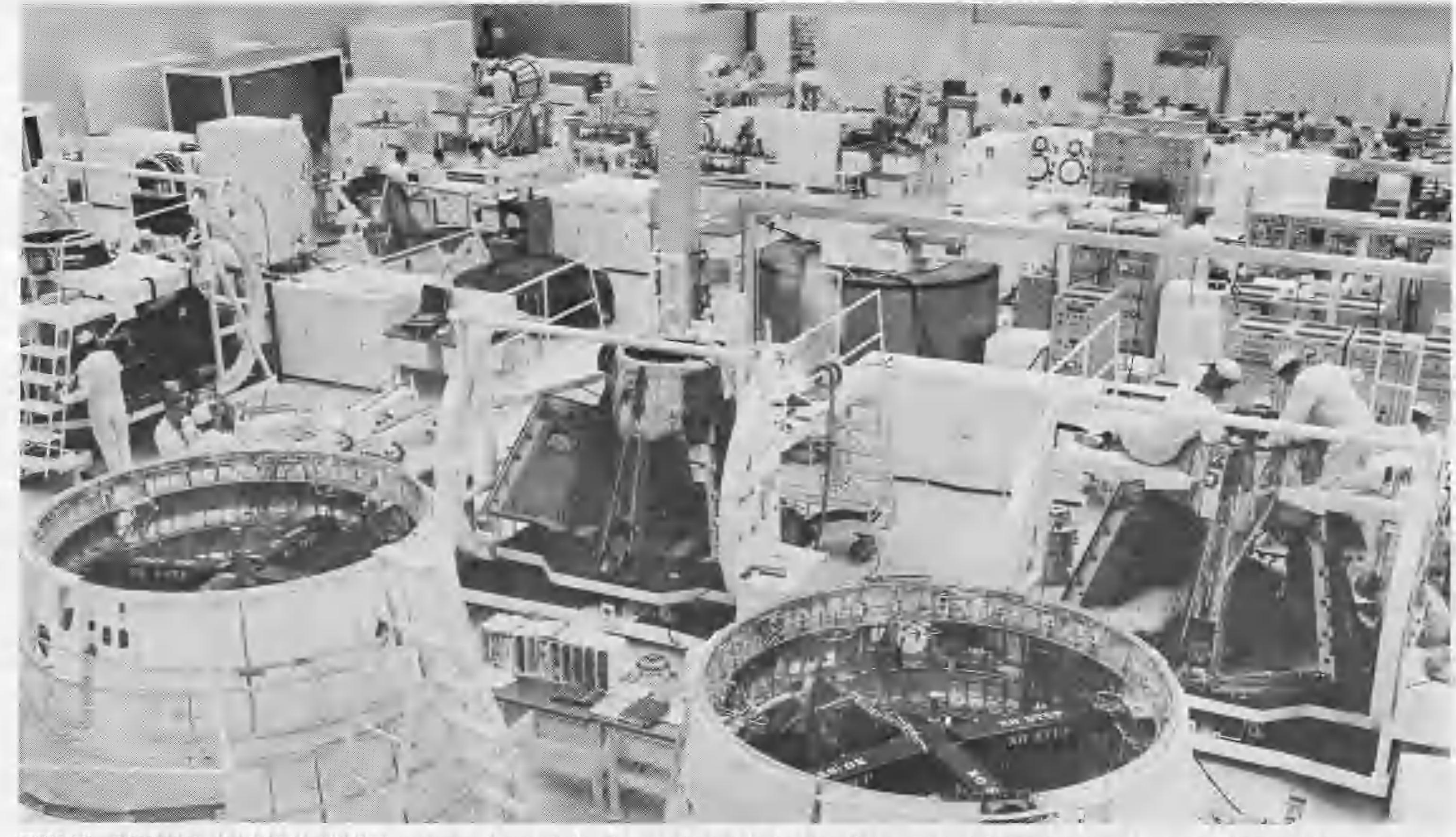
FINAL GEMINI FABRICATION was performed in Space Center's huge clean room where temperatures and humidity are carefully controlled. Clean room's powerful filtration systems remove virtually all dust and other minute particles from the air.
