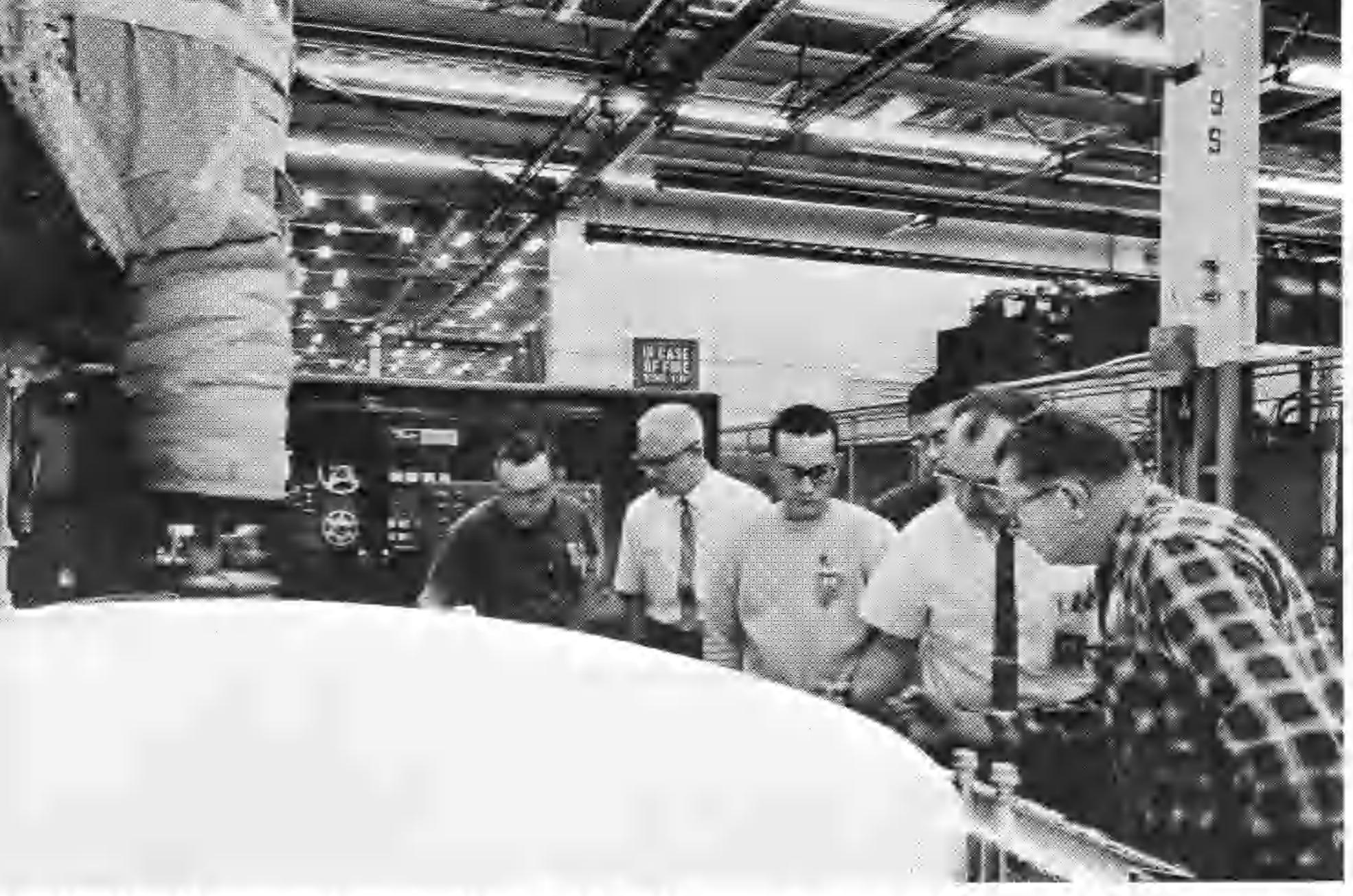
FORMING OF THE GEMINI HEAT SHIELD required precise machining, careful and frequent inspection to maintain the close tolerances that were an absolute necessity. Here a team of McDonnell machinists, inspectors and foremen perform one of many detailed inspections of a 90-inch-diameter, dish-shaped heat shield.
