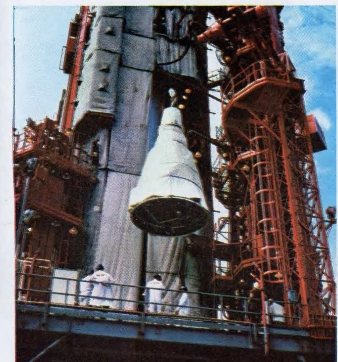
GEMINI 5. Spacecraft, shrouded for protection, is hoisted up gantry of Launch Pad 19 preparatory to mating with its Titan II booster.
