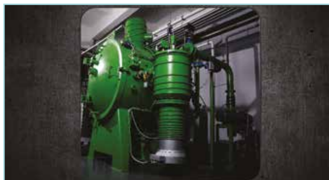
Equipment for precision plasma nitriding nanolayer nanocomposite coating deposition
