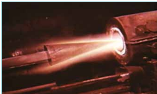
Testing of thermal shielding model on gas-dynamic bench
