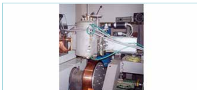
Melt-spinning equipment for amorphous and nano-crystalline soft-magnetic ribbons production Annual capacity - 5 tons
