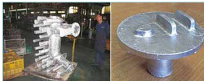
Castings for machine-building (including aircraft) manufactured using developed MHD-equipment and technologies
