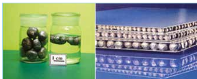
Al sandwich panels and foamed granules with density less than the density of water
