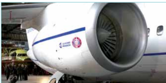
Engine nacelle of Antonov An-148 made of composite material
