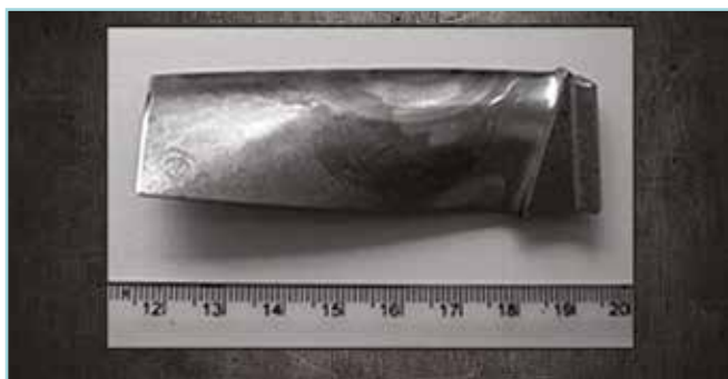
Gas turbine fan blade subjected to local RHT
