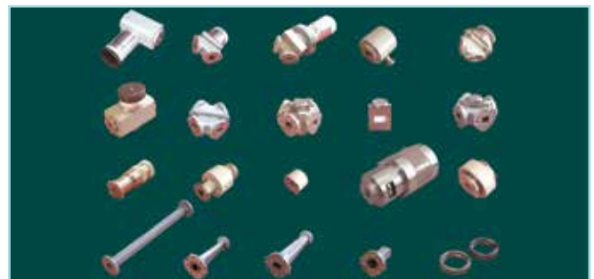
Some wideband THz components, developed in quasioptics department
