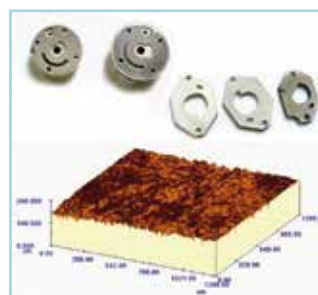
Surface after microarc oxidation and parts, after treatment with MDO
