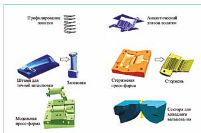
Computer models for complex pre-fixtures and die molds for blade manufacturing
