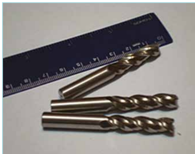
Tools made from steel R9M4K8-MP produced from powder using of STTT
