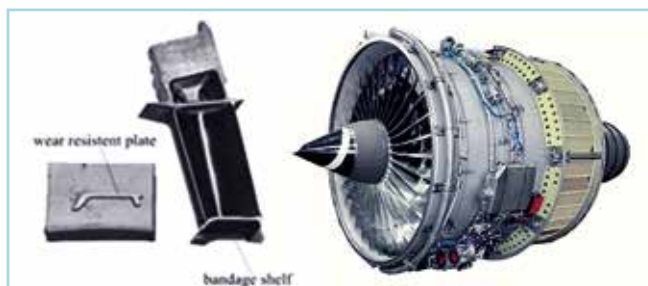
Turbine working blade with wear-resistant soldering for D-18T turbojet bypass engine
