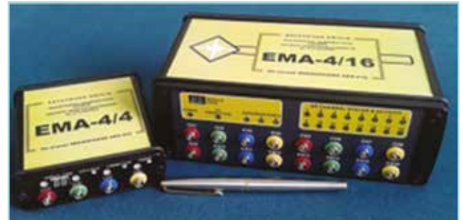
EMA-4 devices based on the 4-channel and 16-channel modules
