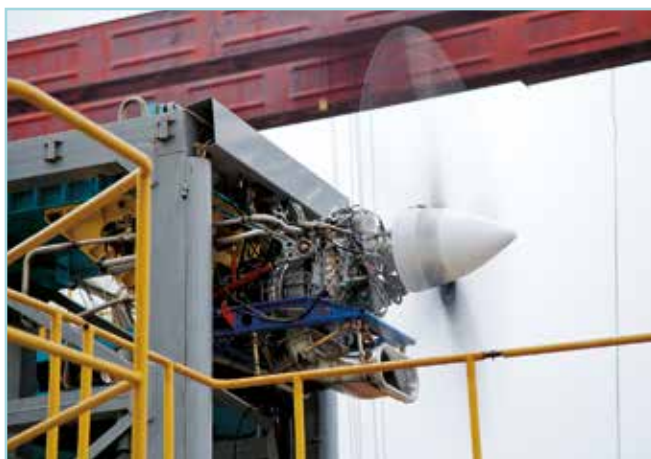
AI-450C turboprop engine for a modification of a single-engine trainer aircraft DART-450
