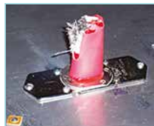
Antenna after the lightning test
