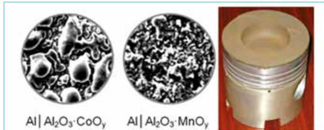
Catalytic oxide coatings for internal combustion piston
