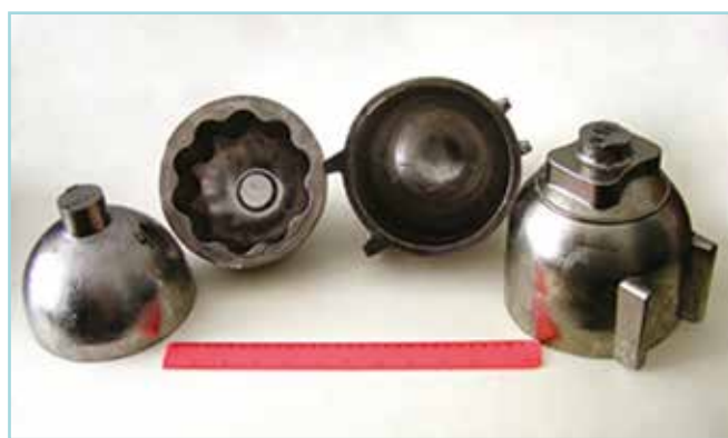
Lids and frames of solid flight recorder of sound information produced by casting technology with the use of titanium waste
