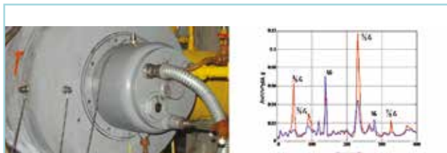
Manifestation of the fractional harmonics of the rotor frequency in the presence of a defect
