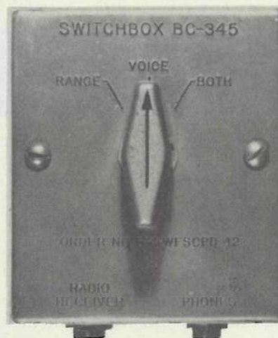
Fig. 66 Filter Switch Box
