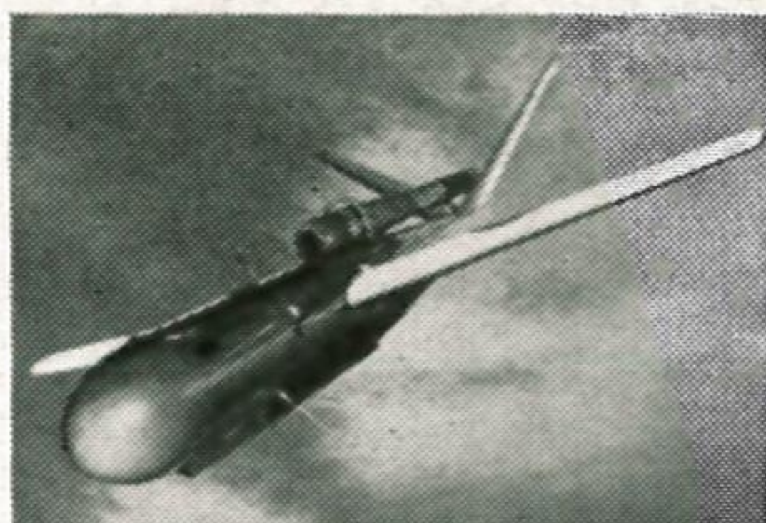
THE KDD-1. The "Katydid," also a guided missile, is radio-controlled and powered by a McDonnell reso-jet engine. It is used as a target in training aircraft gunners.
