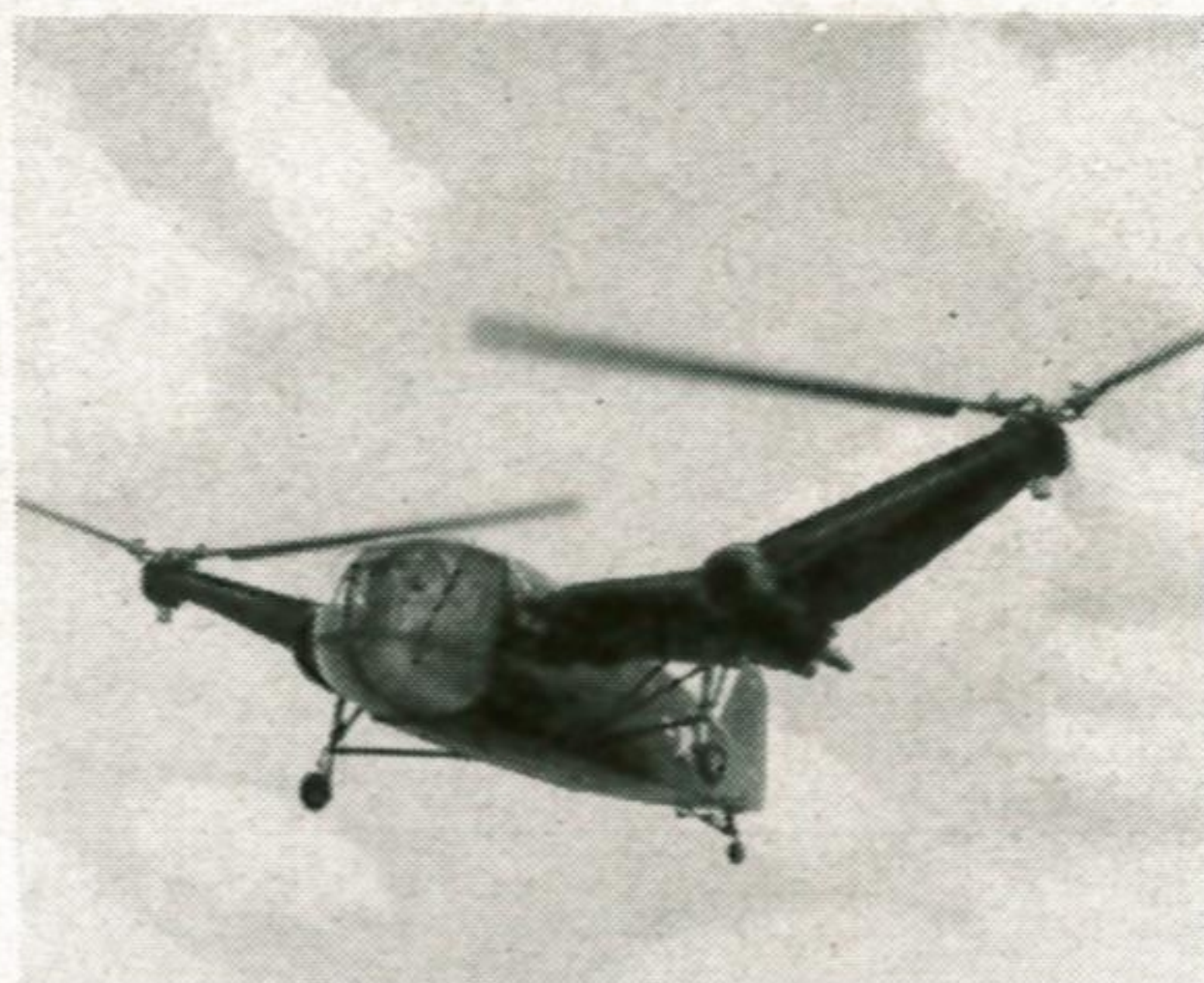
THE XHJD-1. Not only the world's largest helicopter, the "Whirlaway" is also history's first twin-engine helicopter. Designed and developed by McDonnell and the Navy, the XHJD-1 is now undergoing advanced flight research development.
