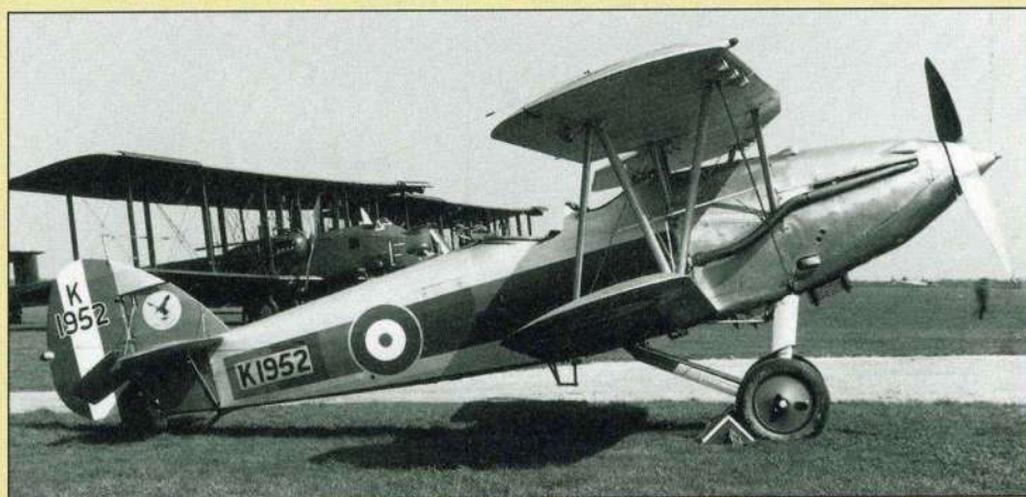
Close-up of K1952, a Hart Fighter of No 23 Sqn. The aircraft in the background is a Vickers Virginia. James D Oughton collection
