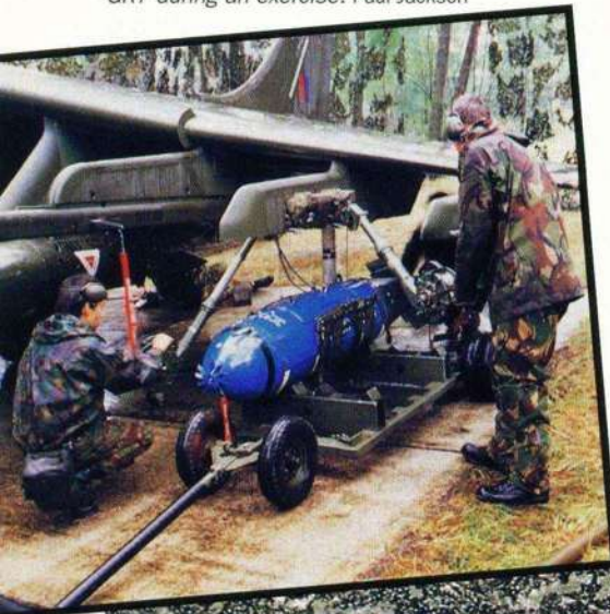
A BL755 cluster bomb is winched onto a Harrier GR7 during an exercise. Paul Jackson
