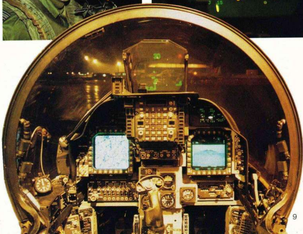
Right: The Harrier GR7's instrument panel is dominated by two multi-purpose screens for infra red imagery (right) and the moving map display (left), plus a central control panel and the wide-angle HUD. Paul Jackson
