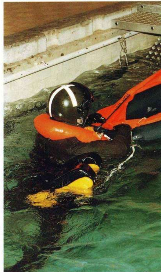
Above: Evaluation of ease of boarding a single seat life raft conducted in the experimental pool at the Institute.
