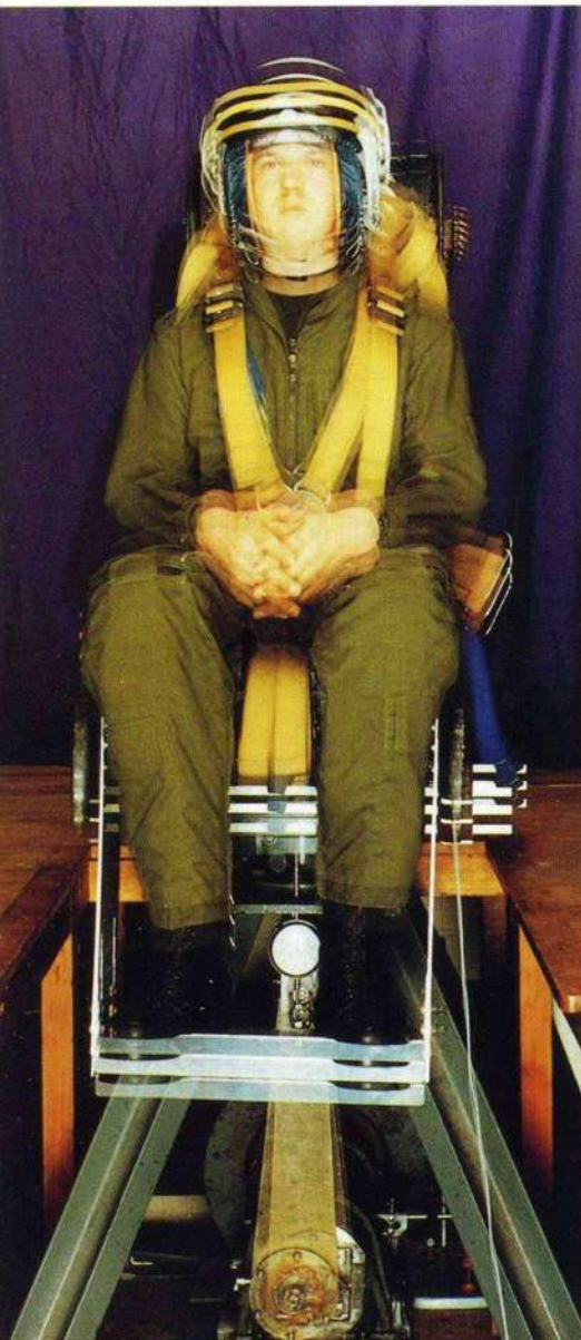
Below: Subject undergoing vertical vibration tests in the Institute vibration laboratory.
