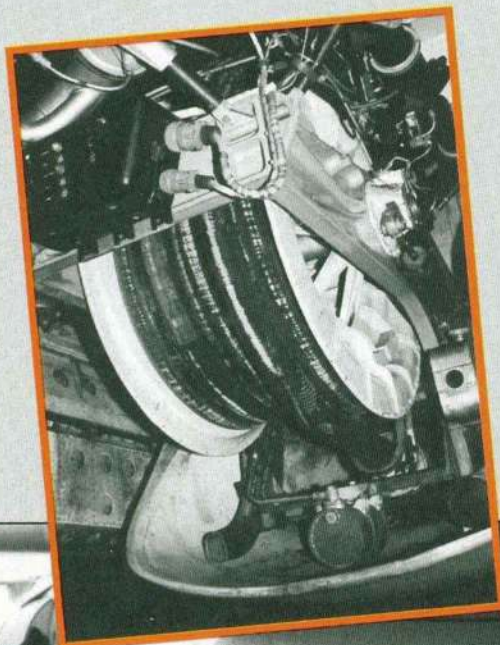
Inset left: Mk 17B HDU inside the bomb-bay, looking towards the rear. Below left: Mk 20B refuelling pod on the Victor's port side. Below right: The Mk 17B HDU in the lowered position showing the basket and signal lights. Photographs Lindsay Peacock
