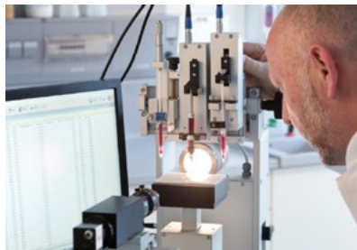
LAUDA Surface analyser for contact angle measurement (surface tension, interfacial tension, wettability).
