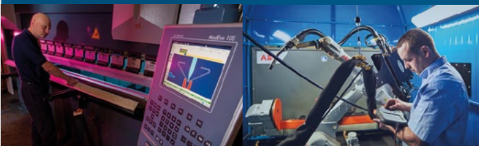
Press braking - 200 tons 4000 mm
