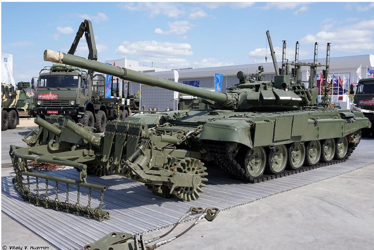
(T-72B3 with TMT-K mine roller at the Army-2018 defense expo. Via vitalykuzmin.net )
