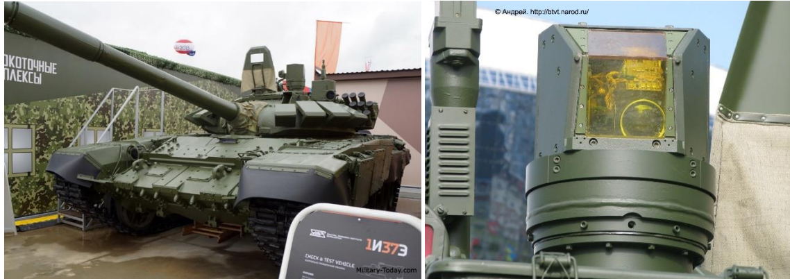
(T-72B3 Model 2014. The PK-PAN sits on the right side of the Sosna-U and behind the commander's cupola, left. Close up of the PK-PAN, right)
