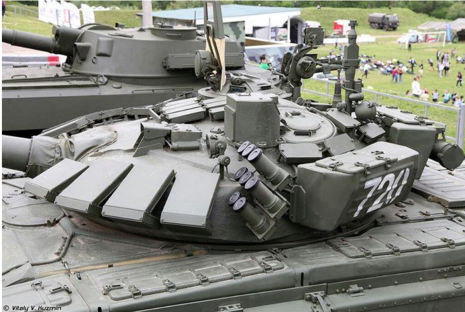
(Side view of the bank of smoke mortars on a T-72B3 Model 2013, the rubberized caps on the ends of the smoke mortar rounds will remain fixed when firing. Via vitalykuzmin.net)
