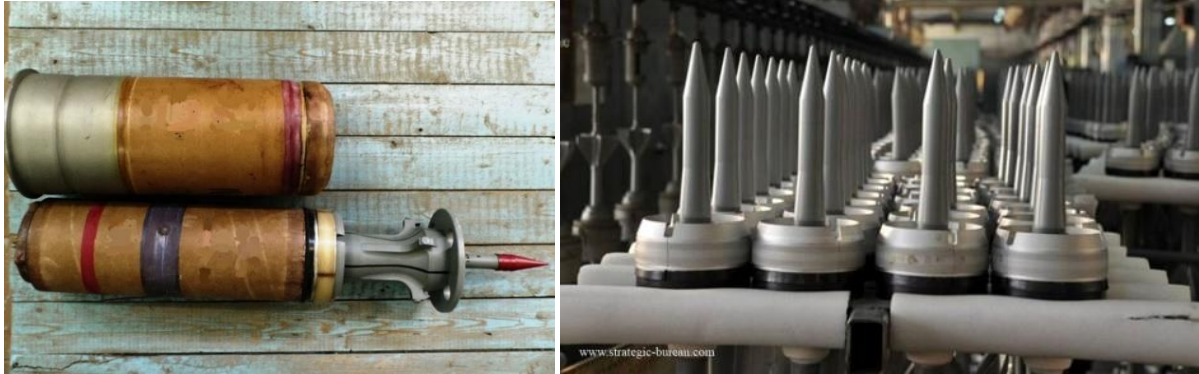
(3BM59 Svinets-1 APFSDS projectile and 4Zh96, left They can be easily identified by the presence of a red band. 3BM42 Mango APFSDS projectiles on the assembly line, right)
