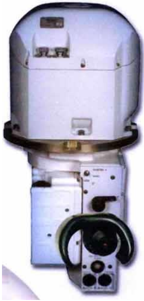
(ESSA sight for the T-90A, left. T-72B2 with Sosna, right)
