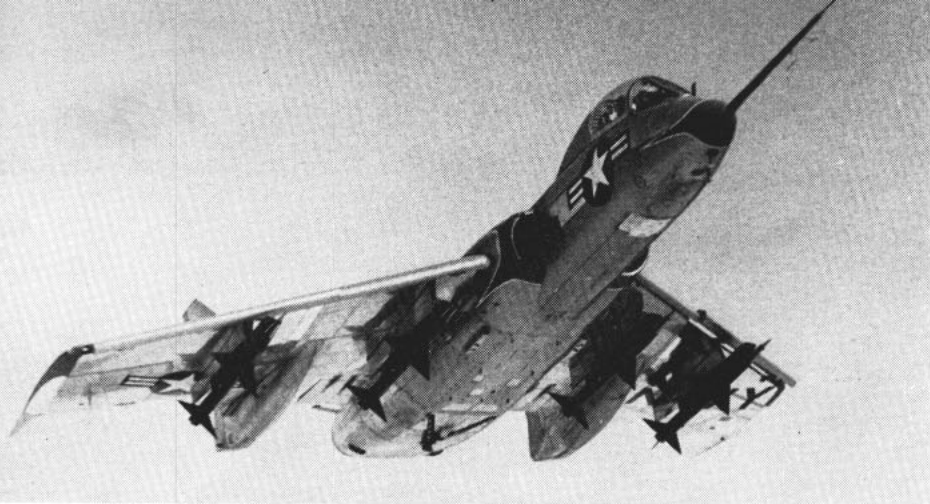
BIRDS FOR THE BIRDS — Air-to-air guided missile Sparrow now operational with the Fleet is taken aloft under the wings of a carrier based F7U-3M Cutlass.
