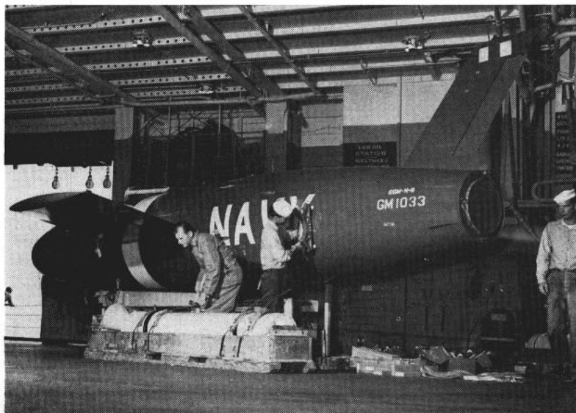
MISSILEMEN COMING UP —Missile and launcher ride elevator to flight deck. Below: Work begins on hangar deck where Regulus is rigged for flight.
