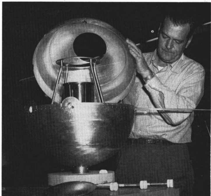
INSIDE STORY — Plastic foam encased electron package is put into gold plated housing and 'lid' is attached.
