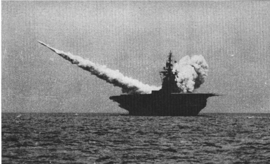
HIGH TEST — Navy surface-to-surface guided missile roars off its launching platform on a test flight using JATO rocket bottles to speed its getaway.
