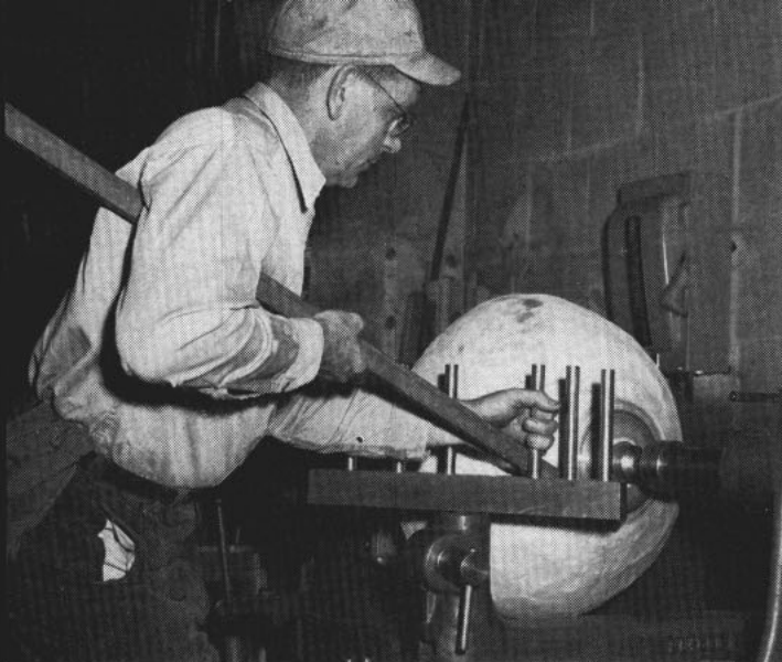
HOW TO MAKE A SATELLITE — NRL machinists work aluminum blank into shape for the satellite's skin.
