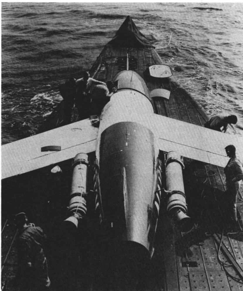
UP FROM BELOW —Guided missile submarine USS Tunny (SSG 282) prepared to launch Regulus from her deck using JATO bottles for initial flying speed.
