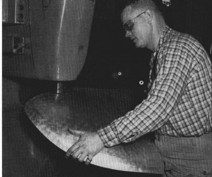
HOW TO MAKE A SATELLITE — NRL machinists work aluminum blank into shape for the satellite's skin.
