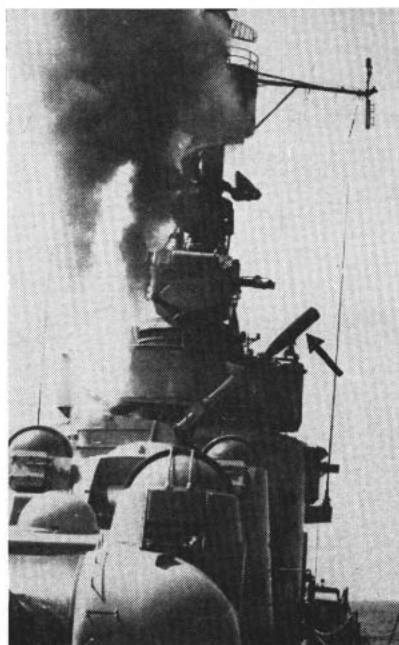
ALL WET—Anti-sub rocket, Weapon Able, is uncovered and fired on board USS Wilkinson (DL 5). Arrow (right) points to rocket leaving its launcher.
