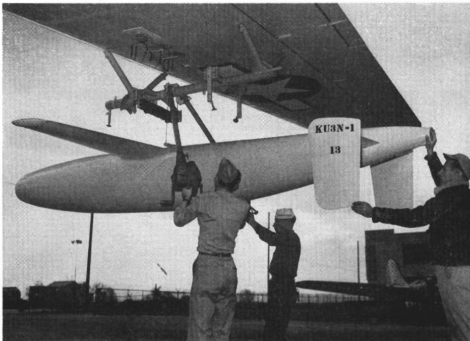
'EARLY BIRDS' — Navymen attach an air-to-surface guided missile to parent plane in 1946 experiments. Below: Loon missile is tested in JATO take-off.
