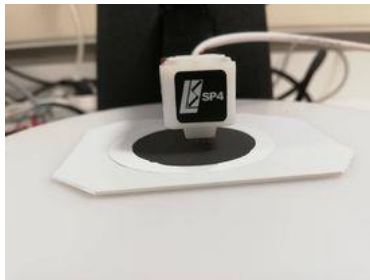
Four-point probe electrical conductivity measurements of different samples transferred on polystyrene substrate
