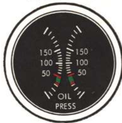
ENGINE OIL PRESSURE (FRONT PUMPS)
