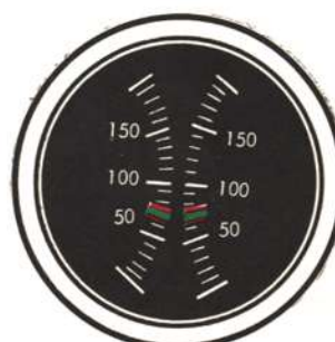
ENGINE OIL PRESSURE (REAR PUMPS)
