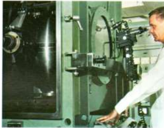
Electron beam welding assures precise welding of exotic aerospace materials.
