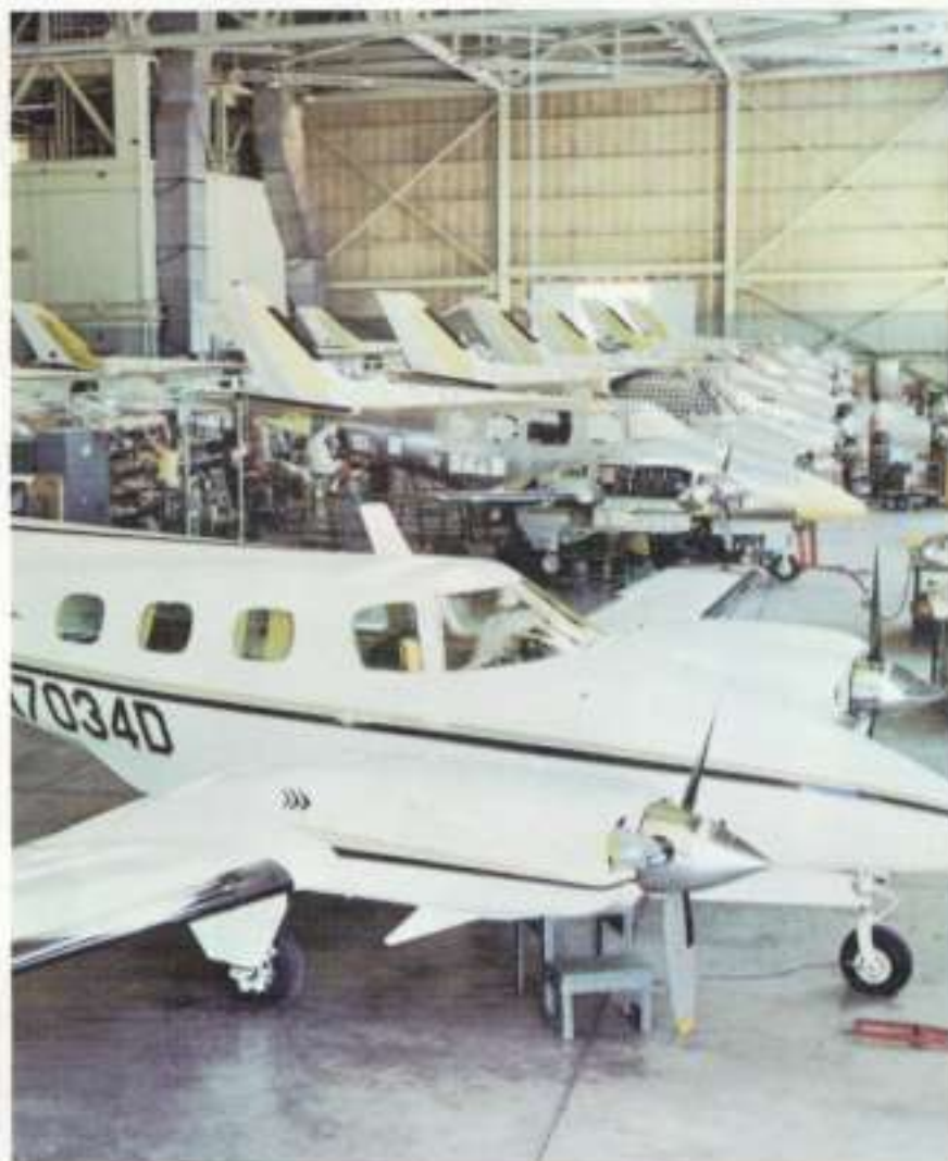
Major production activity at the Salina Division is assembly of the new pressurized, twin-engine Beechcraft Duke.
