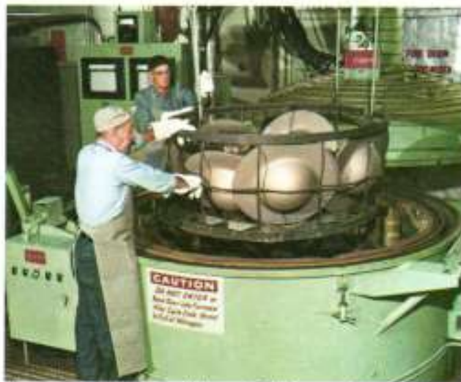
Vacuum furnace with molybdenum hearth heat treats special space-age alloys up to 2,800° F.
