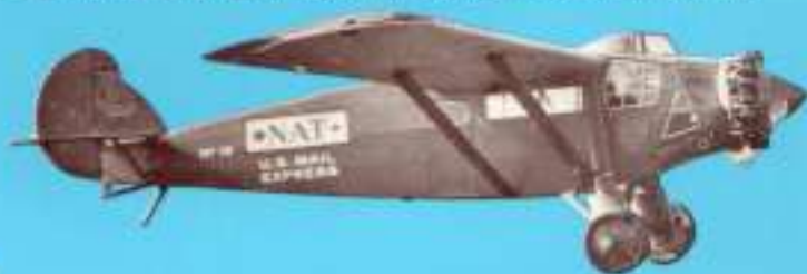
MODEL 5000 TRAVEL AIR. A design competition sparked the creation in 1926 of this famous Travel Air, a five-place, high-wing cabin monoplane and the first aircraft built to airline specifications. The Model 5000 won the demonstration competition and became the first unit of a National Air Transport's airline fleet operating day and night between Chicago and Dallas.
