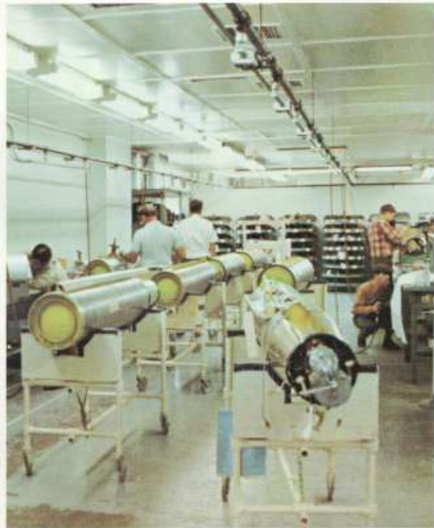
U. S. Navy's rocket-powered, supersonic AQM-37A missile target is assembled and fueled at Boulder Division.
