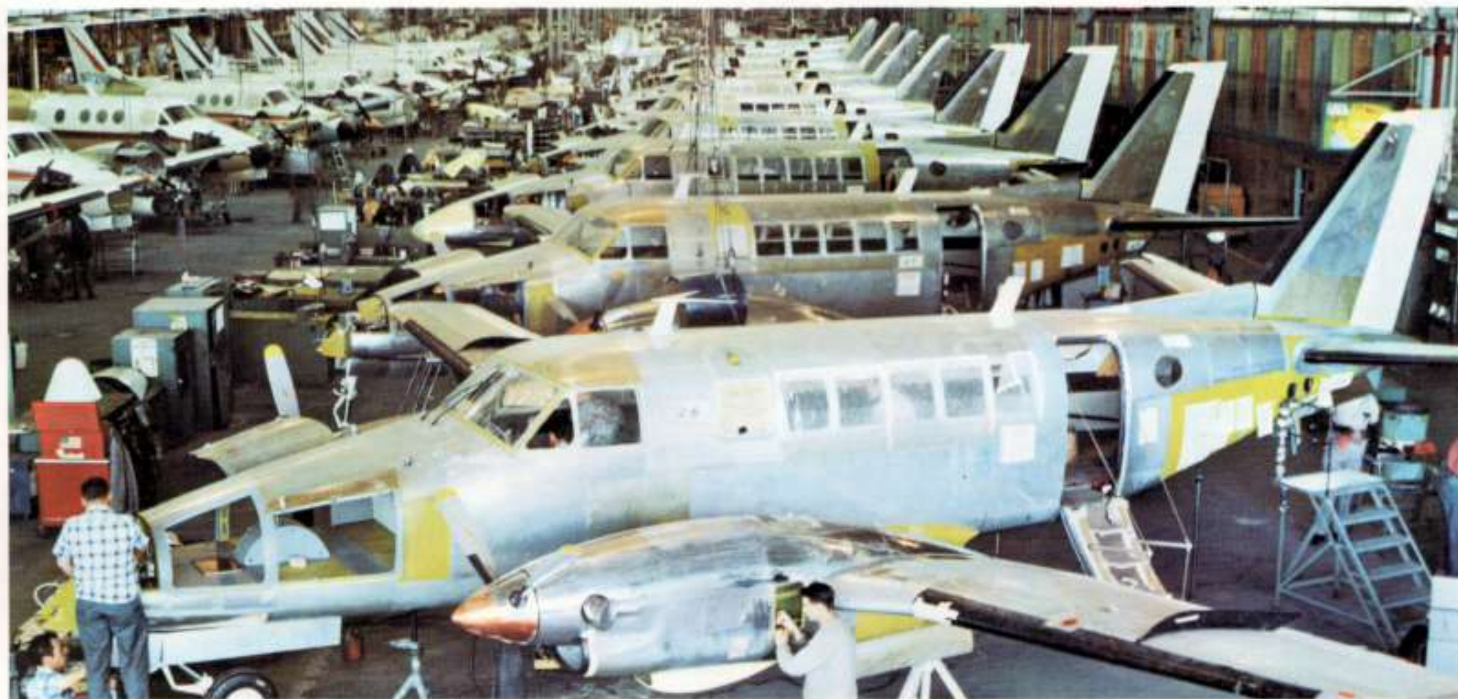
Turboprop Beechcraft King Airs and Beechcraft 99 Airliners occupy Plant I final assembly line.
