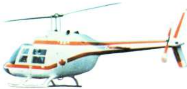
Beech Aircraft produces the complete airframe for Bell's five-place, turboprop JetRanger helicopter.
