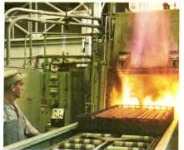
Brazing equipment includes endothermic generator, provision for air, oil quenching.
