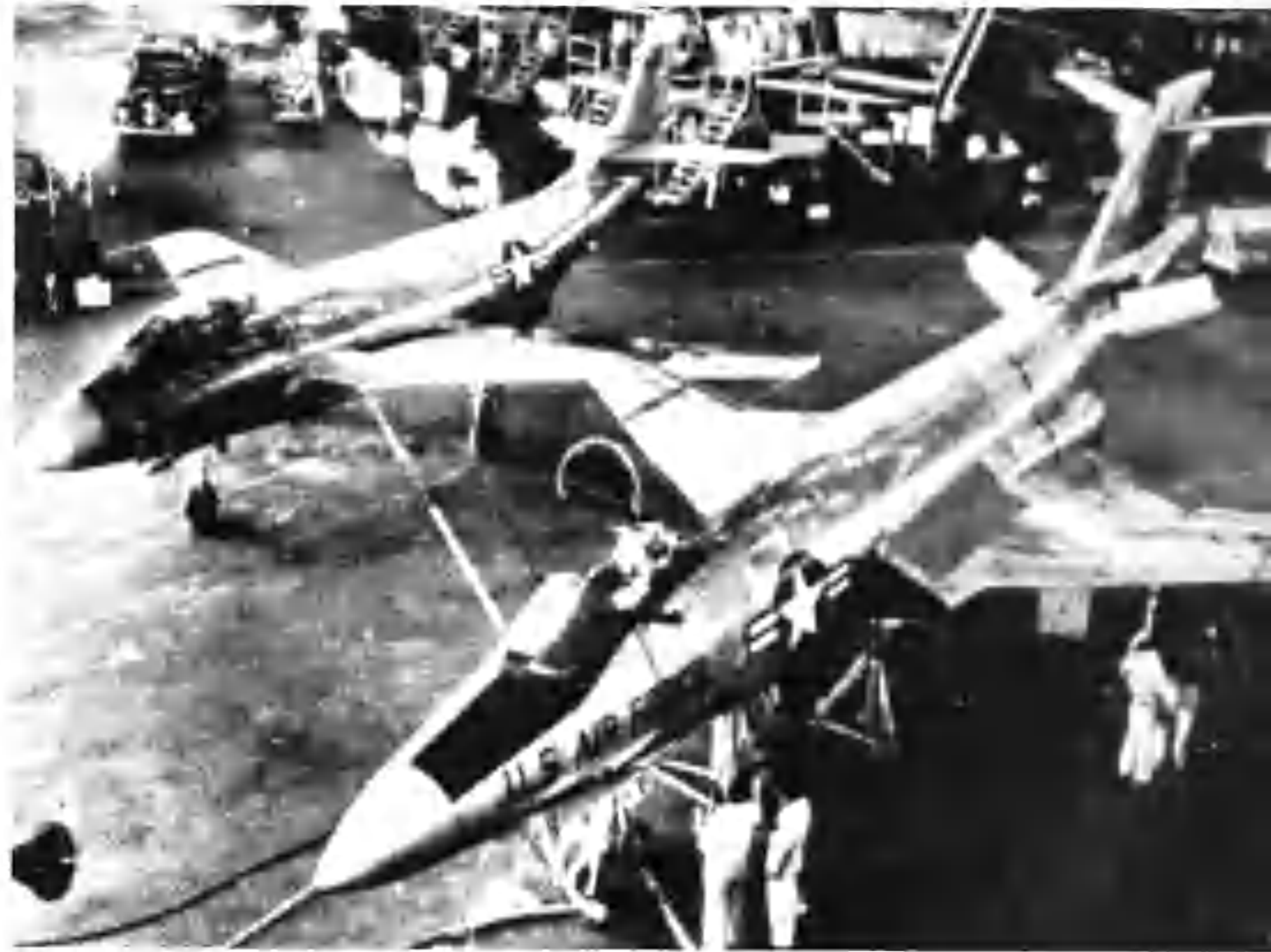
Size is Everything. This side-by-side comparison with the XF-88 shows the much larger F-101A, 53-2418 needed to accommodate the bigger engines and more fuel. The photo also shows the latter's high tailplane and forward-hinged airbrakes. USAF
