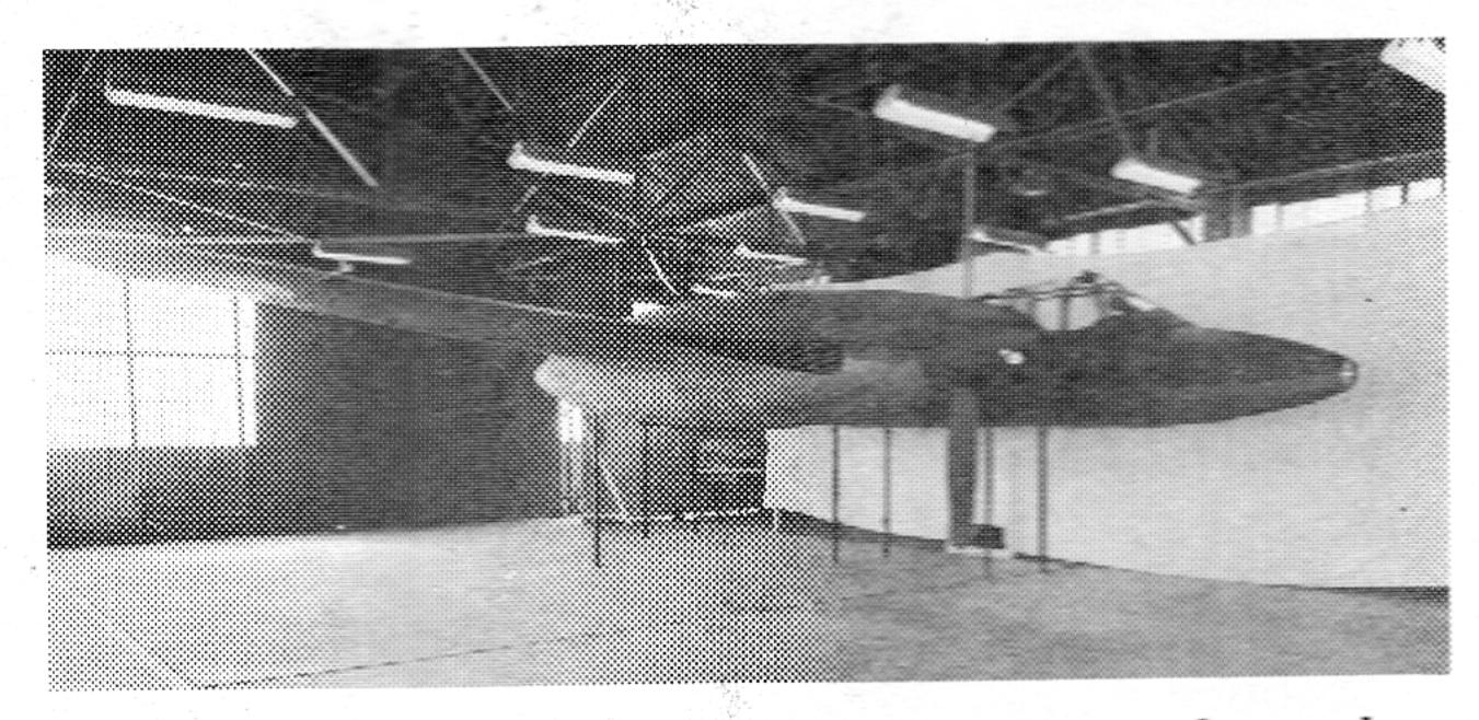
XP-67 mock-up shows unusual cooling duct inlet and two of six 37mm cannons.
