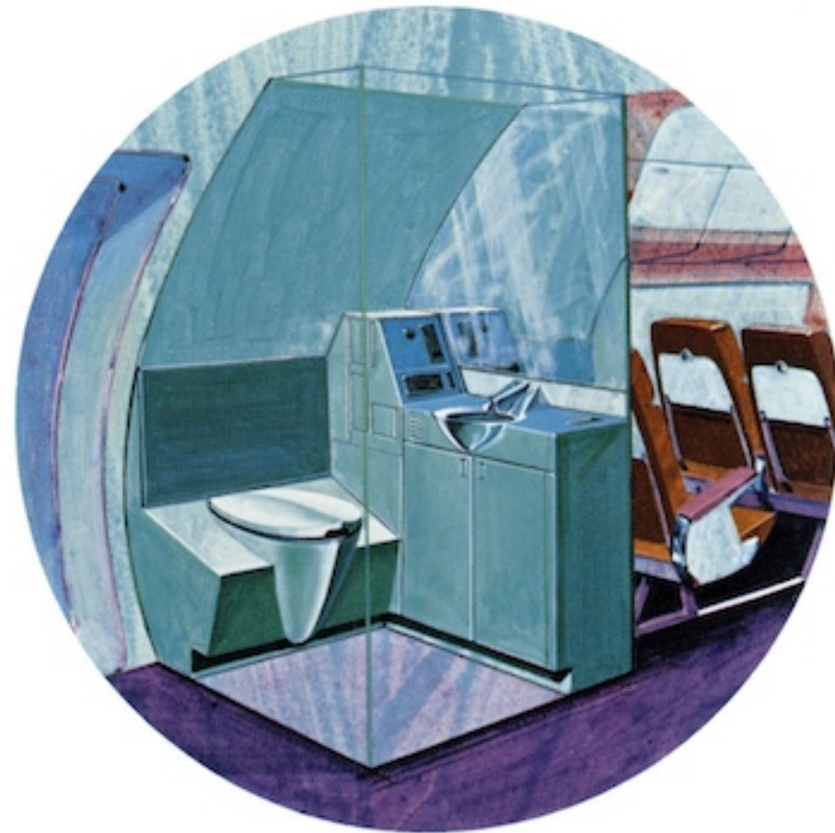
Modular lavatory service units permit optimum cabin arrangements for each airline.
