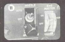
Variable-nozzle switch—**AUTO**. After lockup indicator light is extinguished.
