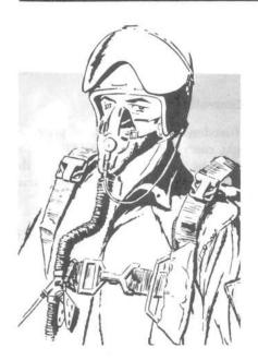
Attach oxygen mask hose (male connector) to parachute harness chest strap by wrapping mask connector tie-down strap underneath and up behind chest strap harness twice, then snapping.
