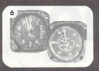
Engine speed—20% to 40% rpm windmilling. Restart at 40,000 feet or below.
