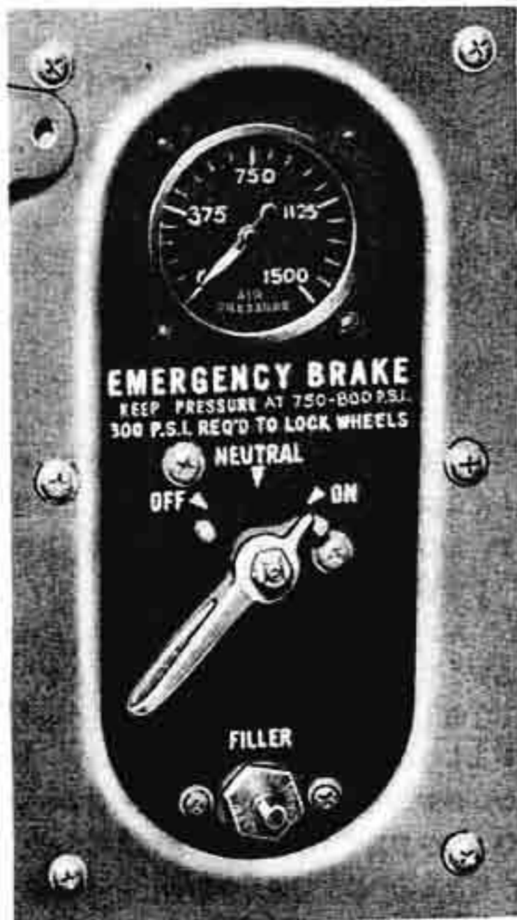
Figure 8 - Emergency Air Brake Control Panel
