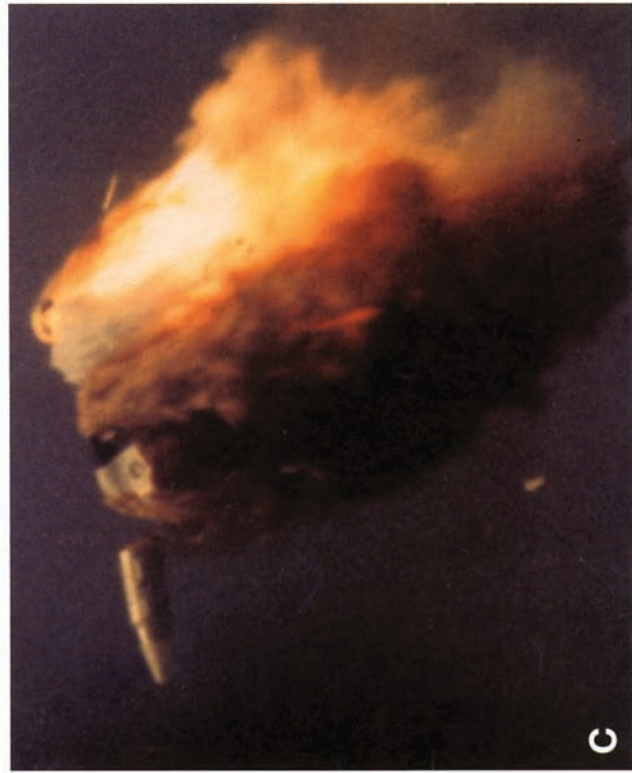
Figure CL.3. Titan II N-20 (61-2743) was launched from Cape Canaveral, Pad 16, on 29 May 1963. Stress corrosion in the Stage I thrust chamber fuel valve caused an engine compartment fire with resultant loss of engine control. A: rapid missile pitch over and interstage collapse prior to breakup; B: major airframe failure and Stage I premature separation destruct triggered; C: complete breakup of Stage I and separation of Stage II; D: Command destruct of Stage II. Courtesy of Darl Kemper.
