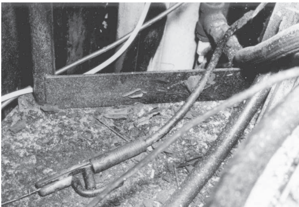
Figure 9.1a. The scene of the accident at Launch Complex 374-4, 308th SMW, Little Rock AFB, Arkansas. The welding rod as it was found by the investigators. The actual nick in the braided line in the right upper corner of the photograph is not visible. The silo wall is to the left and air-conditioning ductwork is just out of view to the right. Courtesy of the Air Force Historical Research Agency, Maxwell Air Force Base, Montgomery, Alabama.
