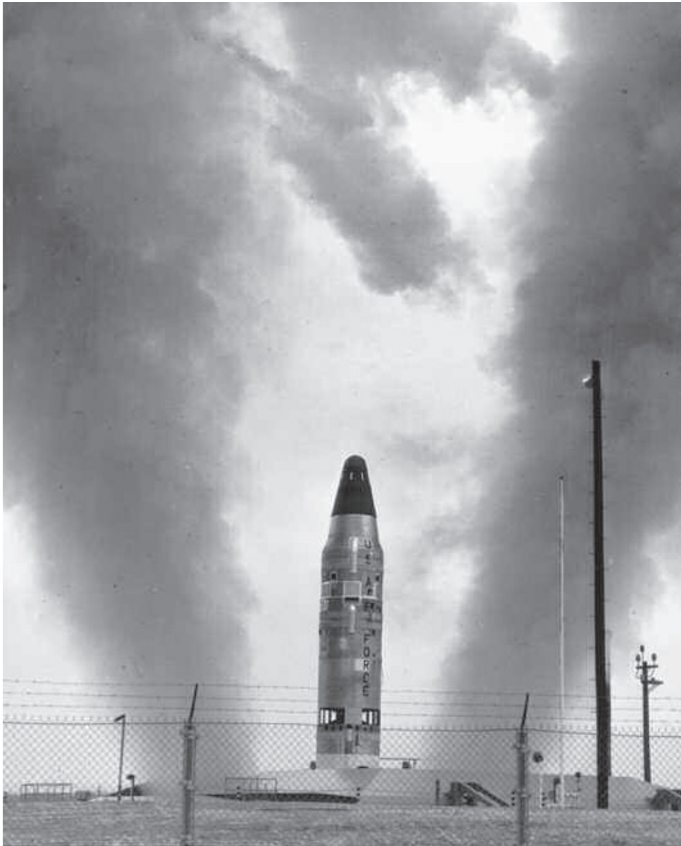
Figure 4.8a. Titan II N-7 (61-2730) lifts off from Launch Complex 395-C, Vandenberg AFB, 16 February 1963. This was the first in-silo launch in the Titan II program. Observers noted immediately that the missile was spinning at this point. Courtesy of F. Charlie Radaz.
