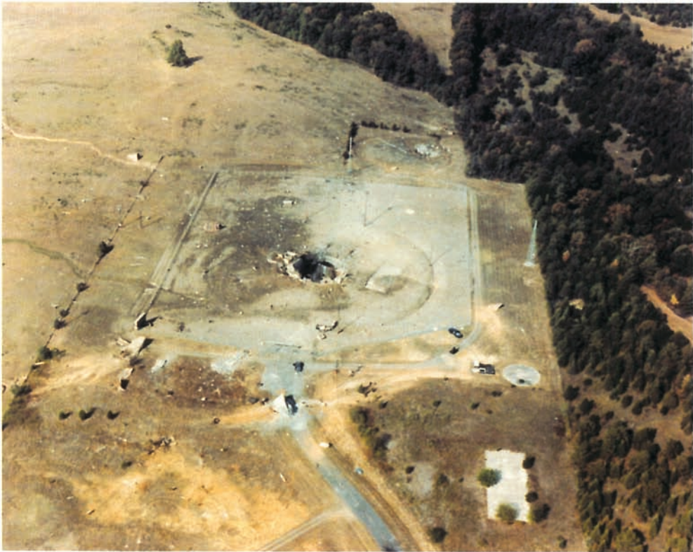
Figure CI.10. Aerial view of Launch Complex 374-7 looking southeast several days after the explosion. The 740-ton silo closure door is in the woods at the upper right of the photograph. The w-53 warhead was found in the ditch beside the road to the helicopter pad at the lower center of the photograph. Courtesy of Bob Eagle.
