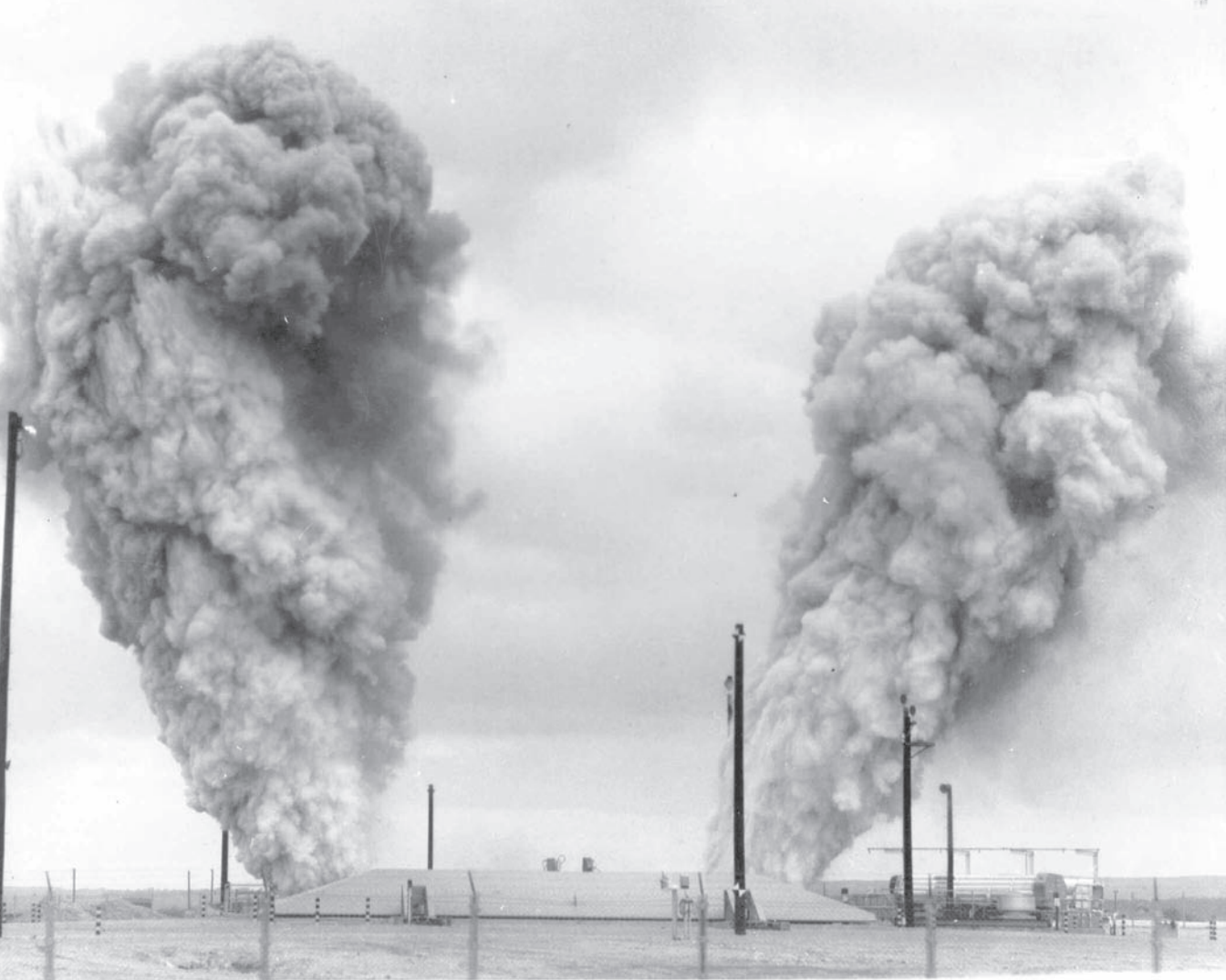
Figure 4.7. The captive fire test with Titan N-7 (61-2730) at Launch Complex 395-C, Vandenberg AFB, took place on 10 January 1963. While the exhaust from the Titan II is transparent in flight, the “oxidizer lead,” meaning that oxidizer reached the injector plate before the fuel, caused the initial exhaust, already opaque due to the steam generated by vaporizing the sound suppression deluge water, to be tinged with orange nitrogen tetroxide vapor. Courtesy of Rick Grossman.
