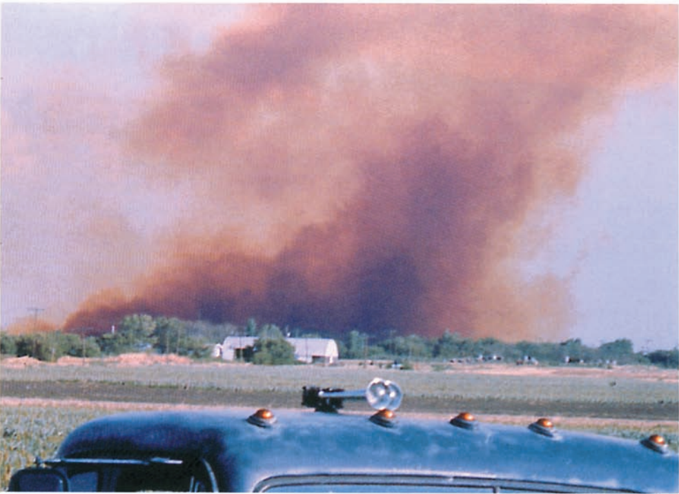
Figure CI.9. Addition of the first portion of 80,000 gallons of water to the nitrogen tetroxide accumulated in the flame deflector at Launch Complex 533-7 caused a violent reaction as the solution boiled and sent clouds of steam and nitrogen dioxide skyward. Courtesy of Mark Clark.
