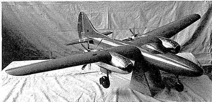
Powered wind-tunnel model of huge XP-71 fighter shows R-3350 nacelles, counter-rotating pusher propellers, bubble canopy, and 75mm cannon in nose. (Curtiss-Wright Photo)
