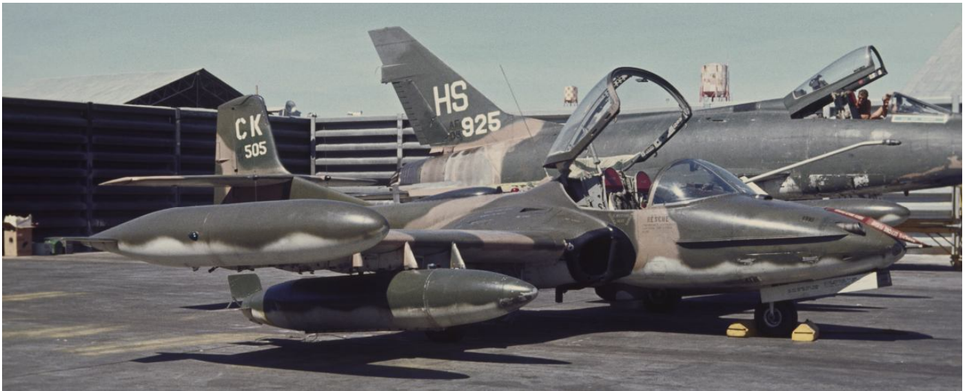
Another page with visitors at Cam Ranh Bay: sharing a revetment were F-100D 55-2925/HS of 308th TFS/31st TFW from Tuy Hoa AB and A-37A 67-14505/CK of 604th ACS/14th ACW. This Dragonfly was the third production aircraft and was based at Bien Hoa AB. The diminutive A-37As were based in Vietnam as an operational evaluation force under project 'Combat Dragon'. Experience gained with the type led to an improved version of the aircraft, the A-37B.
