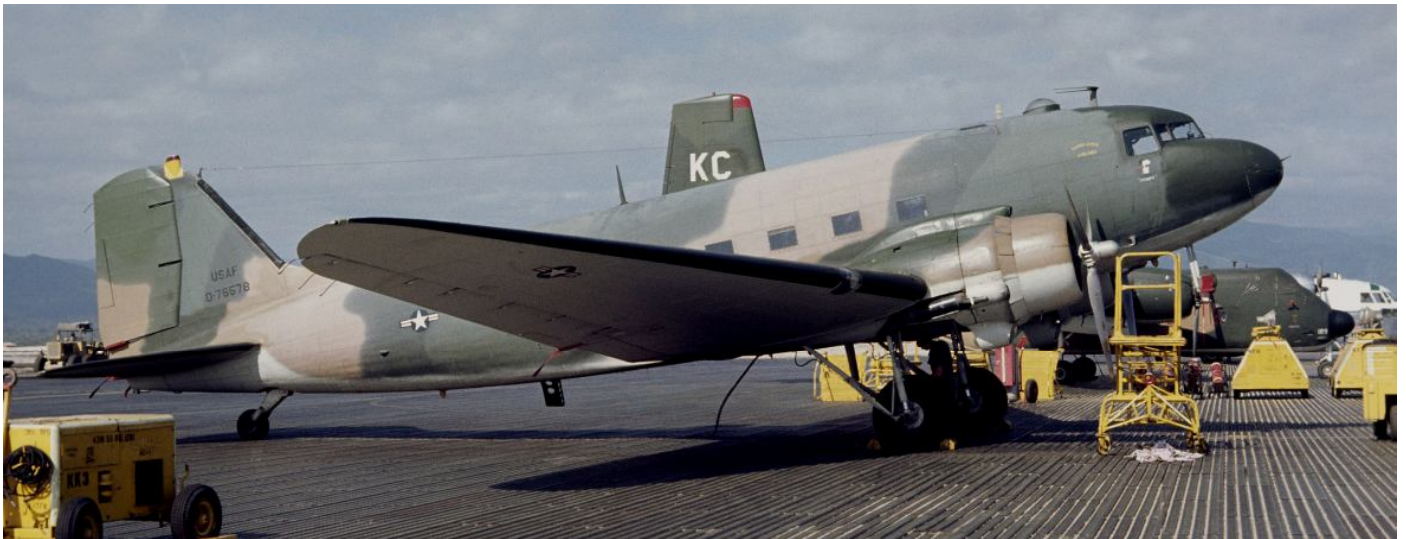
C-47s were still very much in use in Vietnam; the first gunships were converted 'Gooney Birds'. Seen here on the C-7 platform (note the aluminium planking) is C-47D 44-76578. The aircraft's unit remains unknown, but it does carry a small 'Snoopy' cartoon figure beneath the cockpit window.
