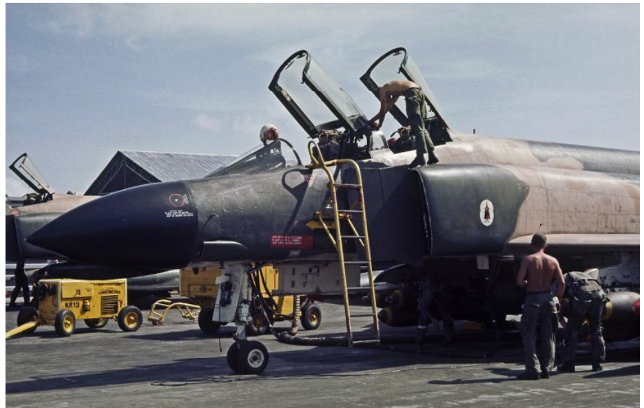
F-4C 63-7528/XC of 557th TFS/12th TFW being preflighted for another missions by its crew and groundcrew. Each wing station totes 3 1000 lb 'dumb' bombs. The crewmember on the right is putting the final touches to his G-suit while the one below the aircraft is checking the gun-pod.
