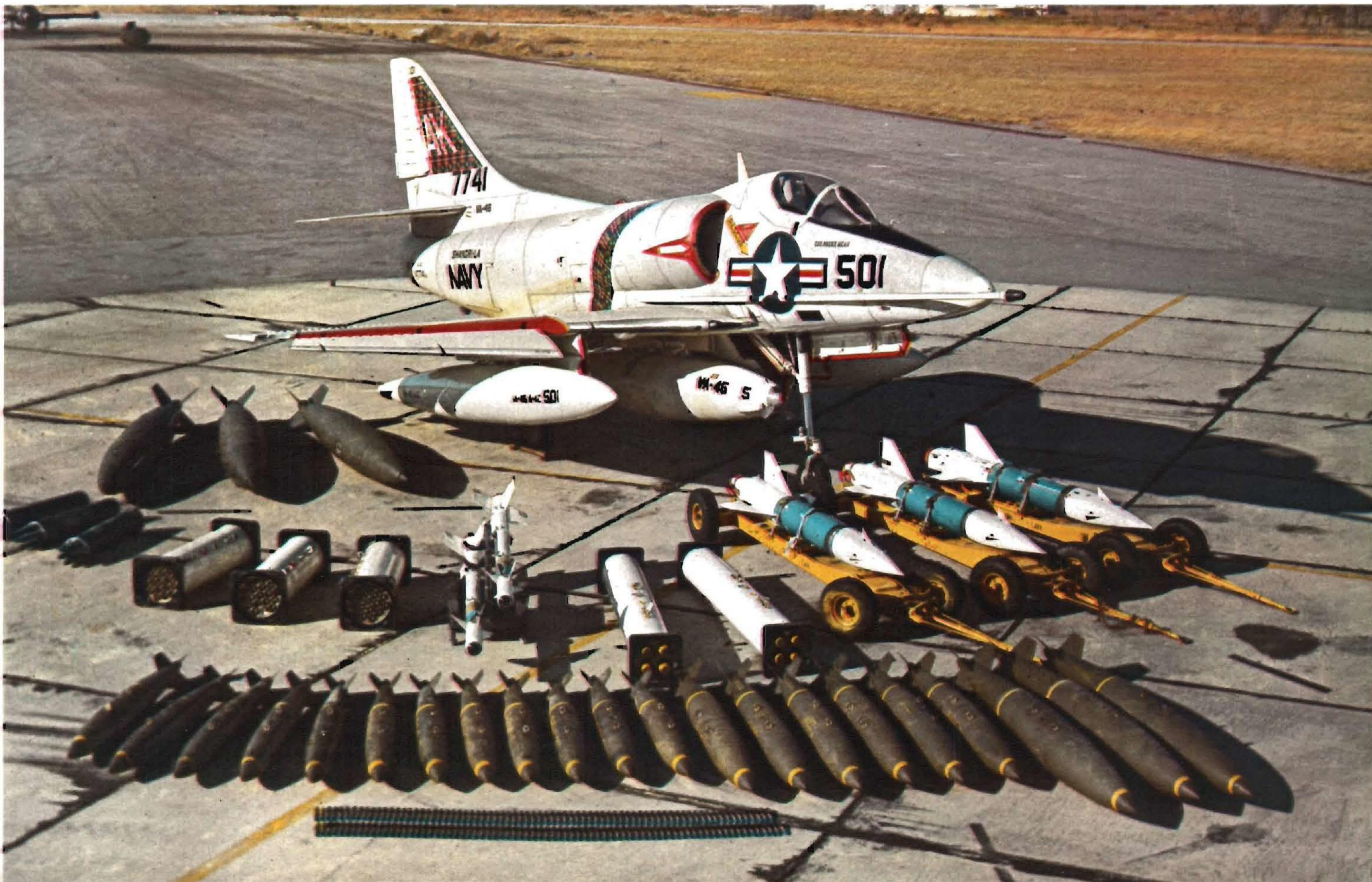
An A-4C from Squadron VA-36 (USS Shangri-La) poses with some of the ordnance which can be carried. In addition to the variety of bombs, this array includes ASM-7 Bullpup A and GAR-8 Sidewinder 1A missiles, LAU-3A/A 19-shot 2.75-in rocket packs, and LAU-10/A 4-shot 5-in Zuni rocket packs. The aircraft itself is carrying two fuel tanks and a Douglas-developed D704 in-flight refuelling store.
