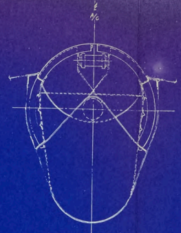
VIEW LOOKING AFT SHOWING PARACHUTE DOORS & BOX SCALE 1/4
