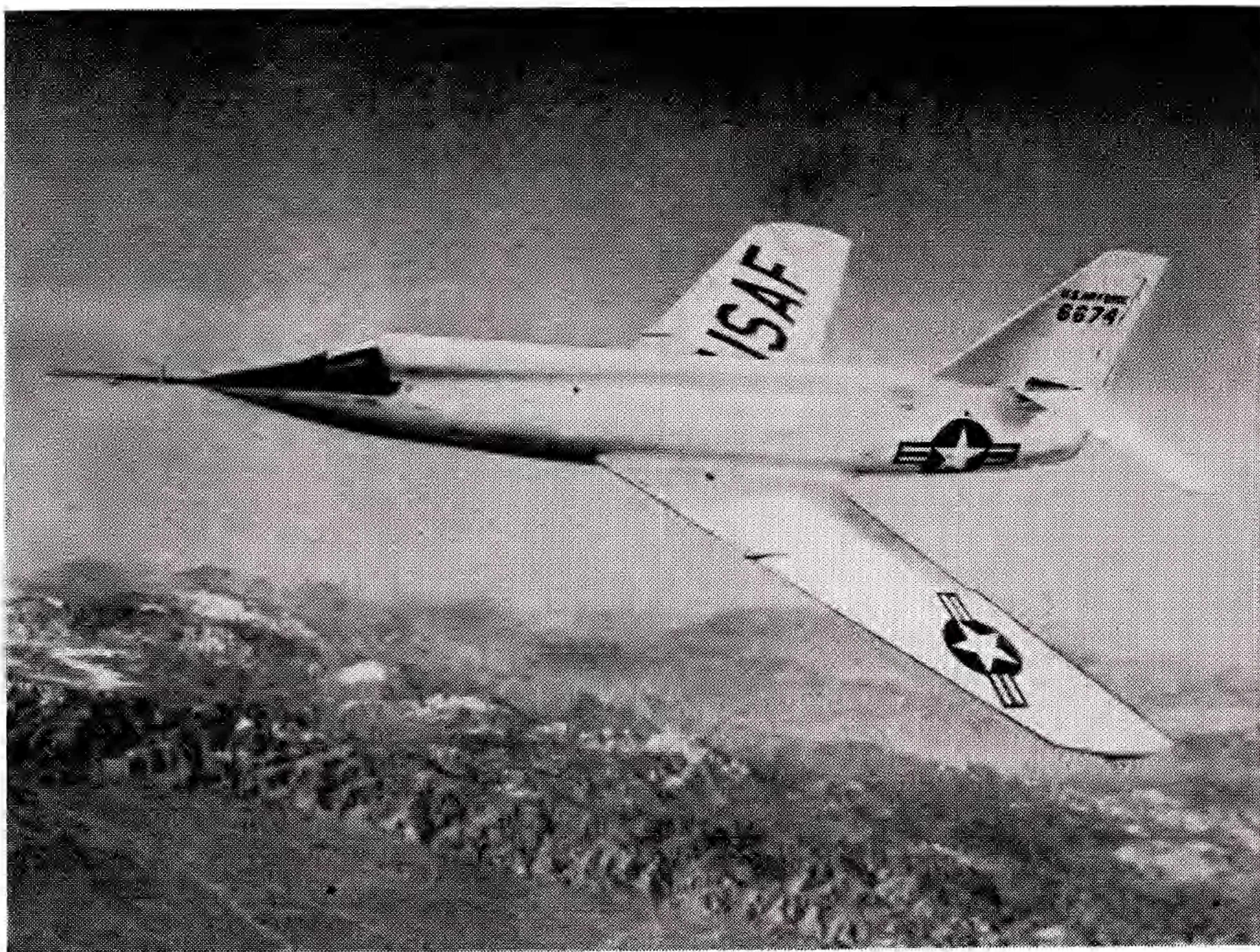
With a rocket engine that was able to develop almost as much power as a Navy cruiser, the Bell X-2 flies over the AF's test center at Edwards AFB, Calif.
