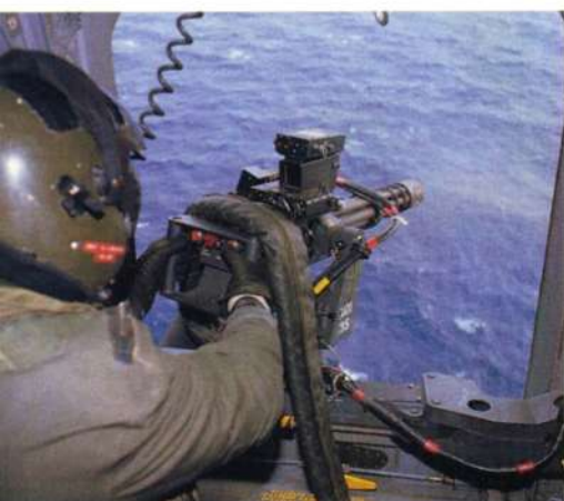
RAF crewmen and AGIs are qualified on both of the Chinook's weapons – the M60D and M134 Miniguns.
