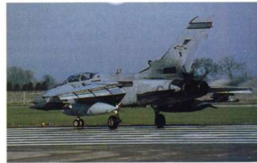
On test at Warton in 1995, F3 ZE161 carries a Towed Radar Decoy on the port outer pylon. Terry Senior
