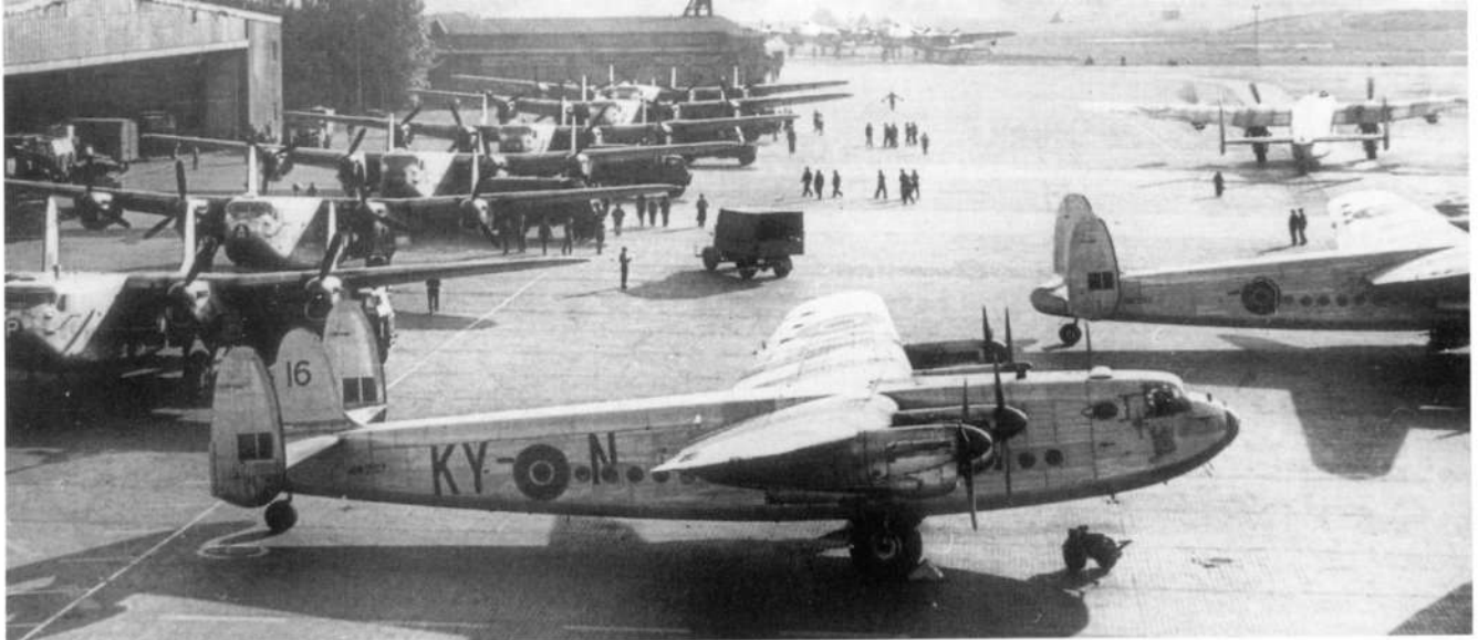
Avro Yorks on Gatow's apron. Note the airlift identity number applied to York 'KY-N', allowing easy recognition once on the ground. IWM
