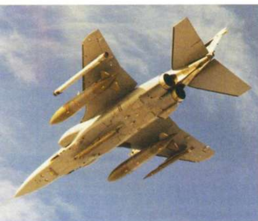
Jaguar 96 prototype XX738 with TIALD in co-operative designation fit.
