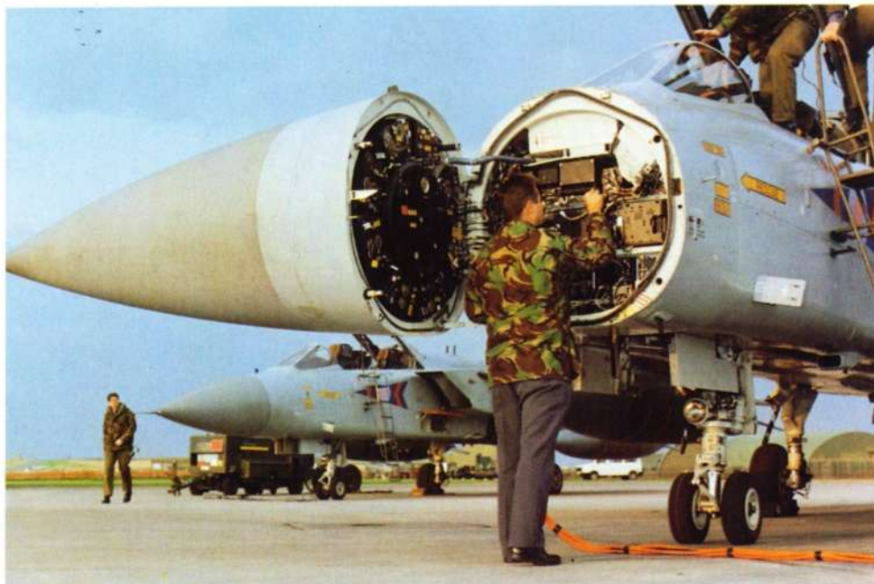
Upgrading the 'historically troublesome' Foxhunter radar has been a priority for the Tornado F3 improvement programme, and has given the F3 OEU considerable trials work.
