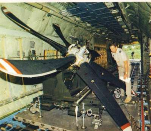
Chief Tech Paul Bradshaw of the AMDS Project Team checks the fit of a Dowty six-blade composite propeller on its transportation dolly in the C-130J's cargo compartment.
