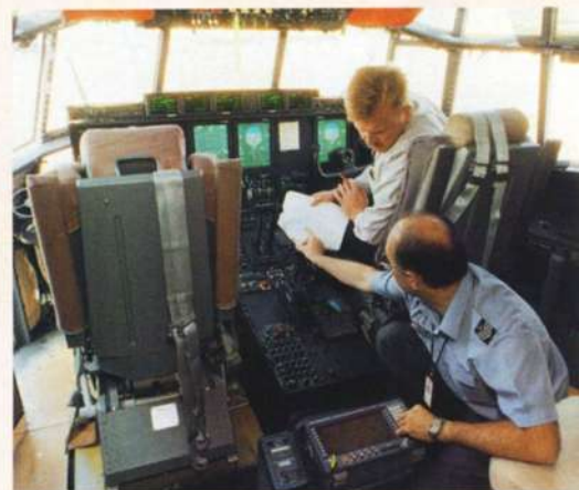
The RAF Team and Lockheed Martin engineers have worked closely together to develop the C-130J's fault diagnostic procedures; here Chief Tech Pete Looper is involved in validation of a maintenance procedure which uses the RAF's CMS33A test set.
