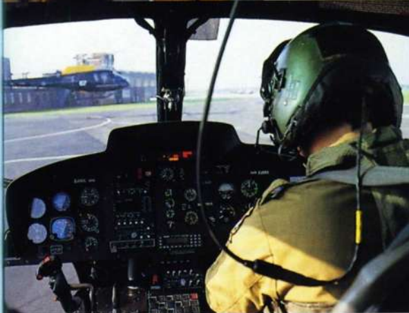
Above: The well laid-out cockpit of the Squirrel HT1, equipped with VOR, DME and GPS. Right: Squirrel HT1s can carry six people although three or four is normal for training sorties.
