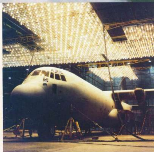
With engines running, the second RAF C-130J undergoes a heat soak in the McKinley Climatic Laboratory at Eglin AFB, Florida.
