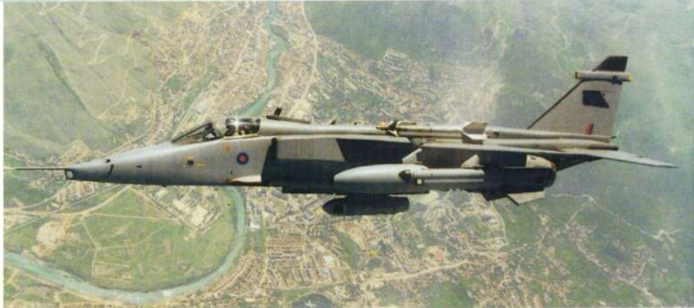
A Jaguar 96 of No 6 Squadron fitted with a Vinten VICON GP(1) recce pod over Mostar during a recent deployment in support of Operation Deny Flight. W Vinten Ltd via Jon Lake
