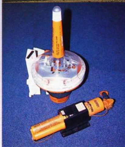
Left: The large object is a typical 406 marine beacon, activated on contact with water. The small unit is a search and rescue transponder (SART), which provides homing information when illuminated by a search radar. David Donald
