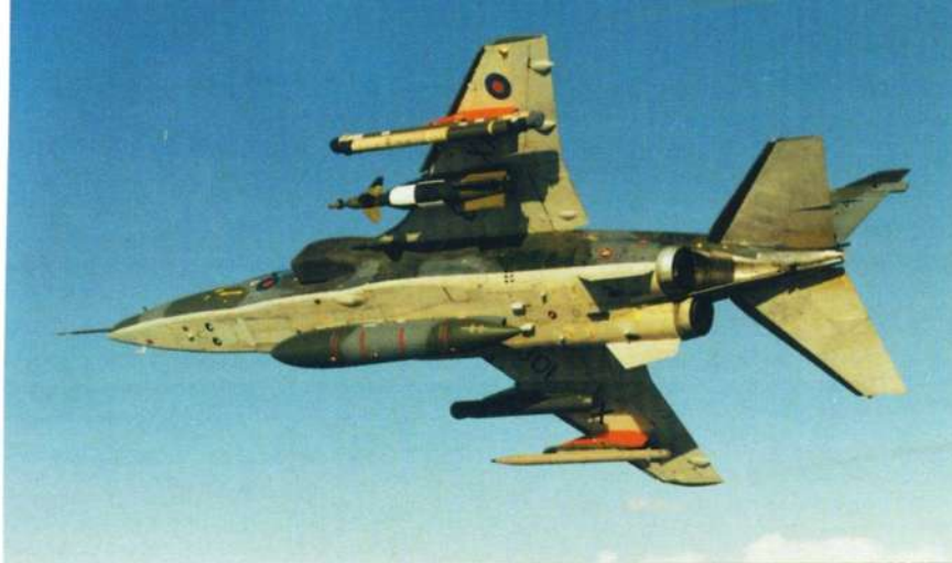
Above: Instrumented Jaguar XX108 is used for aerodynamic clearance of self designation fit.
