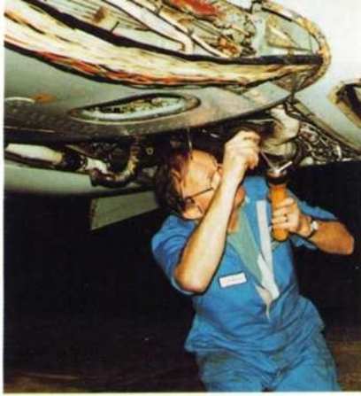
The civilian staff of Hunting Contract Services keep the Jetstream fleet flying. A 35-day Equal servicing is required every 600 flying hours.
