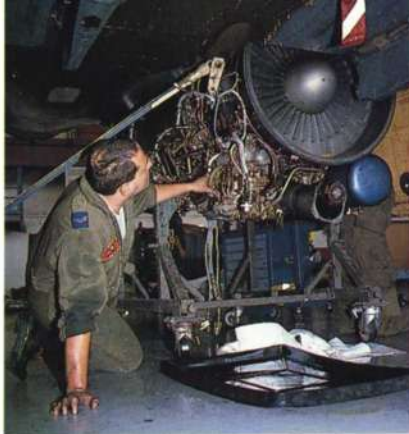
During maintenance, the Tornado's two RB199 engines are made accessible by lowering them onto a special trolley. Jeremy Flack/API
