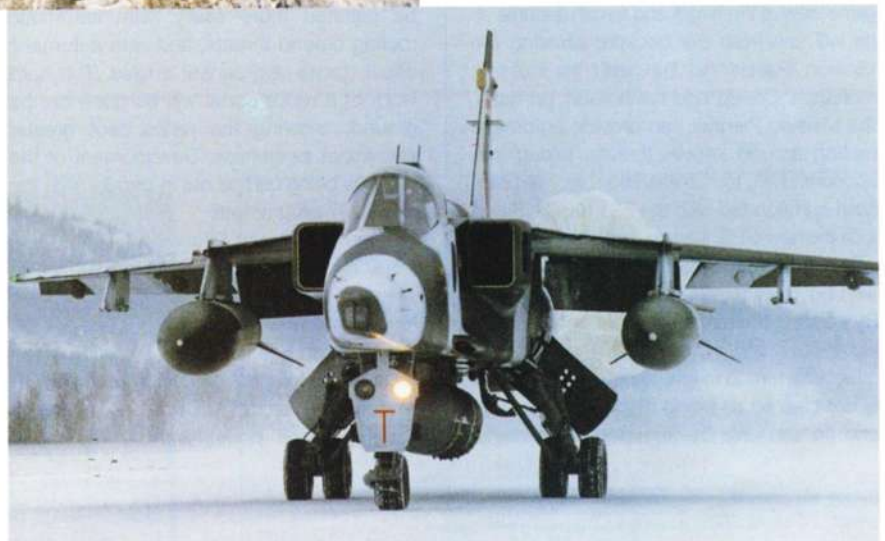
Suitably camouflaged during its deployment to Norway, this Jaguar carries a BAe reconnaissance pod on the centreline.
