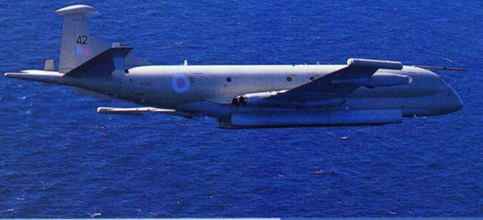
Above: A single Nimrod MR2 from the Kinloss Maritime Reconnaissance Wing is held on one-hour alert for SAR scrambles at all times. The aircraft carries pre-loaded, air-droppable ASR equipment in its weapons bay. Peter R March
