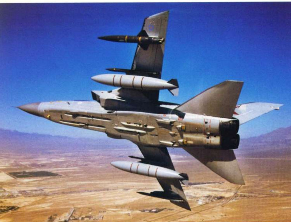
Photographed over the California desert landscape, F3 ZE968 carries a GEC-Marconi Aerial Towed Radar Decoy (TRD) on its re-activated outer wing pylon.
