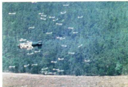
Bomblets separating from a BL755 canister as it nears the ground. Hunting
