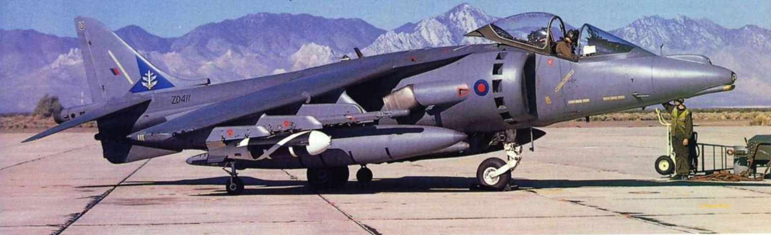
Carrying the Ballistic Test Vehicle (inert BL755) on its starboard pylon, Harrier GR7 ZD411 prepares to leave the ramp at China Lake. Chris Pocock
