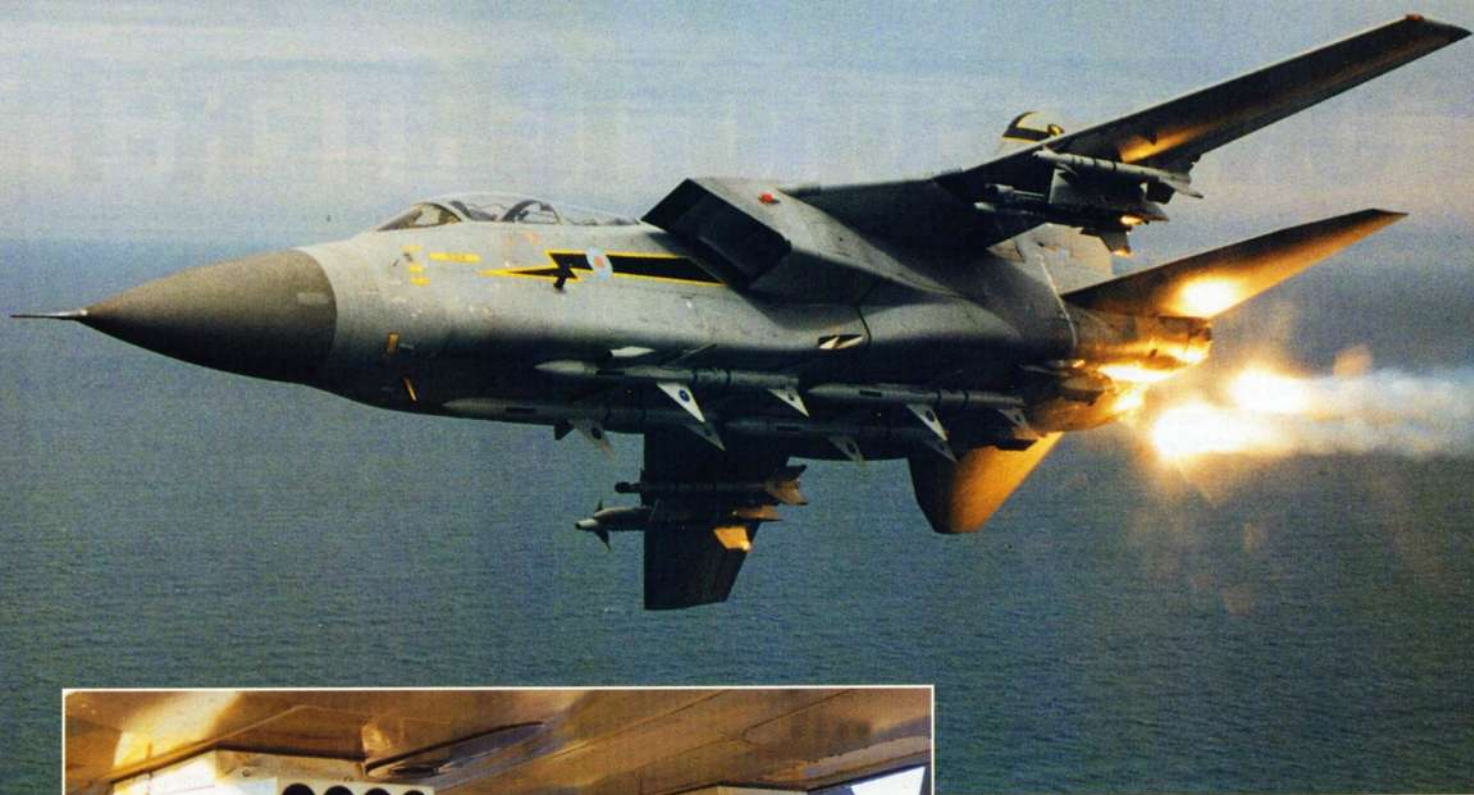
Recent improvements to the F3 have included fitting Vinten Vicon 78 flare dispensers (left), being demonstrated by a Tornado F3 of No 111 Squadron (above). Paul Jackson/Geoff Lee
