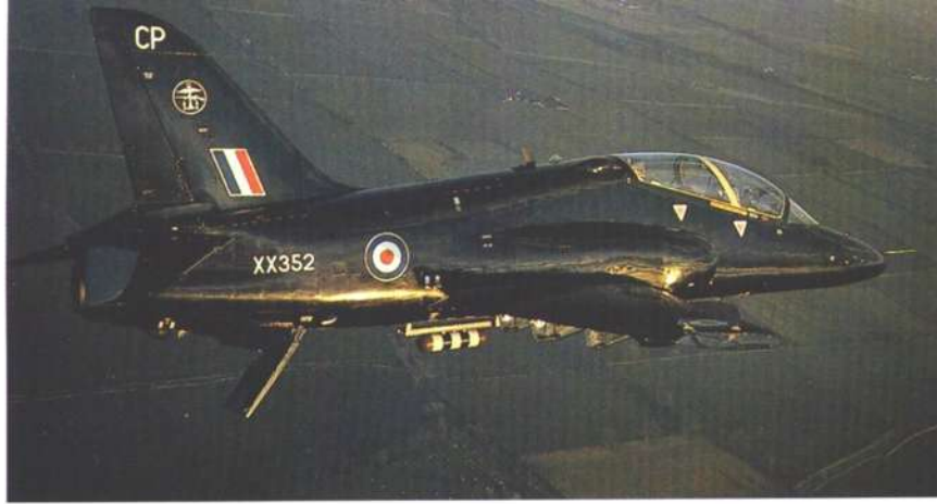
Left: Hawk T1A XX352 wearing the badge of the Joint Forward Air Controllers Training Support Unit (JFACTSU). Readily visible is the radar enhancement pod attached to the underside of the fuselage. Bob Archer
