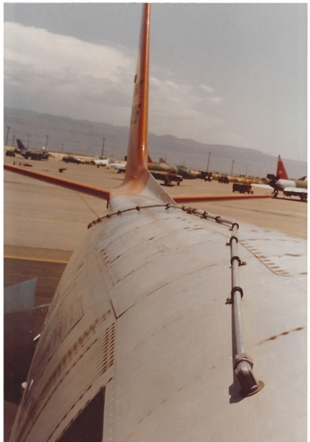
Above – Side view showing faded RCAF markings, oil line and later DFCS antenna mod.
