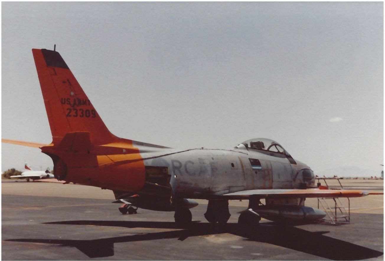
Above – Side view showing faded RCAF markings, oil line and later DFCS antenna mod.
