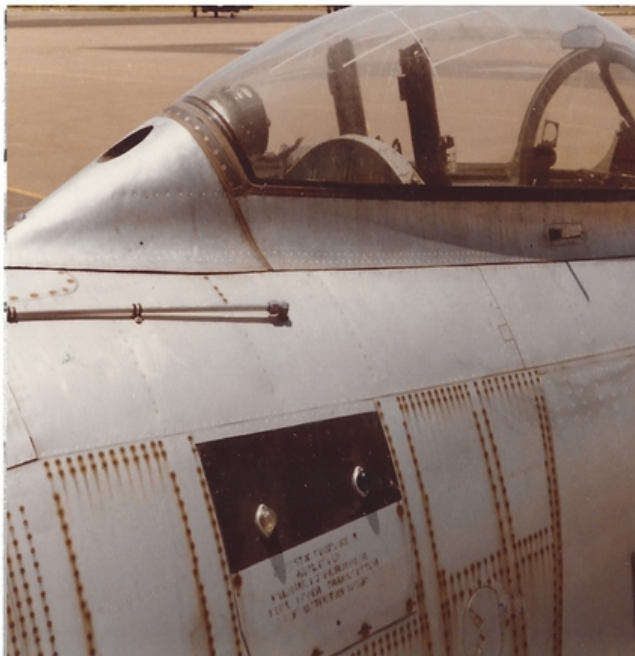
Below – View showing destruct panel and oil supply pipe going into fuselage.
