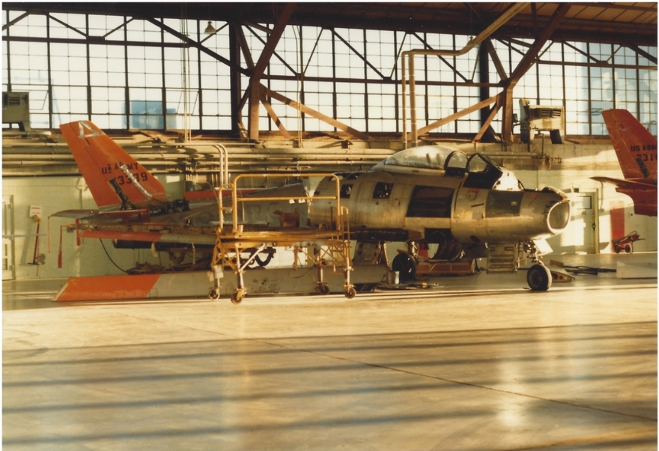
Above — Left hand view of Sabre (No. 23339) undergoing rebuild from damage caused by AIM-9 hit — January 1981.
