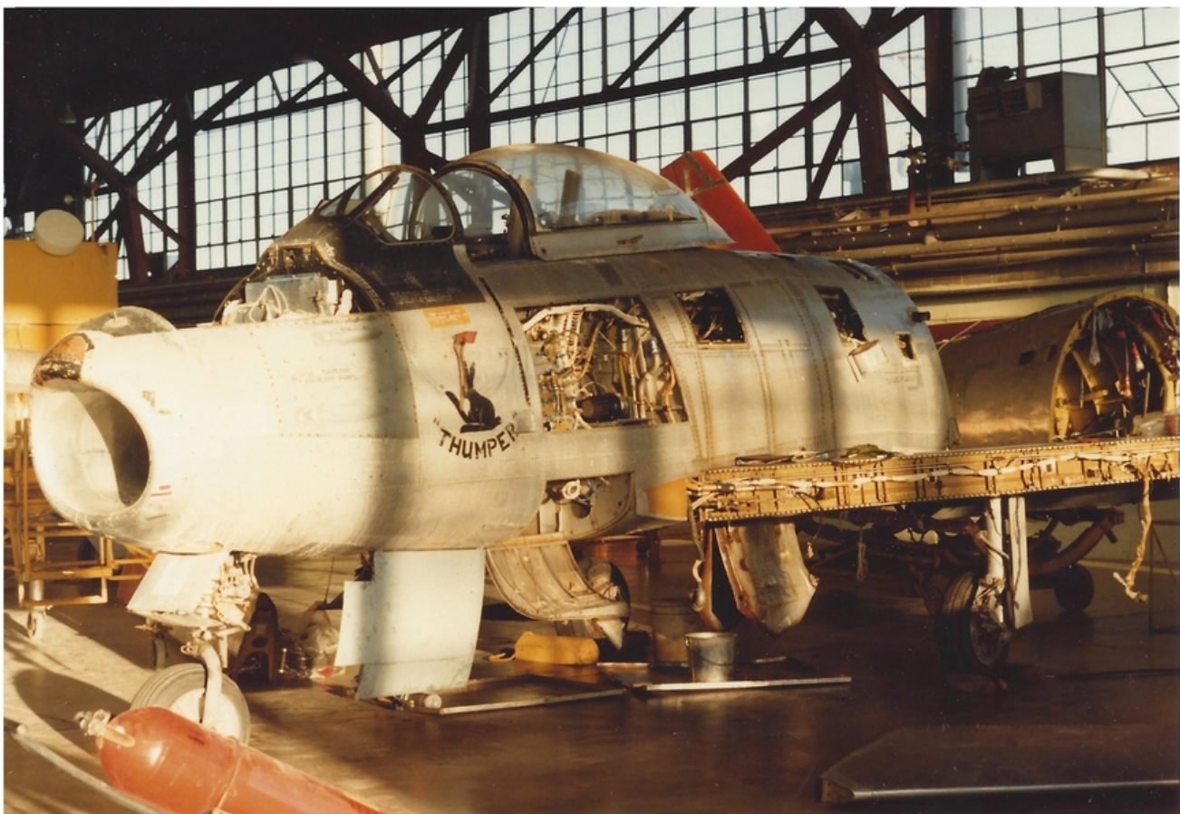
Below — Close-up of same aircraft, "Thumper". Note plugged guns and small scoring antenna on nose.
