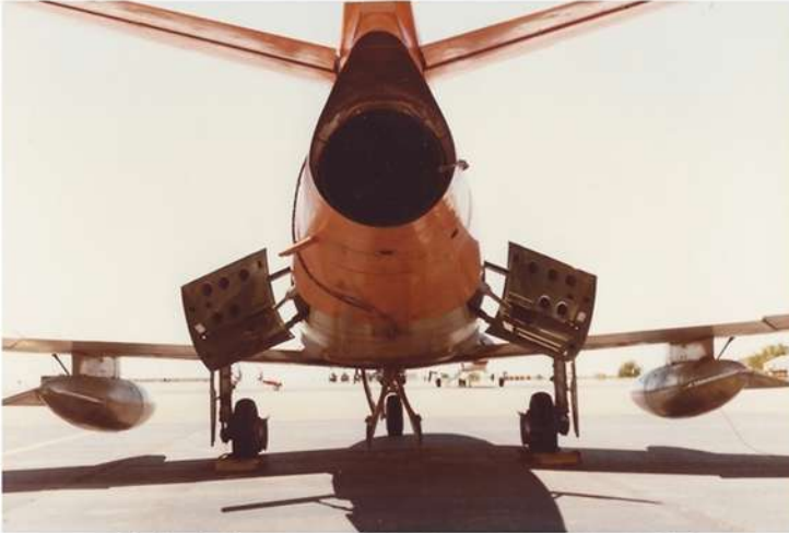
Aft view showing Vega antenna cable, oil line termination and open speed brakes.
