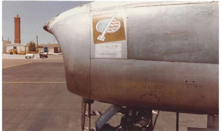
Good nose view showing plugged guns, 'beware of intake' warning (on some a/c) and Patriot missile logo.
