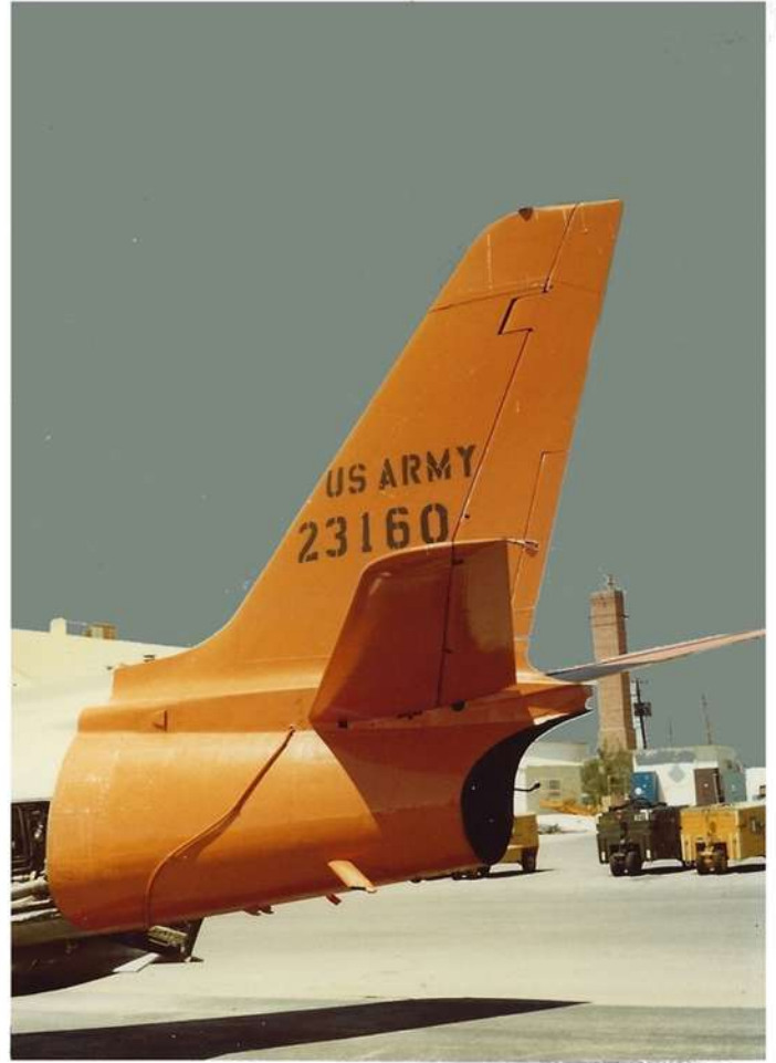
Close-up view of No. 23160, showing Vega system antenna cable and oil injection nozzle by tail pipe.
