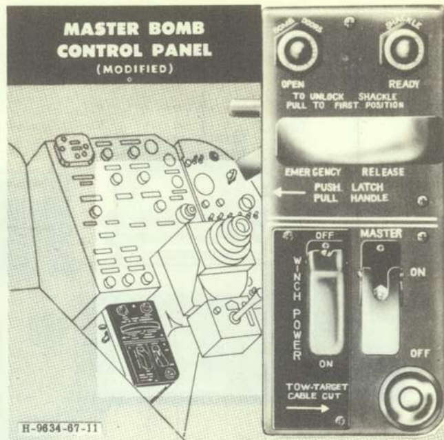
Figure 4-30. Master Bomb Control Panel (Modified)
