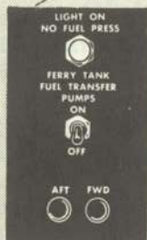
FERRY TANK CONTROL PANEL
