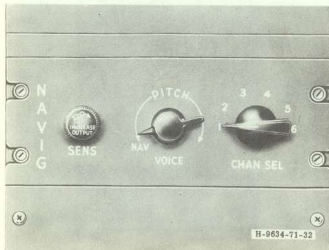
Figure 4-8. HF Control Panel (AN/ART-13 and AN/ARR-15)
