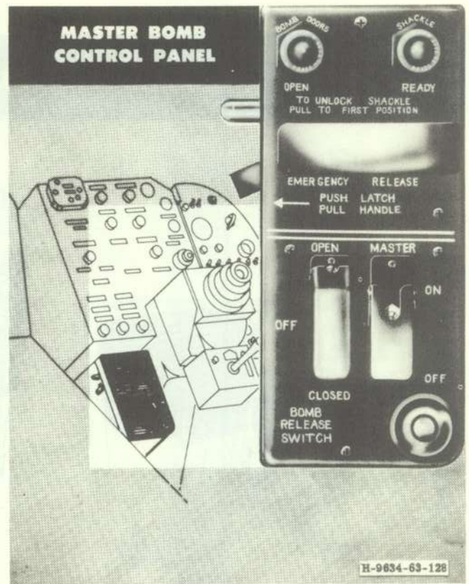
Figure 4-19. Master Bomb Control Panel
