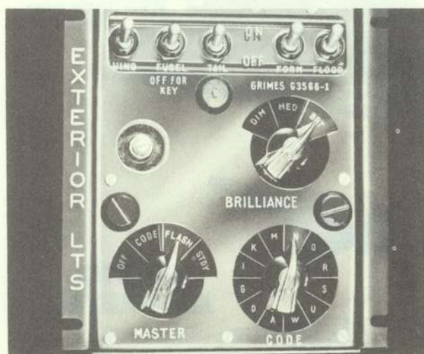
Figure 4-15. Exterior Lighting Control Panel
