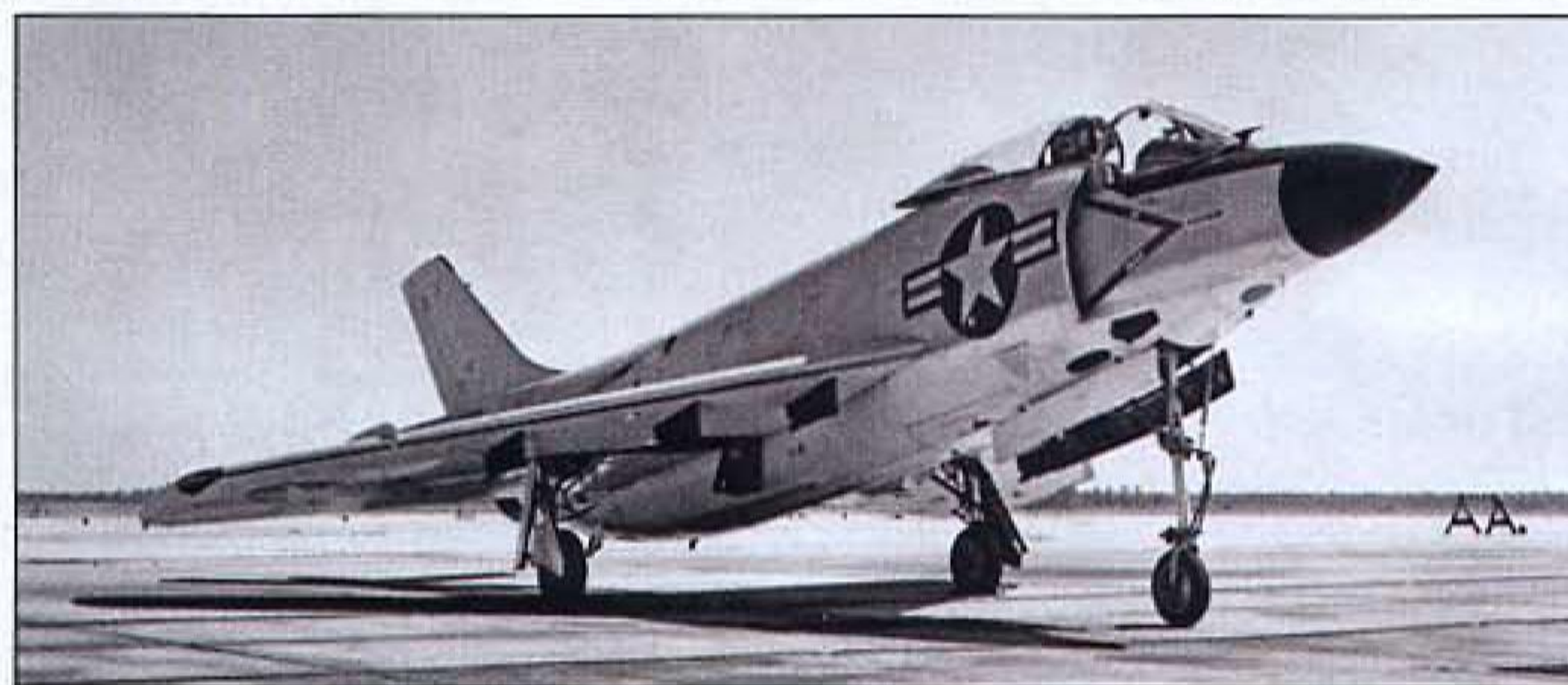
ABOVE This photograph of an early production F3H-2N shows well the unusual angle at which the type sat while on the ground. Note also the standard windscreen in place of the original one-piece.
