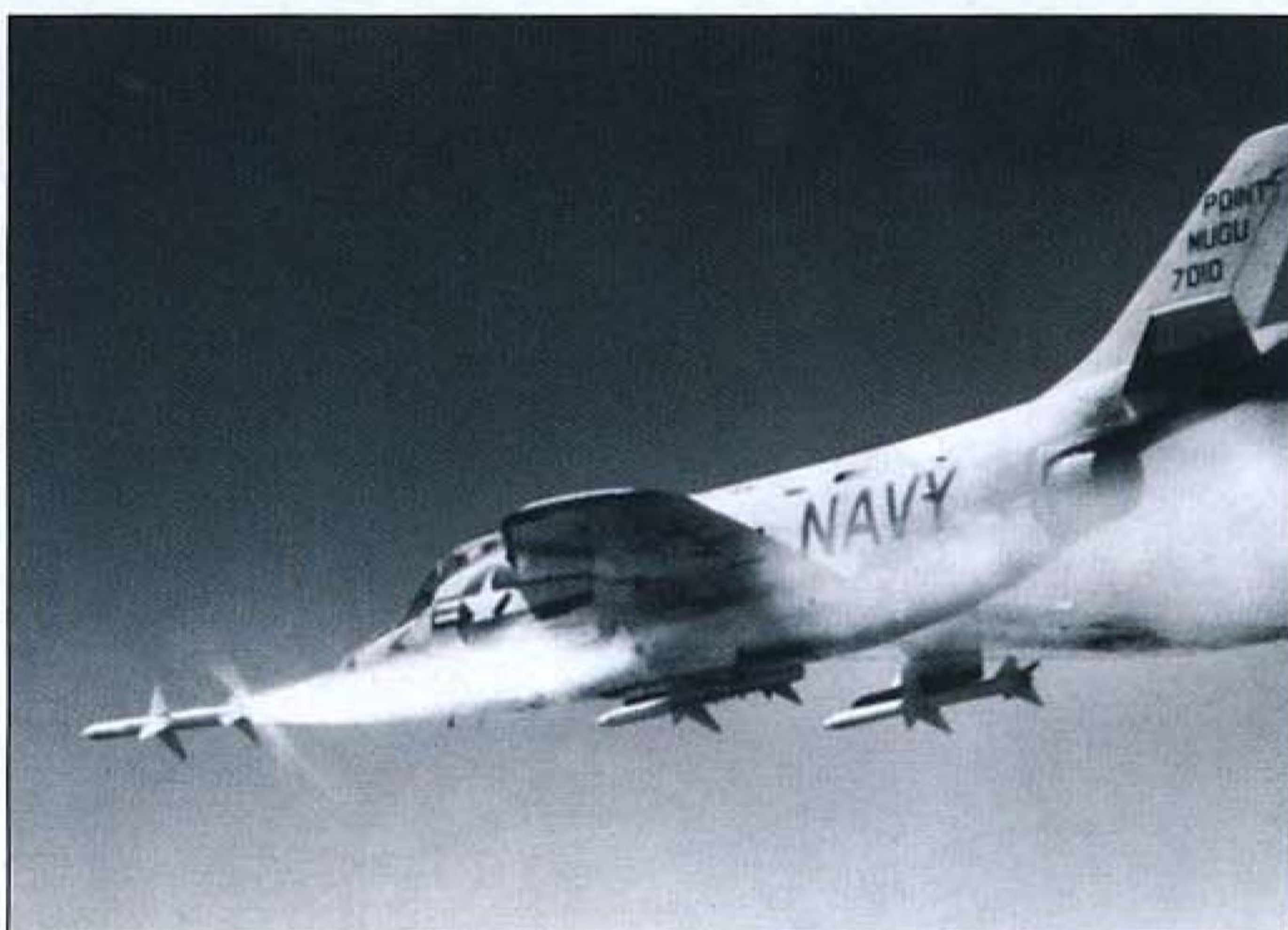
ABOVE An F3H-2M lets loose one of its complement of four radar-guided Sparrow air-to-air missiles during a series of tests at the Naval Missile Center at Point Mugu, California, in 1956.
