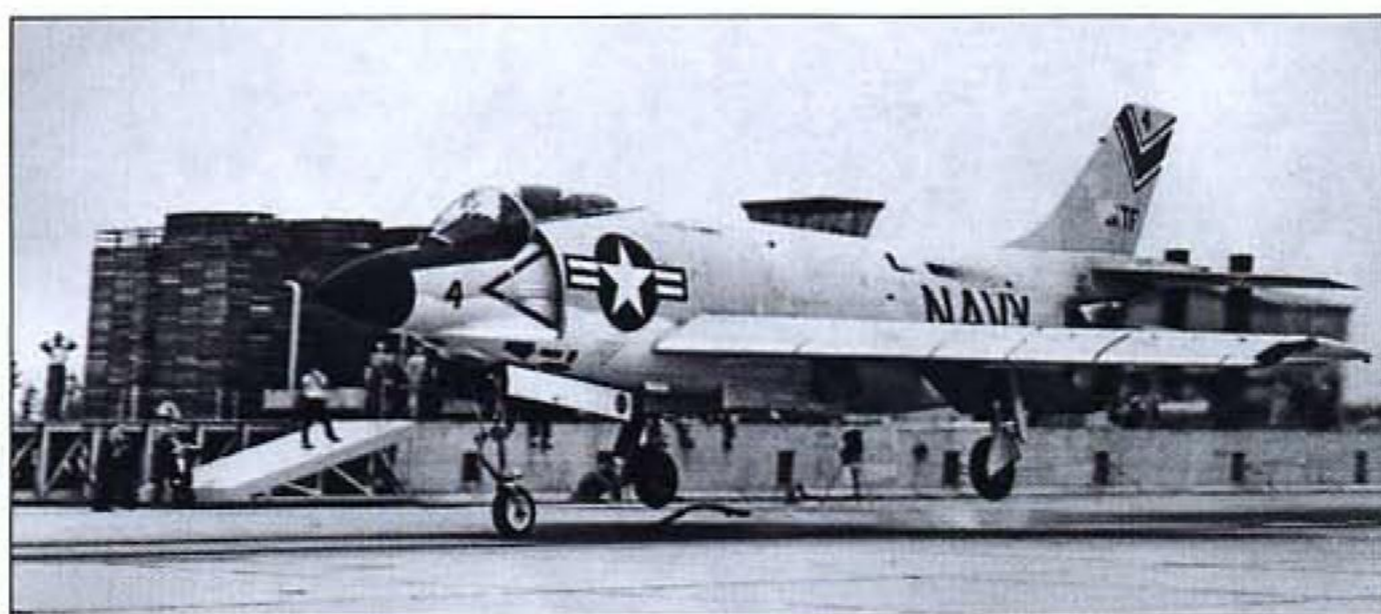
ABOVE An F3H-2 Demon is given a rocket-powered kick-off during tests at the Naval Air Test Facility at Lakehurst, New Jersey, in May 1959. Most aircraft catapults at the time were steam-powered.
