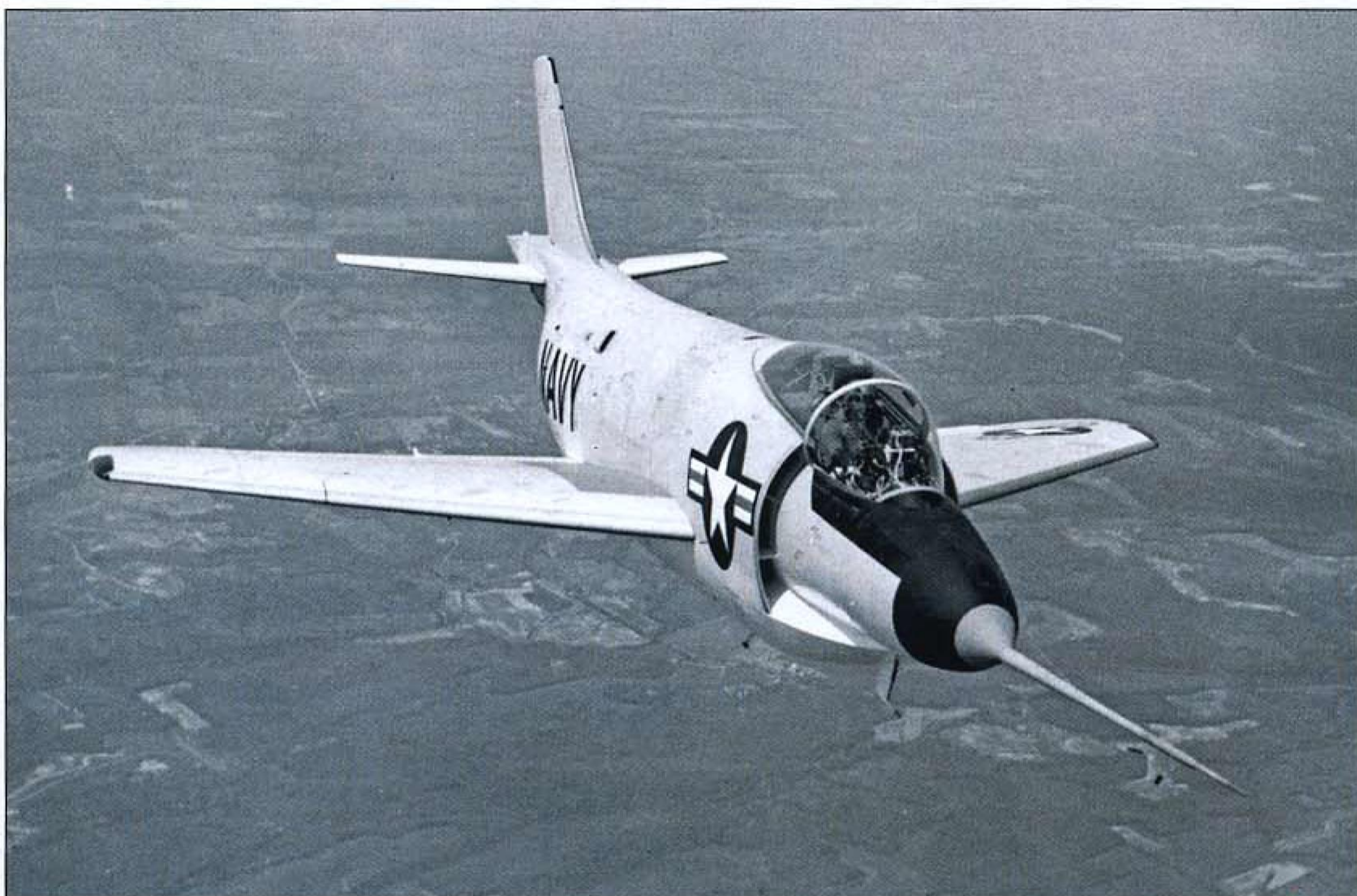
ABOVE Seen here on an early test flight in April 1955, BuAer 133549 was the first production F3H-2N, fitted with strengthened wings, improved radar and – crucially – the superior Allison J71 engine.
