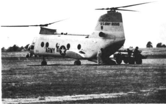
The HC-1B CHINOOK cargo transport has a maximum speed of 150 knots.
