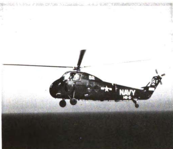
The HSS is used primarily for ASW search and attack missions. A Marine general transport version of the HSS is designated the HUS.
