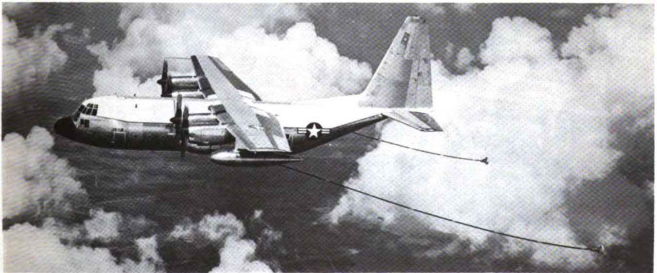
The GV-1 is the Marine version of the Air Force C-130 and is used as a refueling tanker.
