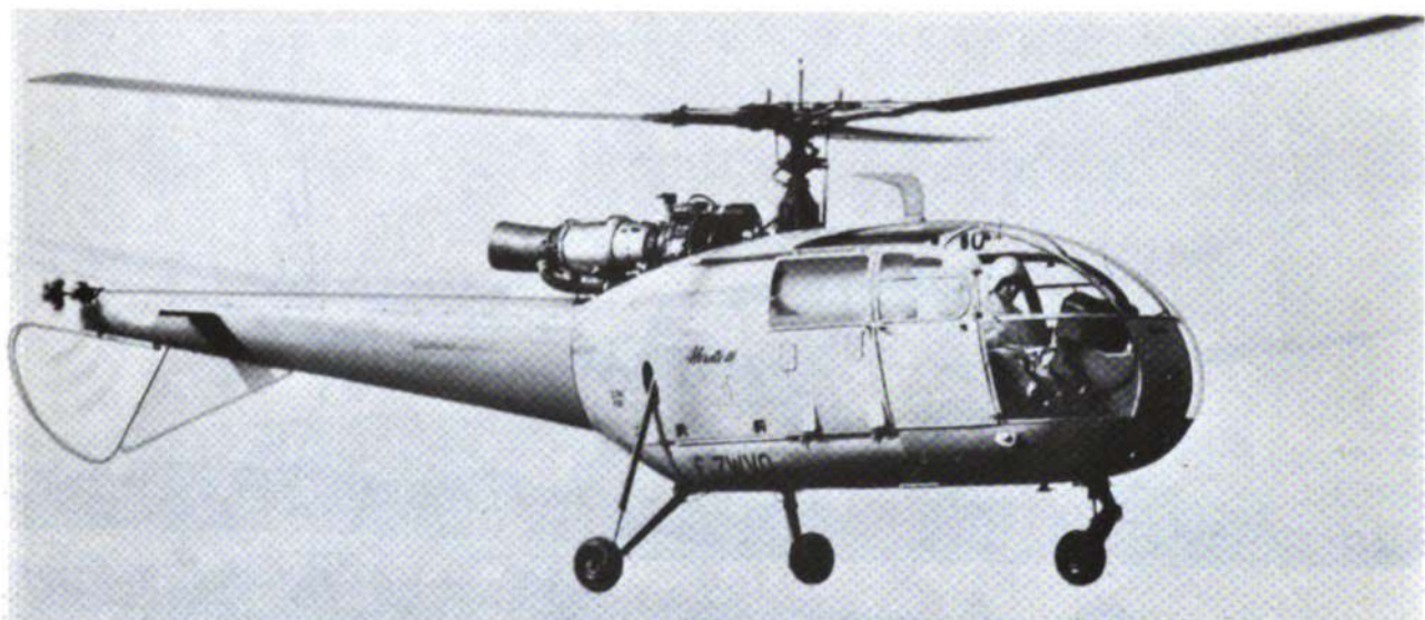
The S.E. 3160 ALOUETTE III is a multi-purpose helicopter developed from the Alouette II.
