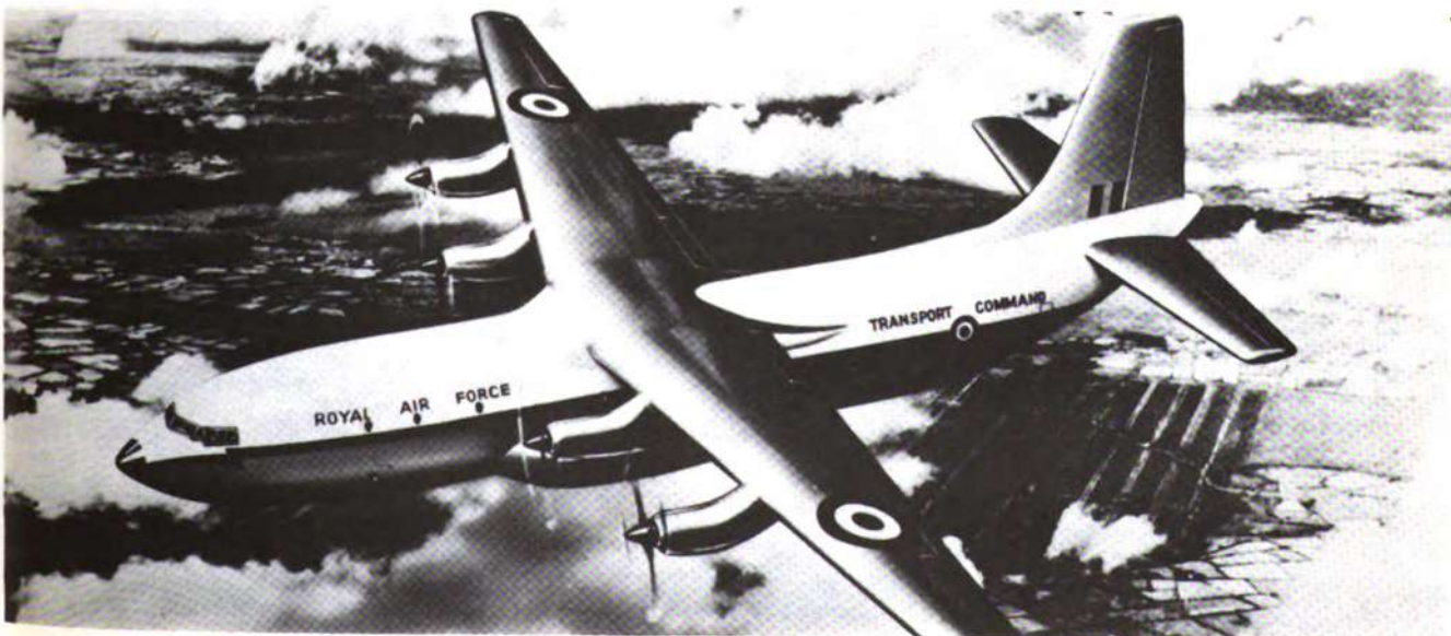
The BRITANNIC is distinguished by the high-mounted wing and long, slender engine nacelles.
