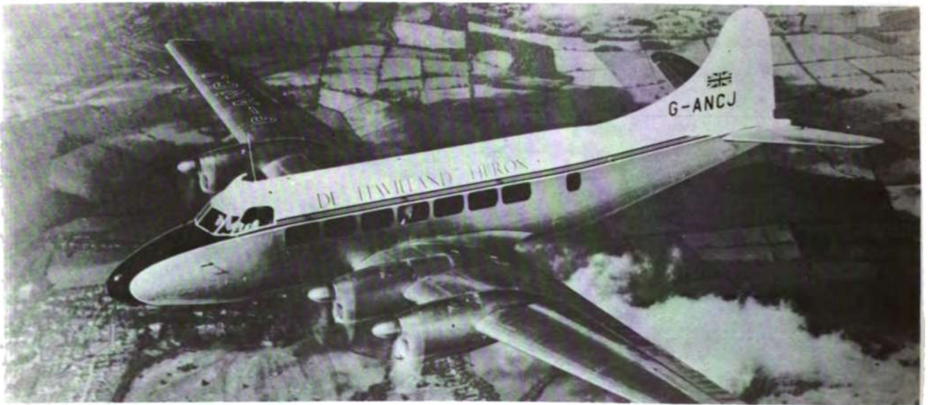
The HERON is a commercial airliner capable of carrying 14 to 17 passengers.
