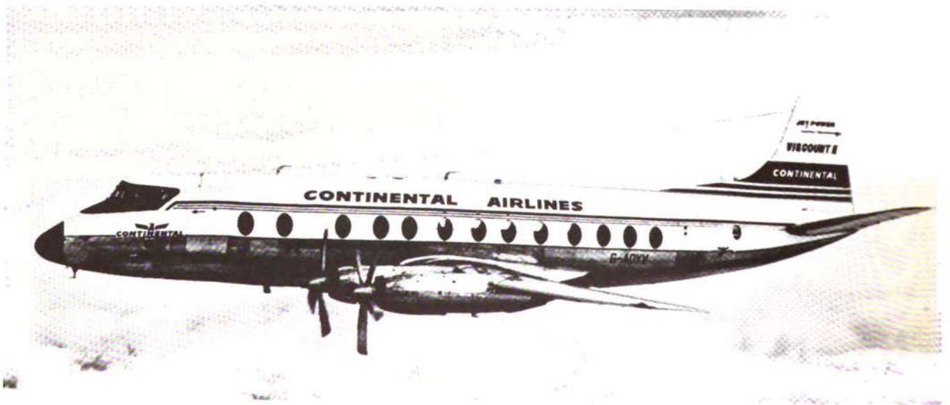
The Vickers VISCOUNT turboprop transport is used on U.S. airlines.
