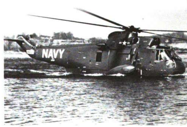
The HSS2 is an amphibious antisubmarine helicopter designed for all-weather operation.
