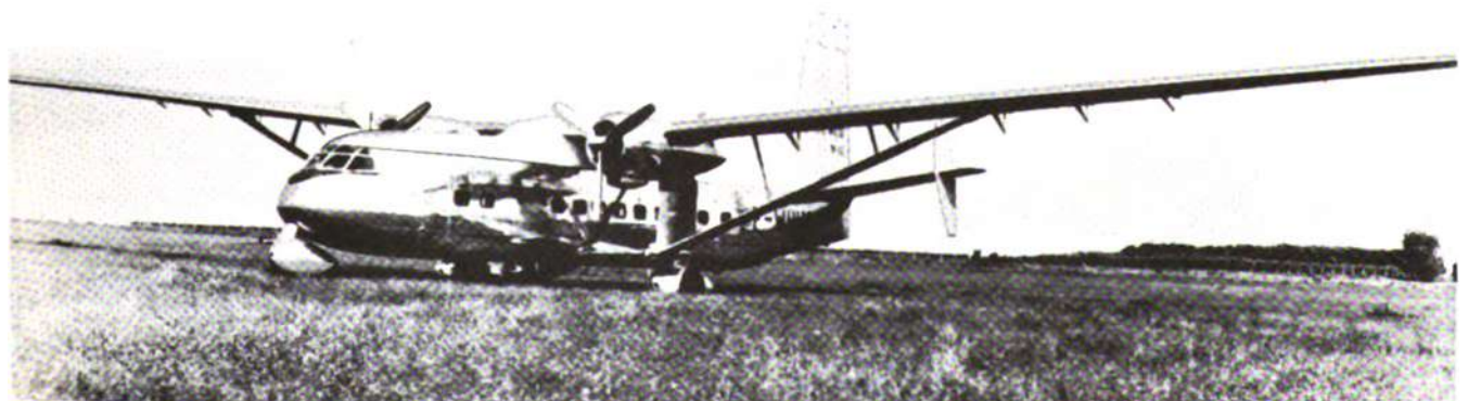
The H.D. 321 cargo transport features a high aspect wing ratio.
