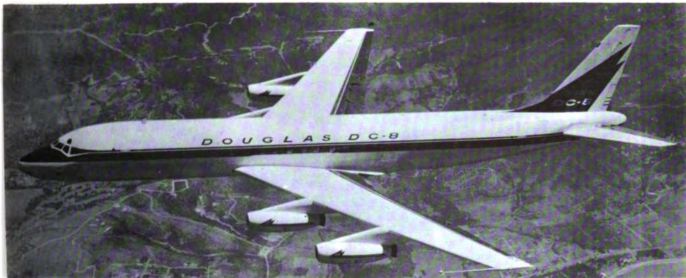
The Douglas DC-8 can accommodate from 118 to 176 passengers.
