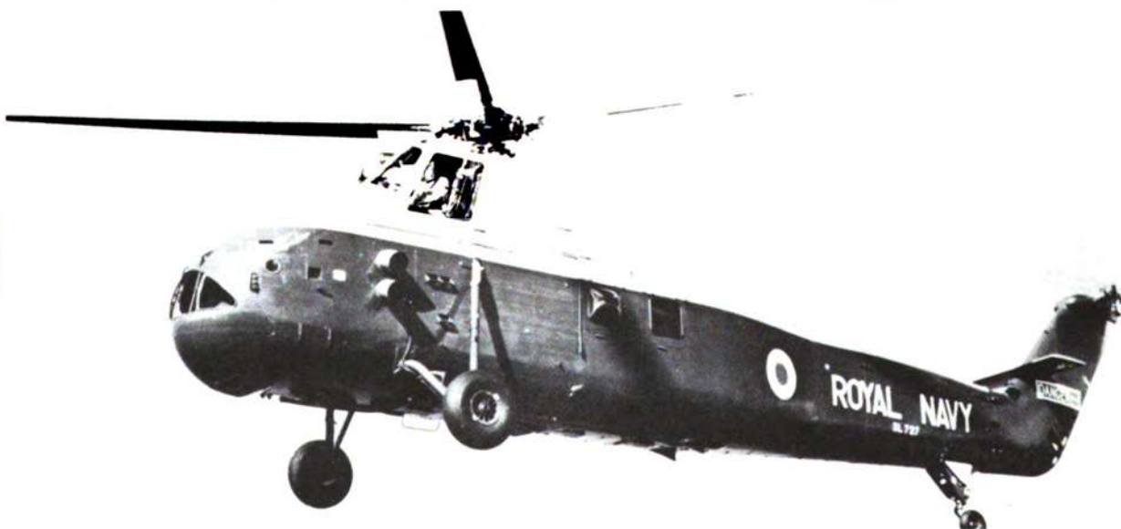
The WESSEX ASW helicopter is the Sikorsky S-58 built under British license.
