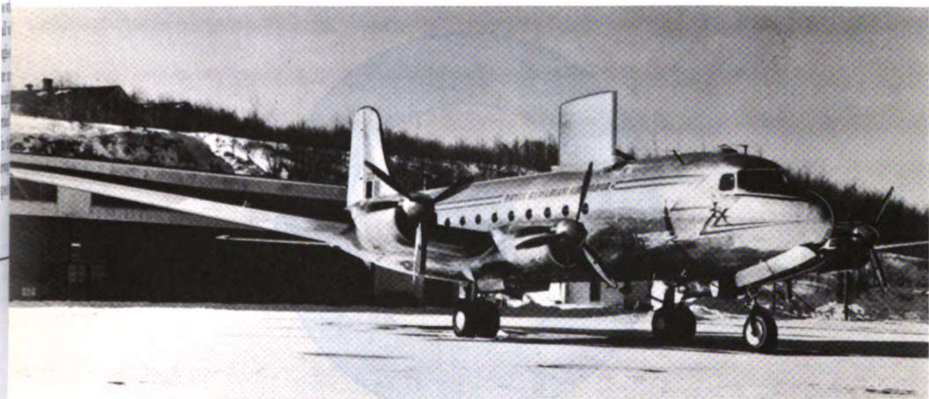
The NORTH STAR transport, relative of the DC-4/C-54, shown modified for airborne icing research.
