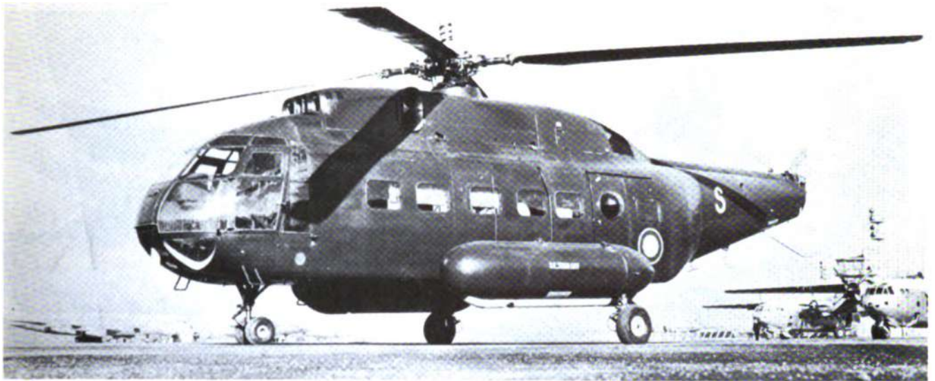
The S.E. 3200 FRELON is a 24-passenger heavy helicopter that also has an ASW capability.
