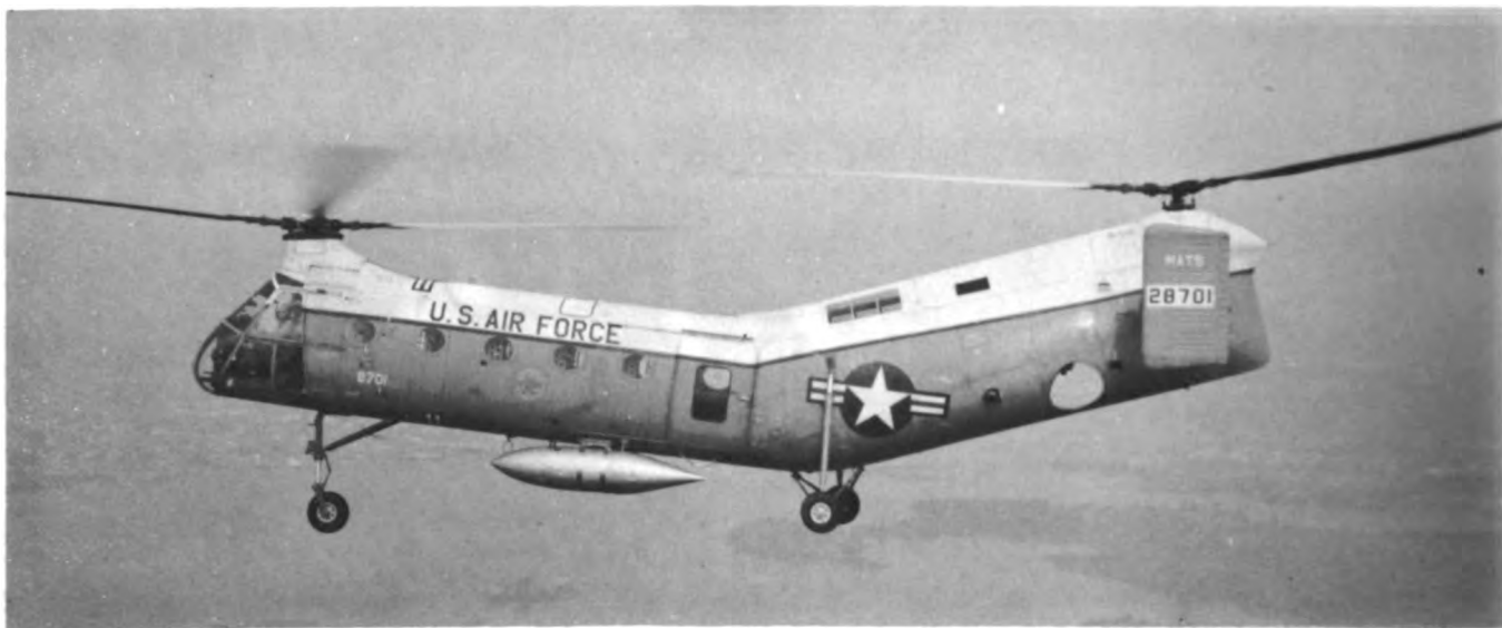
The H-21 RESCUER is capable of carrying 12 stretchers or 20 troops long distances.
