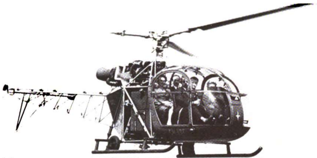
The S.E. 3131 ALOUETTE II was the world's first turbine-powered production helicopter.
