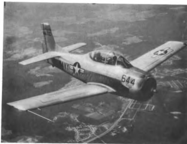
The T-28 high-performance, two-place, single-engine, propeller-driven trainer.
