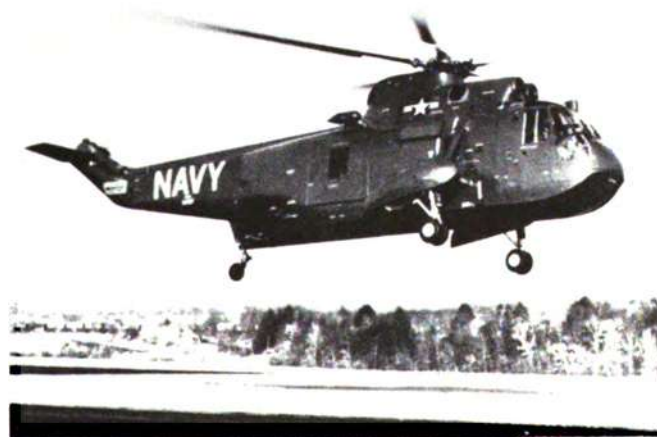
The HSS2 is an amphibious antisubmarine helicopter designed for all-weather operation.
