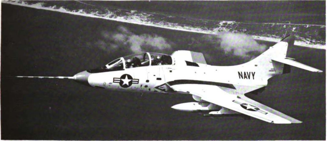
The F9F-8T COUGAR is a two-seat fighter-trainer version of the F9F-8 jet fighter.
