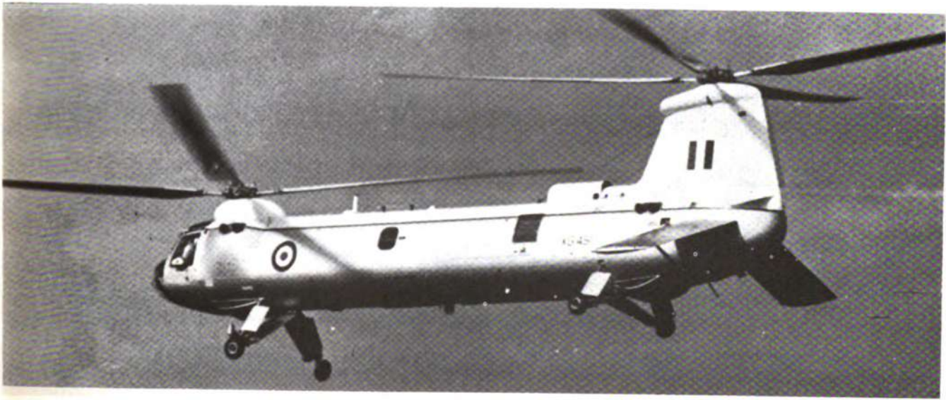
The BELVEDERE is a dual-rotor transport helicopter.
