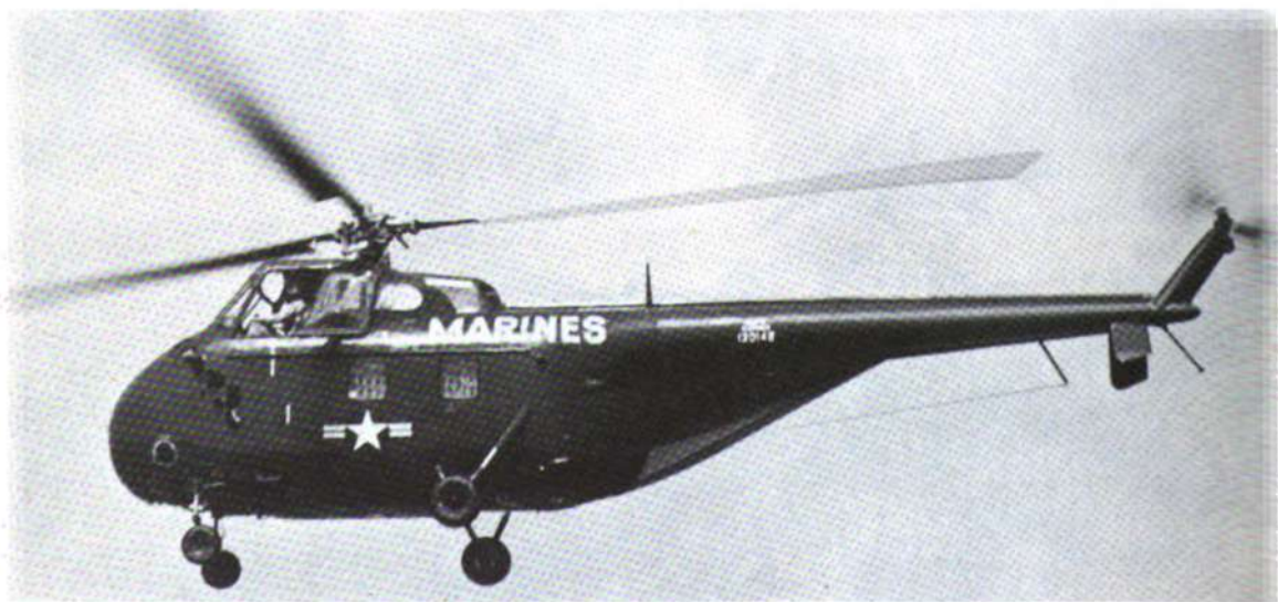
The HRS is the Marine assault transport version of the HO4S.
