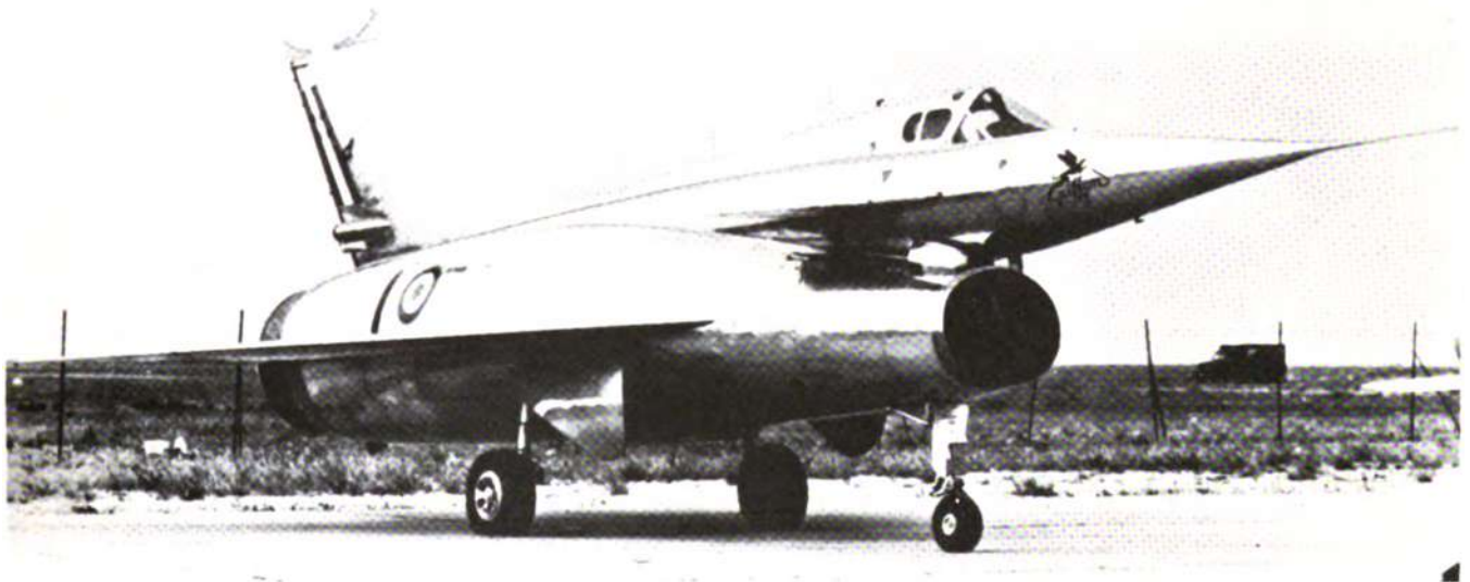
The Nord 1500 GRIFFON II experimental aircraft, designed to test a combination turbojet-ramjet propulsion system.
