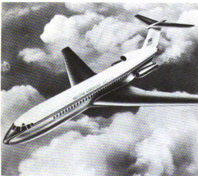
The TRIDENT (D.H. 121) is a three-jet, short-haul transport.
