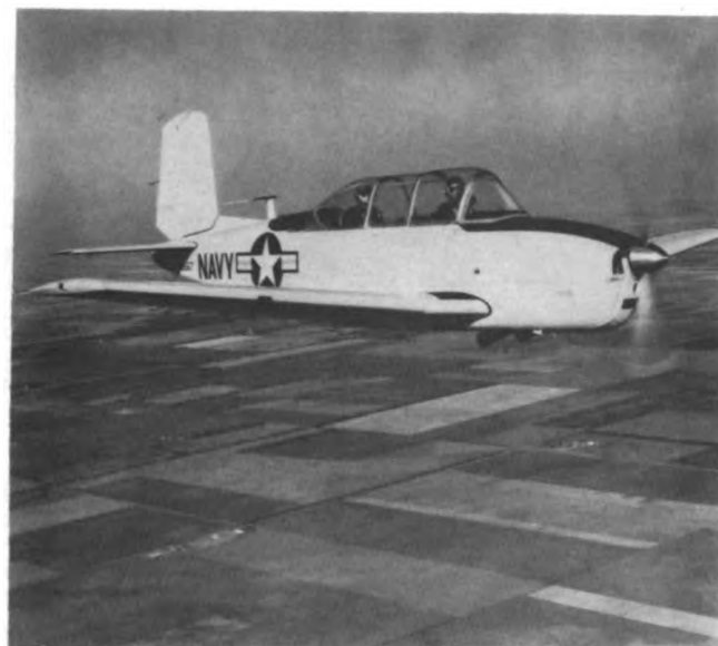
The T-34 is a two-place, single-engine, propeller-driven trainer with retractable tricycle landing gear. It replaced the SNJ.
