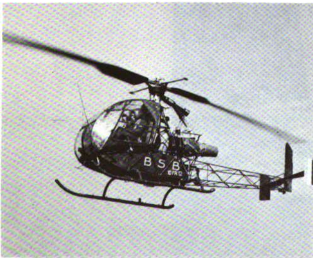
The S.O. 1221 DJINN is a two-seat, turbine-powered helicopter.
