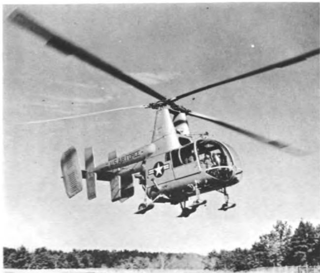
The H-43A carries a pilot, rescue crew of three, and fire-fighting equipment.
