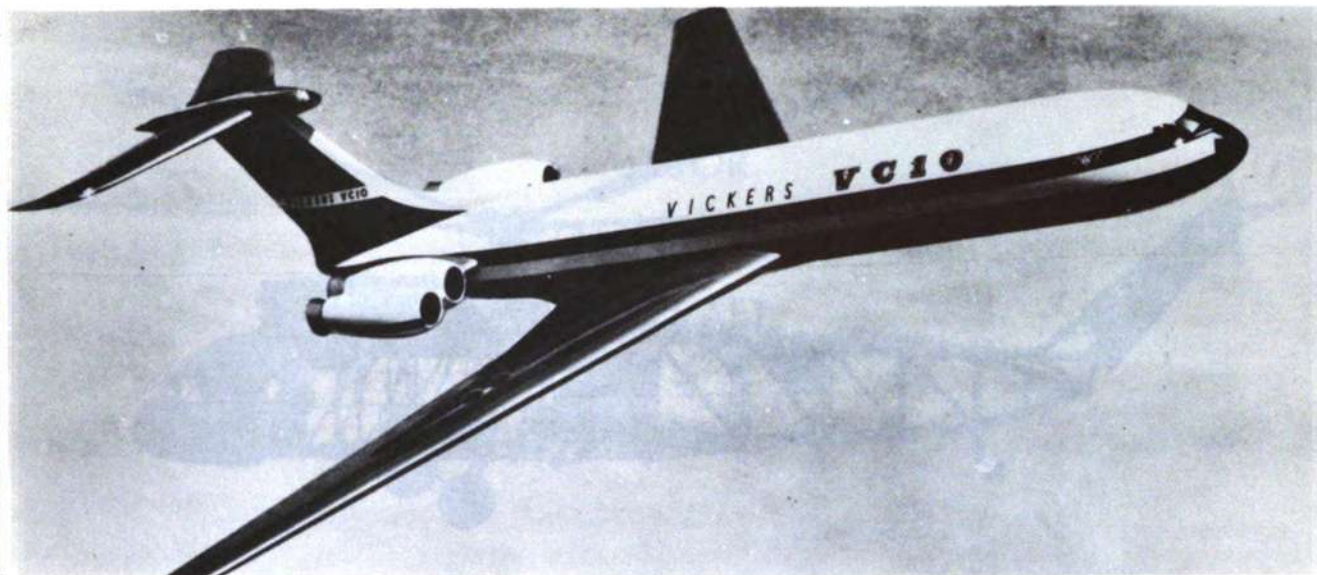
The VC. 10 airliner is the first aircraft to have four jet engines mounted at the fuselage rear.
