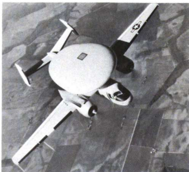
The WF2 TRACER is a modification of the S2F tracker, with the main difference being the huge radome for housing detection equipment, and the dual-fin tail.
