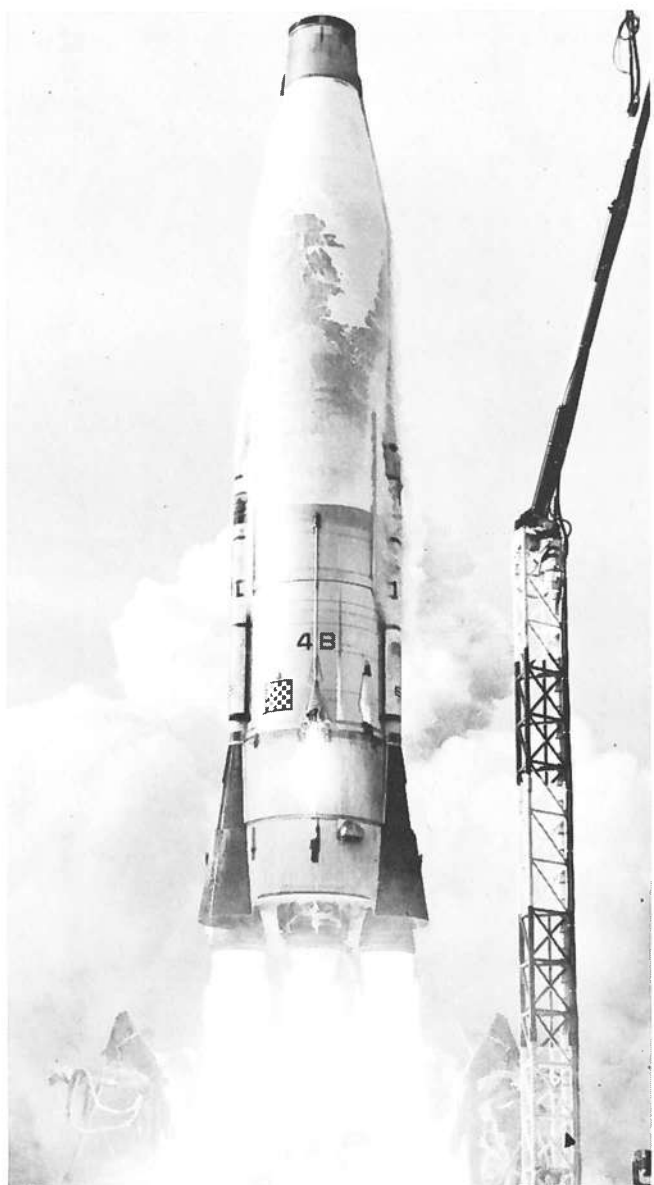
Atlas 4-B, actually the second flight of a 'B' vehicle, was launched on 2 August 1958, and flew 4,000 km down range. Note the corrugated transition section at the top, developed to support the General Electric Mk. 2 warhead.
