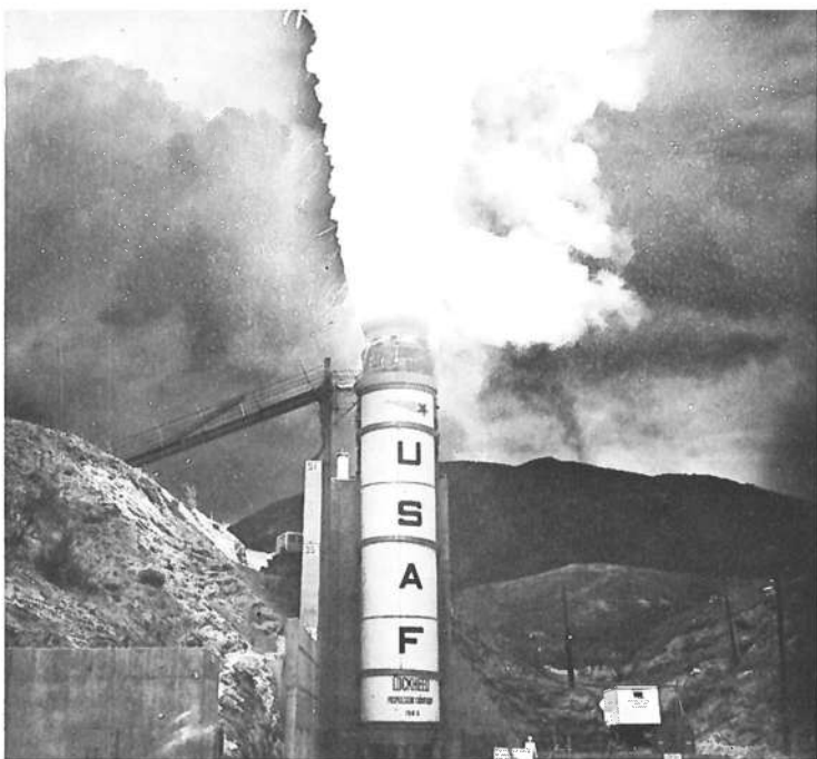
While large liquid propellant launch vehicles in the Saturn class were being developed, Lockheed Propulsion test a 3.96 metre diameter solid propellant rocket motor consuming 317 tonnes of propellant in 55 secs and producing 1,360 tonnes of thrust.
