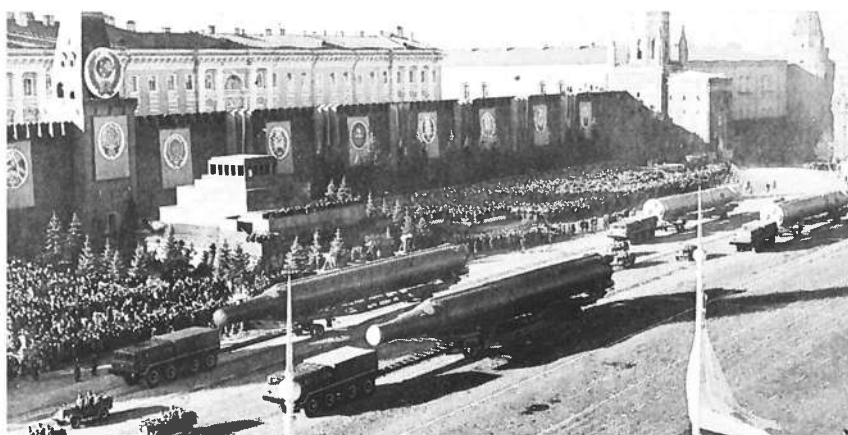
The SS-10 Scrag, obsolete because of non-storable propellants, was the longest ICBM ever developed. Note the truss structures separating the three stages and the four large motor nozzles in the first stage; upper stages had a single motor each.
