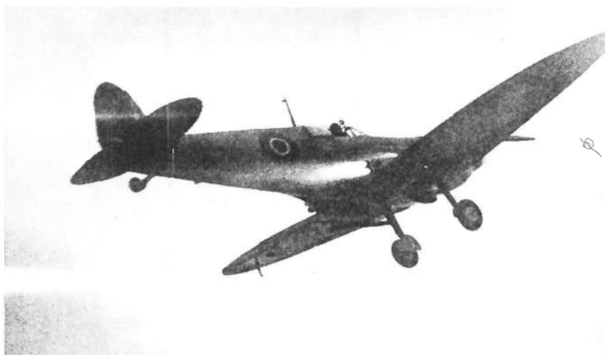
Launched from an aircraft carrier, the Supermarine Seafire receives a takeoff boost from two solid propellant rockets mounted each side of the fuselage on the upper surface of the wing.
