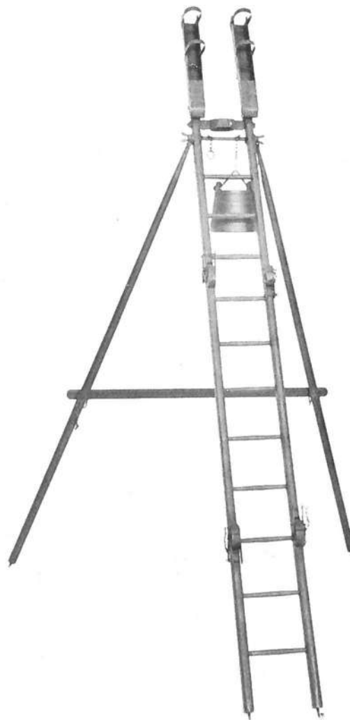
A typical launcher for ground-based Congreve rockets. Note the loops through which the cylindrical case of the projectile will be passed before launch.
