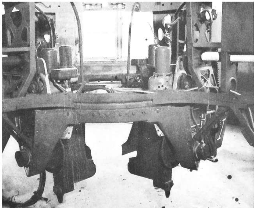
A-4 guidance was controlled in flight by four carbon rudders connected to servo-motors which in turn responded to signals from the guidance platform.
