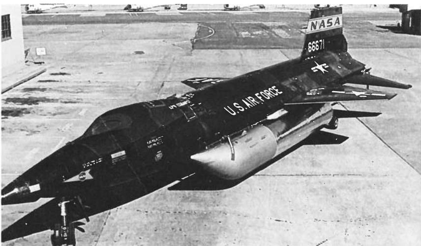
Work by Reaction Motors Inc., on the MX-774 propulsion system led from work on the rocket engine used for the Bell X-1 research aircraft. The definitive US rocket powered aircraft – the X-15 – is seen here sporting cylindrical propellant tanks used for boosting performance.
