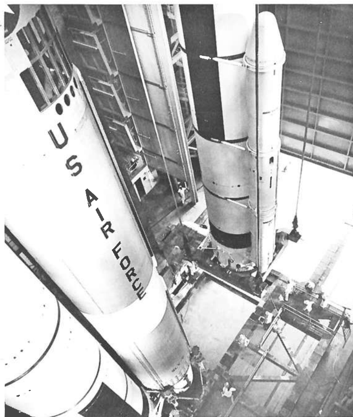
Engineers give scale to the massive strap-on boosters of a Titan III. Note the cone-topped nitrogen tetroxide container attached to the booster at right which would be used as a fluid injection control system.
