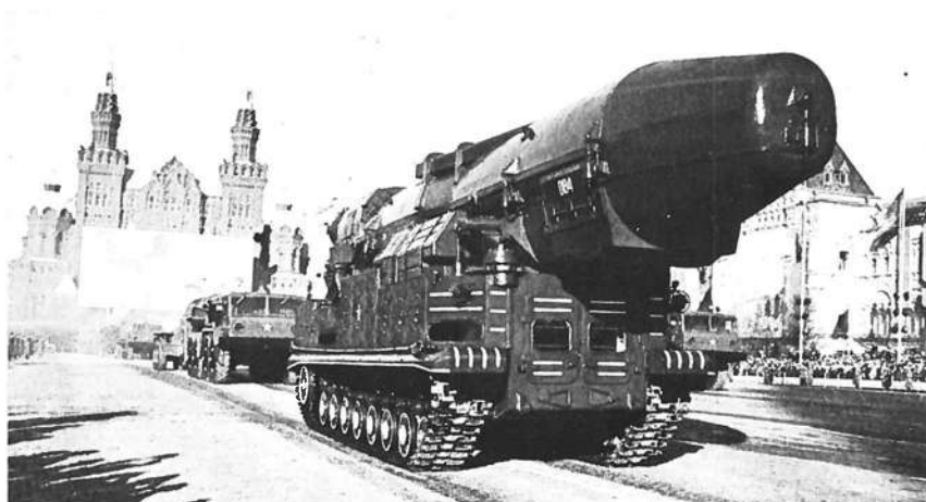
Concealed by its container in this view, the SS-15 Scrooge has a range of 5,500 km. Mobility is a key feature of medium range missiles like this and the SS-14.
