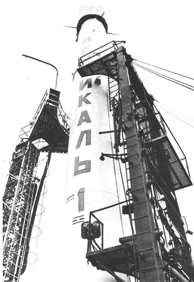
Service masts and access platforms surround this Soviet rocket launched for scientific research.
