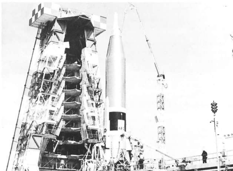
This series 'D' Atlas was sent on a successful flight from Cape Canaveral on 3 August 1960, with a simulated Mk. 3 nose cone. Note the large service tower at left, removed before launch.
