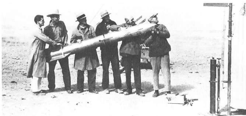
Goddard (second from right) and assistants prepare for a flight test which came on 27 October 1931, from Roswell, New Mexico. The new streamlined shape is in marked contrast to the earlier test vehicles and fins were added for stability. It flew to a height of 405 metres and a range of 283 metres.
