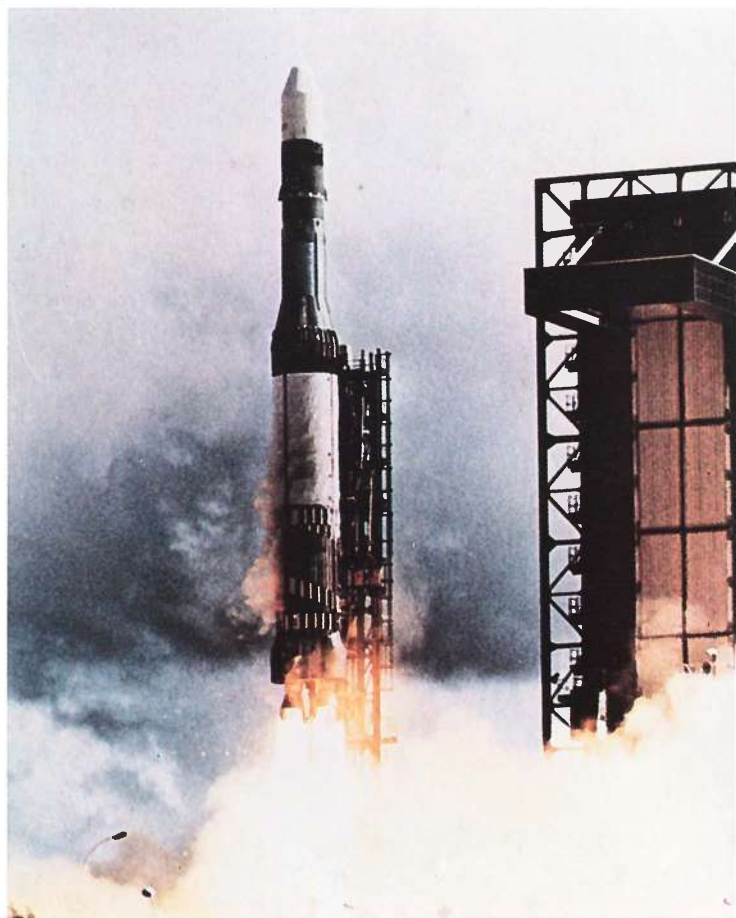
The Europa II launch vehicle, seen here ascending on a test flight, was developed from the British Blue Streak long range ballistic missile.
