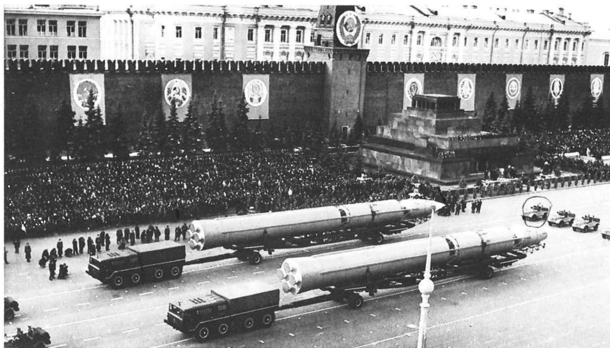
The SS-10 Scrag, obsolete because of non-storable propellants, was the longest ICBM ever developed. Note the truss structures separating the three stages and the four large motor nozzles in the first stage; upper stages had a single motor each.
