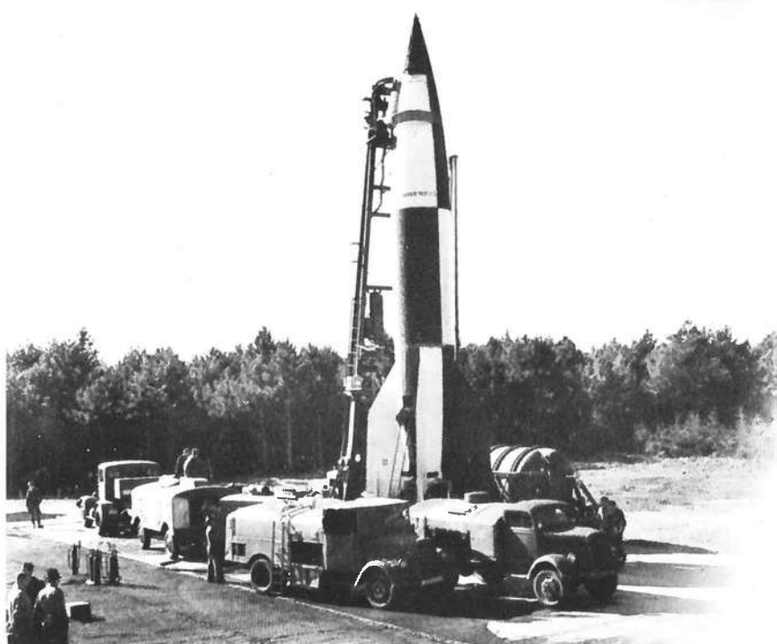
The Firing Control Vehicle from which final countdown and launch preparations were conducted before ignition of the V-2 propulsion system.
