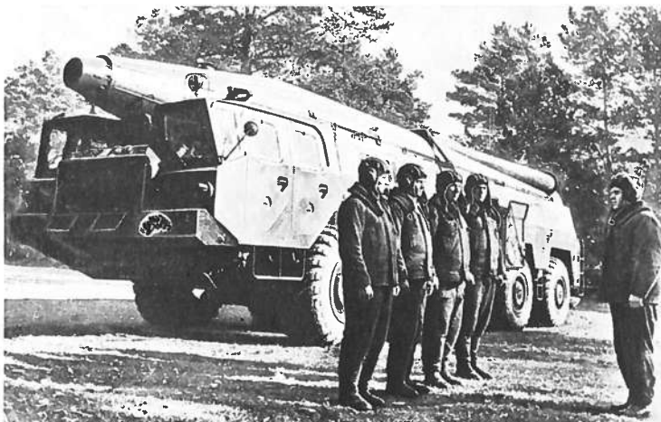
The solid propellant SS-12 Scaleboard had a range of 700 km and is seen here carried by a MAZ-543 transporter-erector.
