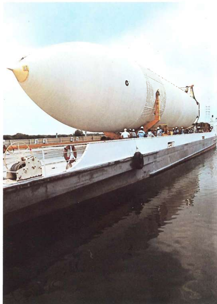
The massive External Tank that will be used to provide propellant for the Shuttle's three main engines is moved slowly by barge to the test site.
