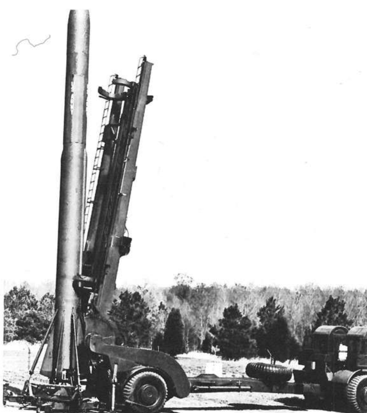
Developed at the Jet Propulsion Laboratory, the Corporal tactical battlefield missile would see extensive service with the US Army. The transporter/erector has just raised the missile 90° from the mobile position.
