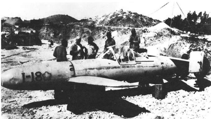
Japan's Ohka dive-bomber used a liquid propellant rocket motor to accelerate the device in the last 30 sec before impact. American personnel are seen here examining a captured example.
