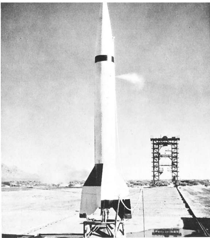
The earliest post-World War II effort in long range liquid propellant missile design was the brainchild of Karel J. Bossart, working at the then Consolidated Vultee Aircraft Corporation. Project MX-774 bore superficial resemblance to the V-2 (note the fin shape and the launch pedestal) but pioneered several revolutionary concepts.
