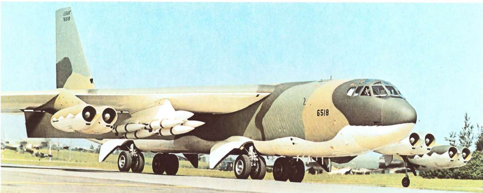
B-52 bombers of the US Air Force Strategic Air Command can carry 20 Short Range Attack Missiles, 8 internally and 12 under the wings. SRAM is an impressive extension of the bomber, itself only one element of the triad comprising manned aircraft, land-based missiles and submarine launched missiles.
