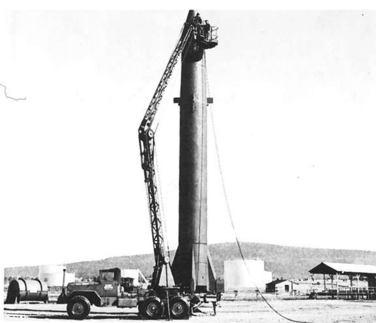
Technicians prepare a Redstone medium-range ballistic missile. Note the four short fins forward and the four aerodynamic fins and rudders at the rear.
