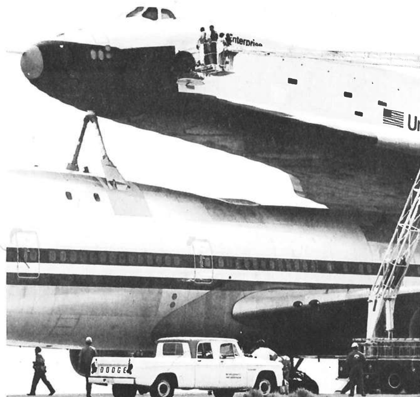
When Shuttle Orbiters are moved from one location to another they will be carried on the upper fuselage of a converted Boeing 747, as in this view taken during the drop-tests in 1977.
