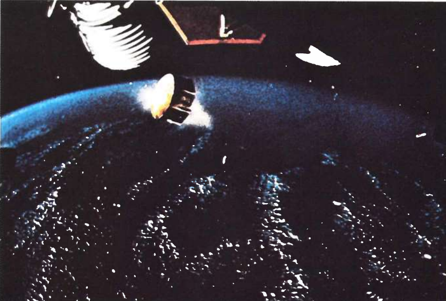
First stage separation of a Saturn V as viewed from a 16 mm film camera placed in the engine bay of the second stage, looking aft. The top of the frame in all four views is filled by two of the five J-2 second stage engines. At top, the first stage can be seen falling away; at mid-upper, the separation structure linking first and second stages is jettisoned; at mid-lower, the separation structure is seen tumbling; at bottom, it continues to fall beneath the ascending second stage.
