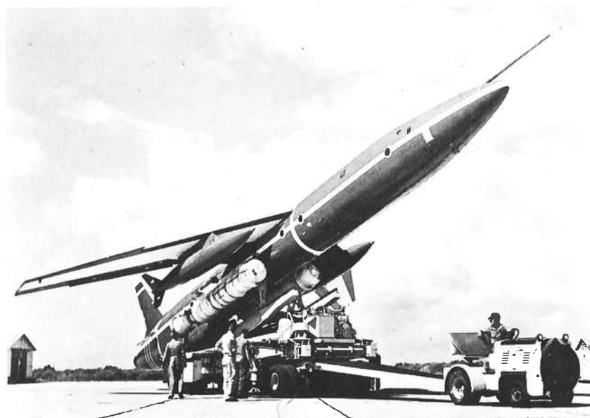
The turbojet powered Snark was propelled into the air by two solid propellant rocket motors, seen as white cylinders under the body of the missile, and could reach targets 11,000 km away with a 2.3 tonne warhead. Snark is here being towed from a test area to the main hangar at Cape Canaveral, Florida.
