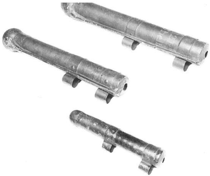
Examples of different Congreve solid propellant projectiles. Note the looped bands for emplacing the wooden guide stick and the single orifice through which the exhausted gases would escape.
