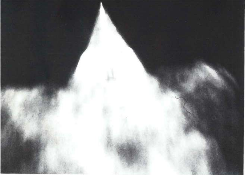
The instant of first-stage separation. Solid propellant rockets fire to retard the forward momentum of the stage and thus prevent re-contact with the upper stages of the Saturn V, momentarily enveloping the launch vehicle in a brilliant fire-ball.
