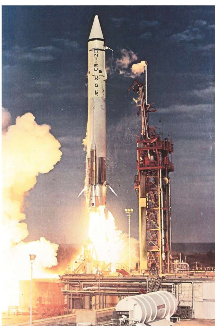
27 March 1969. An Atlas Centaur launches Mariner VII toward Mars from Launch Complex 36 at the Kennedy Space Centre. Note the large, cylindrical liquid nitrogen pressure vessel in the foreground and the two small vernier motors firing to left and right of the base of the Atlas.
