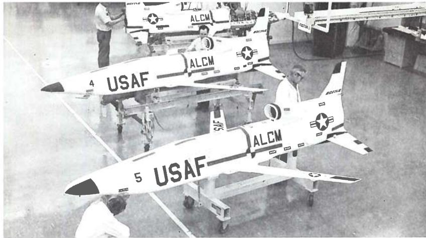
The Boeing Air Launched Cruise Missile is one of the most potent, yet compact, defence systems to be developed. Powered by a turbofan engine it could provide a similar deterrent threat to that posed by the MX system. Wings are folded until the missile is launched.
