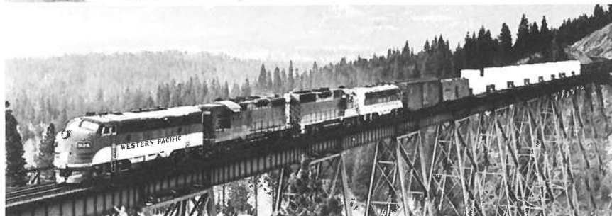
More than three decades span these contrasting modes of transport. The inset shows Robert Goddard transporting his experimental rockets by road in the early 1930's while, in the mid-1960's, a Western Pacific locomotive hauls separate segments of the solid propellant boosters used with Titan III.
