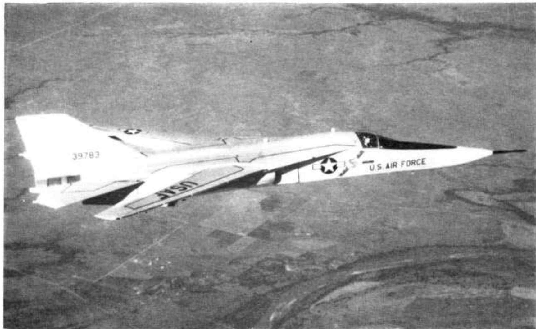
Head-on shot gives idea of F-111A's size. The tail stands 17 feet above ground. The aircraft is 73 feet, 6 inches long. Wingspan can vary from 31 feet, 11 inches to 63 feet.
