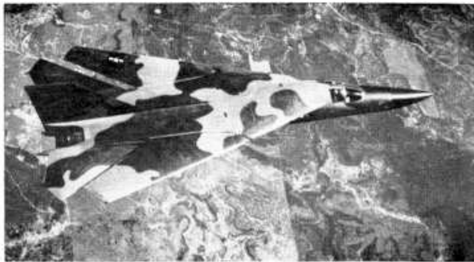
As speed increases and lift turns to drag, span and surface areas are reduced by sweeping the wings 72.5 degrees until tips rest close to the tail for supersonic dash capability.
