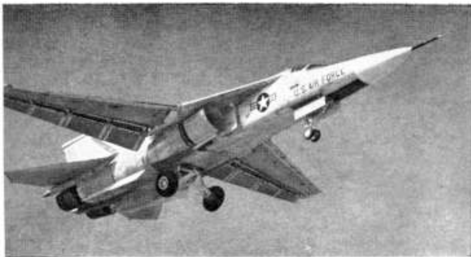
F-111A on early cross-country flight from Fort Worth, Tex., to Edwards AFB, Calif. With wings straight out, pilot gets maximum lift for takeoff and landing on short runways.
