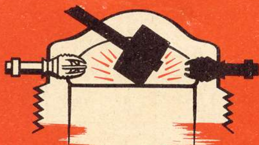
Sudden combustion causes detonation
