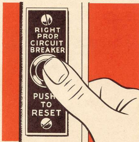
In emergency, hold circuit breaker in
