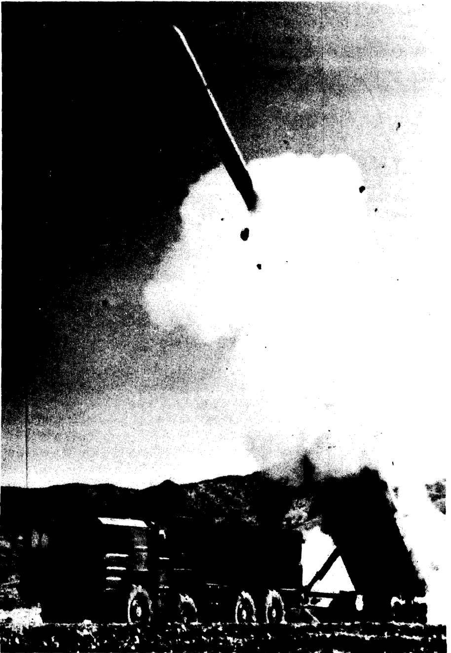
General Dynamics GLCM fired from its TEL (Transporter-Erector-Launcher). (General Dynamics)
